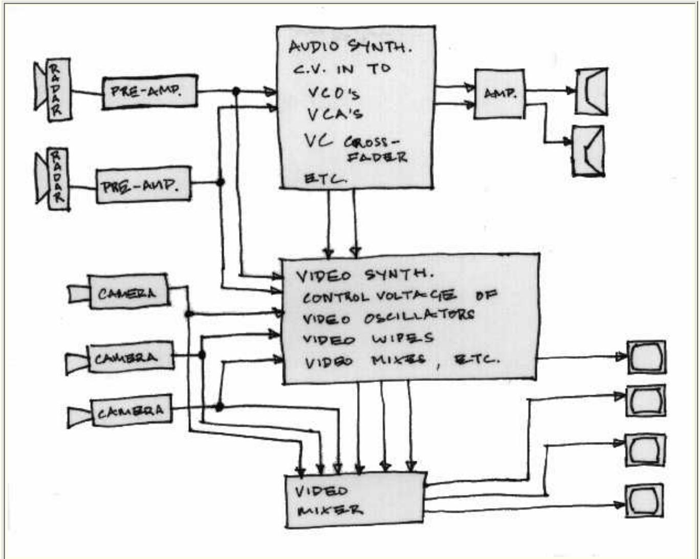
**A live performance installation system using doppler shift detector radars for detecting the performers movement throught the performance area - the data from the radars is fed to the synthesisers to control the camera / video synthesiser mix and the sounds generated by the audio synthesiser . The performer can then modulate her actions according to the feedback from monitors and speakers so as to create the effects desired.**
