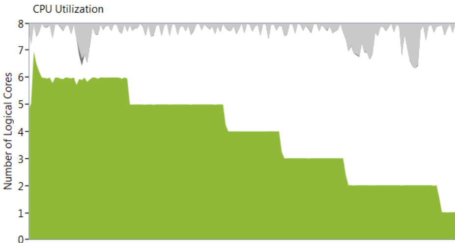
Figure 6-2. Overall CPU utilization rose to almost 8 logical cores (100%) and then dropped to only one logical core at the end of the run
