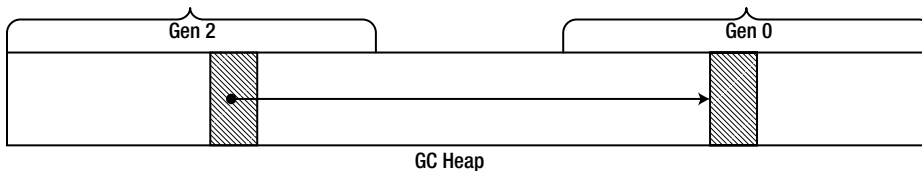
Figure 4-14. References between generations might be missed if during the mark phase we stop following references once we reach an object in a higher generation
