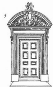
② Columns were a desirable but expensive frame to a door; plasters were a less expensive alternative. Ham House, Surrey, 1640.
