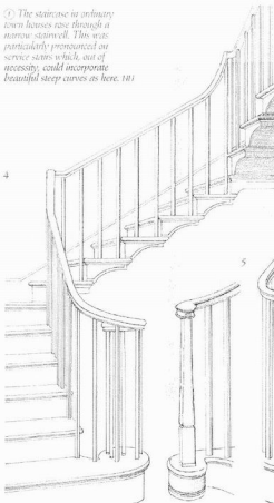
② In grand houses, the handrail on main stairs was finely moulded and terminated in a spiral, be it a tight coil or, as here, a loose curve. 181
