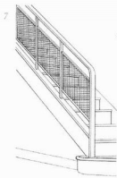
⑧ Flowing lines are characteristic of the Modernist period. Here regular loops of steel are arranged up the staircase: the treads and a chromium rail on the upper floor provide the points of contact. A brass handrail accentuates the staircase's form, 1938.
