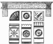
⑧ Millwork catalogues include doorcase ornamentation. Shown here are a hardwood "cap trim", as well as corner and head blocks made of composition. RO
