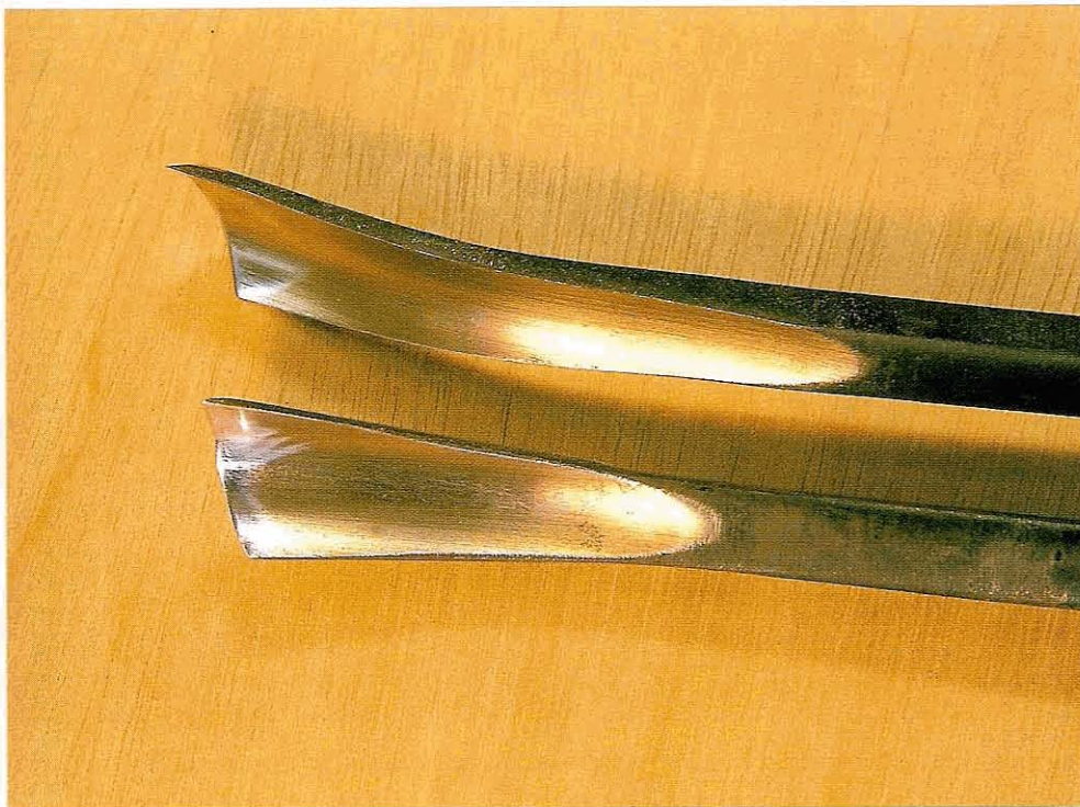
Fig 6.6 The working ends of these Cogelow gouges are skewed and slightly bent
