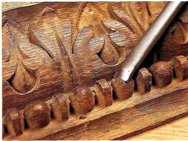
Fig 5.15 The beads in this old carved moulding were cut with a gouge in the reversed position
