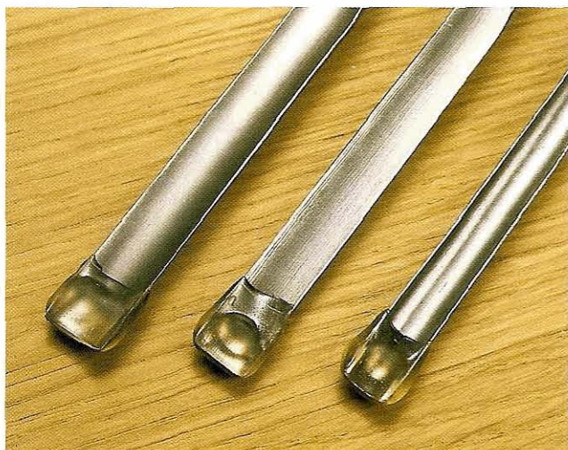
Fig 8.4 Brightly polished, pre-sharpened tools, their tips protected by dipping in a rubbery gel
