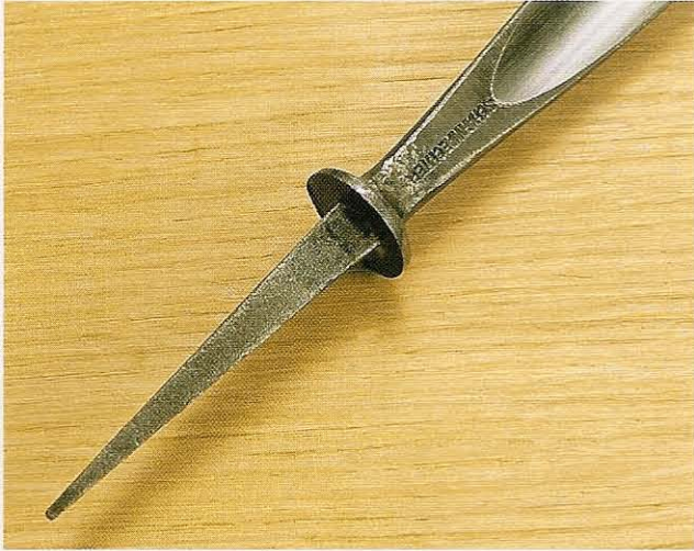
Fig 2.72 A strong, straight, well-made and purposeful tang
