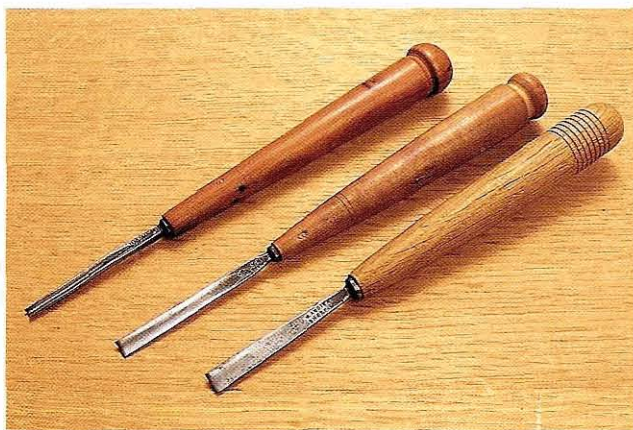
Fig 5.24 Short tools can be brought back into circulation with handles of extra length
