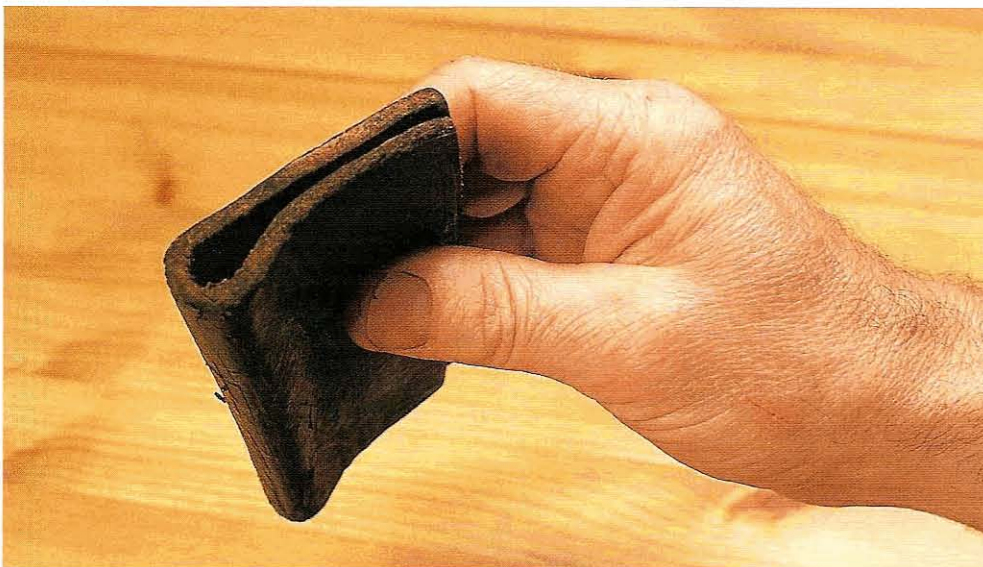
Fig 11.31 For larger tools a piece of folded and dressed leather is the simplest slipstrop. Be sure to make it of an adequate size to keep the leather flexible where the abrasive covers it, and to keep your fingers clear of the blade
