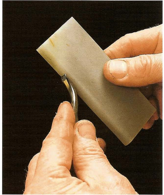
Fig 12.56 Slipstones are used with the benchstone to sharpen a backbent gouge
