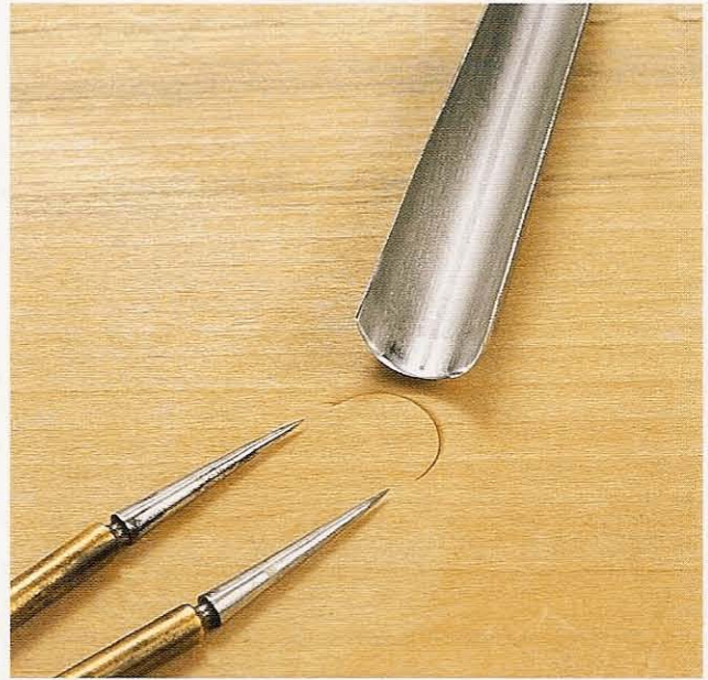
Fig 2.60 With the exception of skew chisels, it is the actual cutting edge which is measured, from corner to corner
