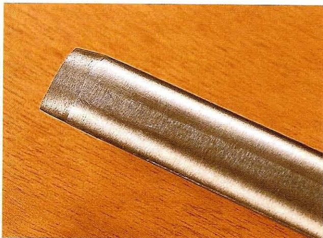
Fig 9.47 Coarse scratches on a bevel which has been ground but not honed; you will need to orientate the blade to examine them clearly
