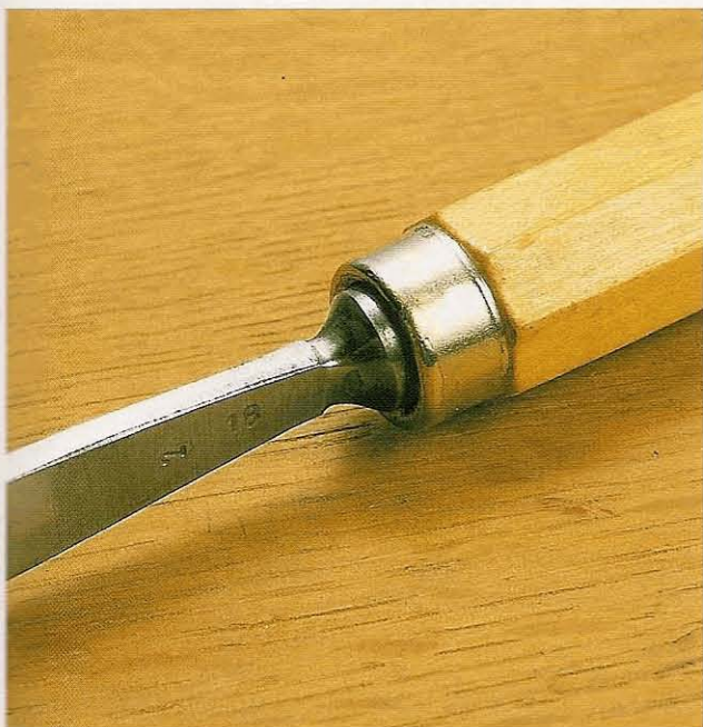
Fig 3.9 A thick layer of varnish over the whole handle has congealed into a glob on the ferrule. Removing it may make the handle much more comfortable
