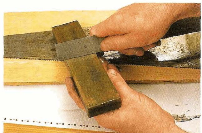
Fig 11.14 It does not take long before the surface of the stone is truly flat
