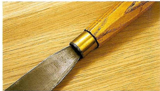
Fig 5.30 A gouge which had lost its tang through rust, now back in use
