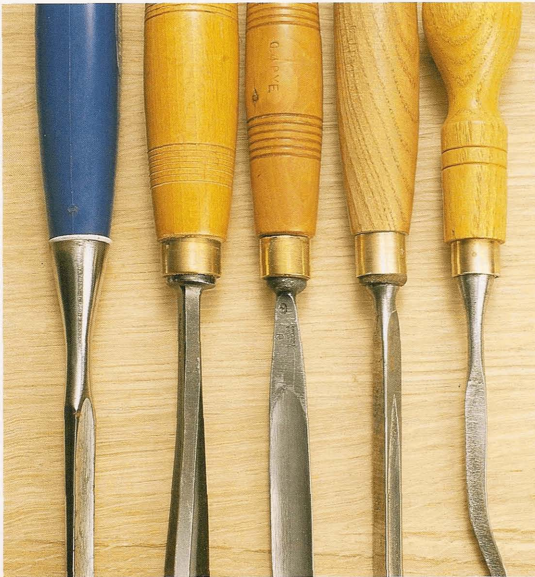
Fig 2.68 Different manufacturers shape the shoulders of their tools in different ways, some taking more care than others
