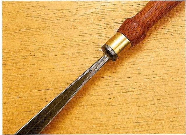
Fig 9.39 Uneven wall thickness in a V-tool may sooner or later cause difficulty in sharpening
