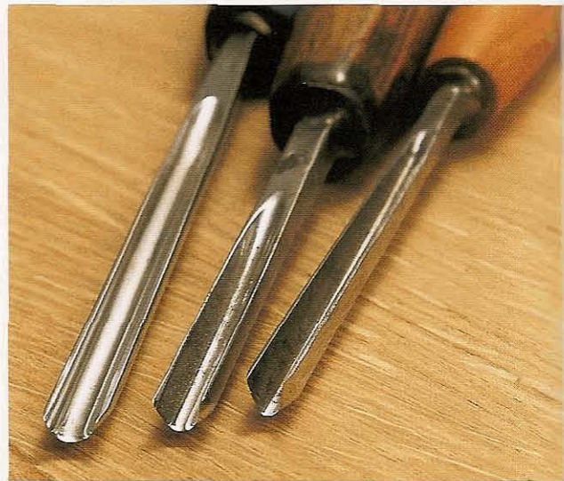
Fig 2.24 A selection of deep or 'quick' gouges, from a semicircle on the left to the deeper U-shaped tool on the right
