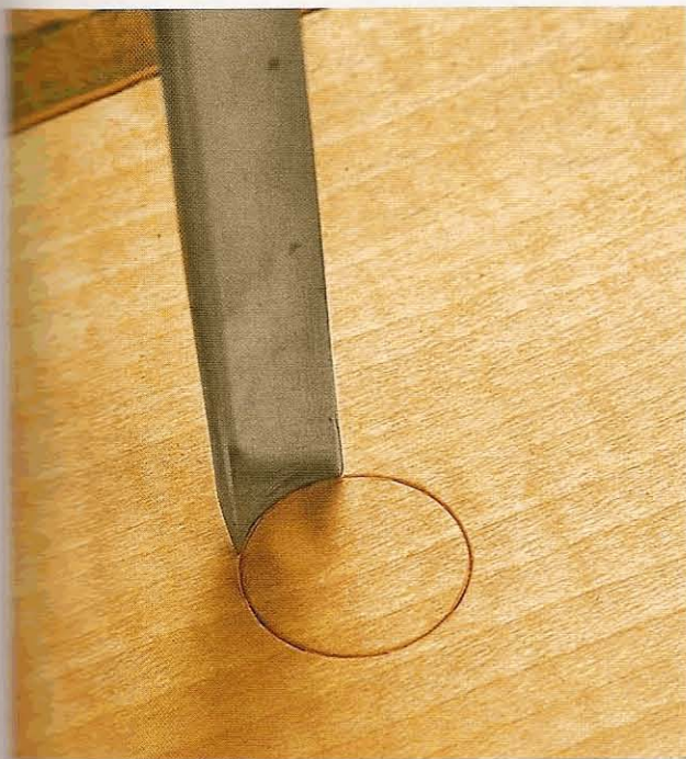
Fig 2.26 Any gouge with a circular sweep will cut a circle of a size corresponding to its own radius
