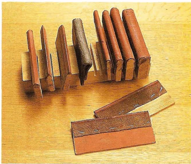
Fig 11.35 An assortment of slipstrops kept ready for use in a purpose-made rack
