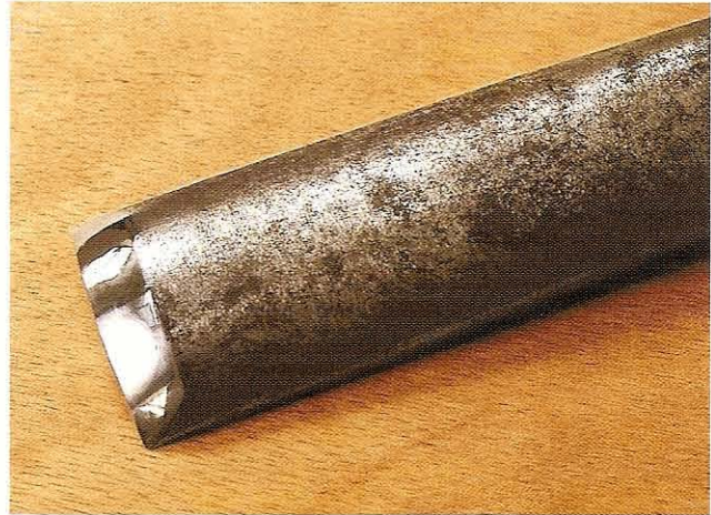
Fig 5.28 A badly rusted surface on a gouge blade, but not pitted enough to affect the cutting edge, which lies more towards the centre of the steel
