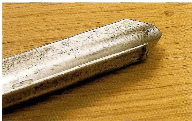
Fig 8.1 The nose of a woodturner's spindle gouge: both the steep bevel and the rounded end make this an unsuitable shape for a carving tool
