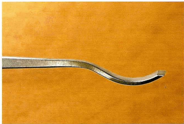
Fig 9.5 The bevel offered by the maker of this tool is about 45°. It may never occur to a newcomer to carving that this can be, and needs to be, changed
