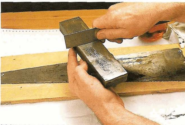
Fig 11.13 . . . and wipe with a metal straightedge. The new flat surface will be seen encroaching on the hollow, sludge-filled centre
