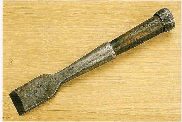
Fig 2.73 A socketed shipwright's chisel with an iron end ferrule; such a strong socket will take far more punishment than a tang
