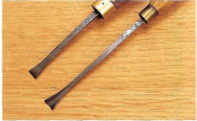
Fig 5.25 The older fishtail tool at the top started life about the size of the lower one
