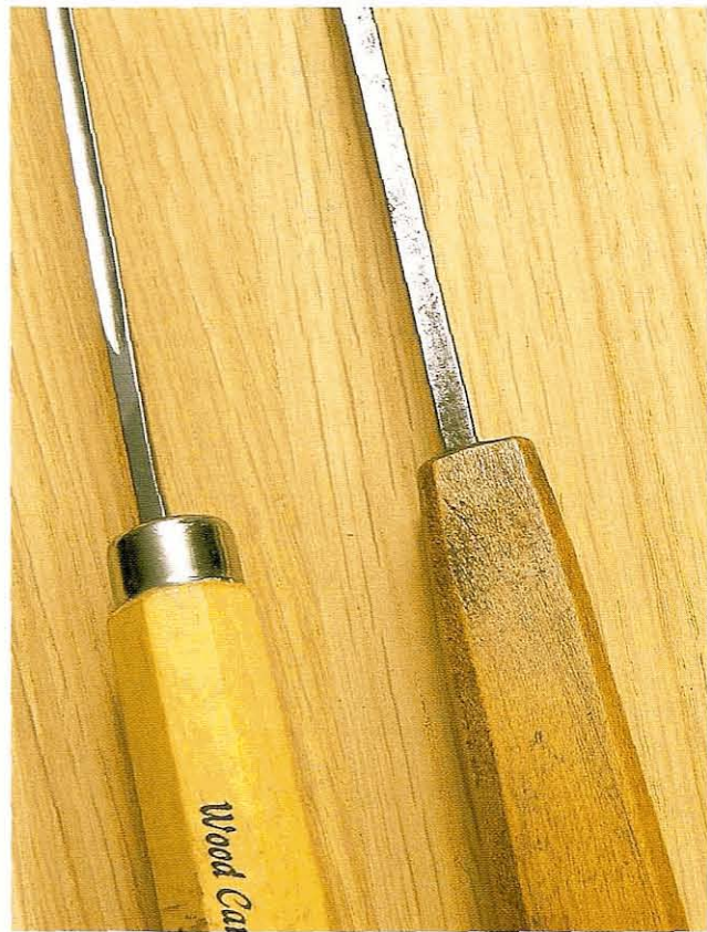
Fig 3.26 Accurate boring is needed if the blade is to be concentric with the handle
