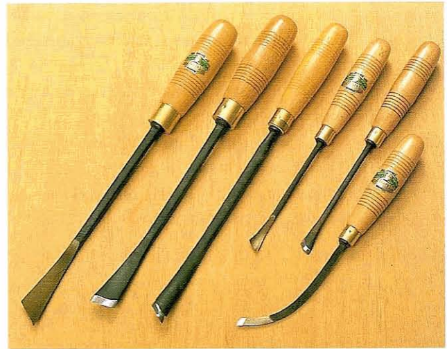
Fig 6.5 A selection of Cogelow tools; these come in a variety of lengths, shapes and bends, including the bent skew chisel shown on the right
