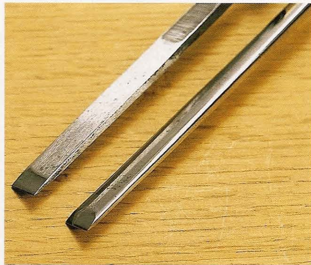
Fig 2.36 The straight chisel normally has flat faces. The oval shape of the lower tool is an attempted innovation, but I find its smooth corners make it less easy to grip
