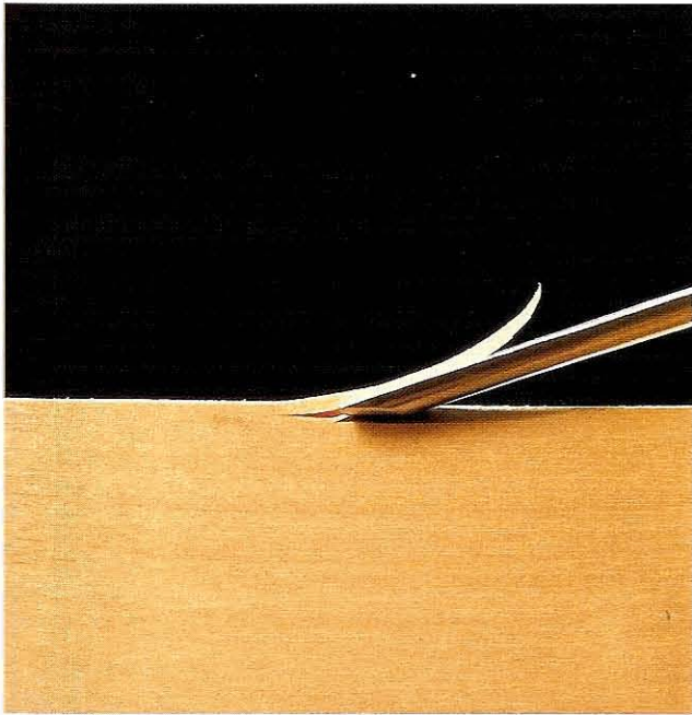
Fig 9.3 The wedge-like action of the bevel is evident here, causing the wood to split in advance of the cutting edge
