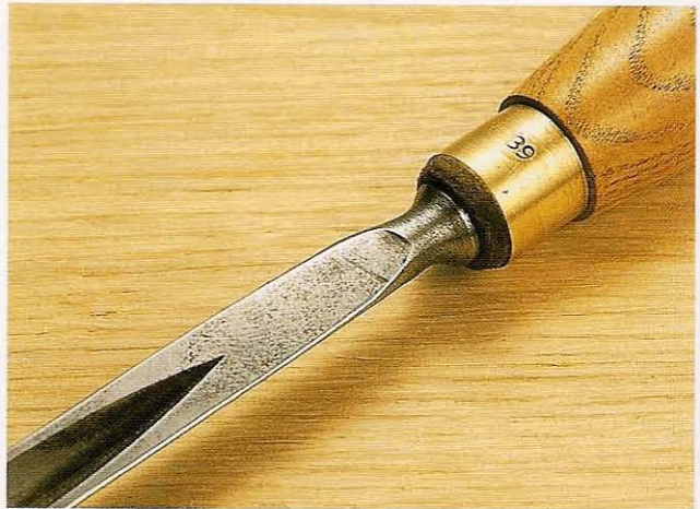
Fig 2.65 Leather washers like this are more for the sake of appearance than for function
