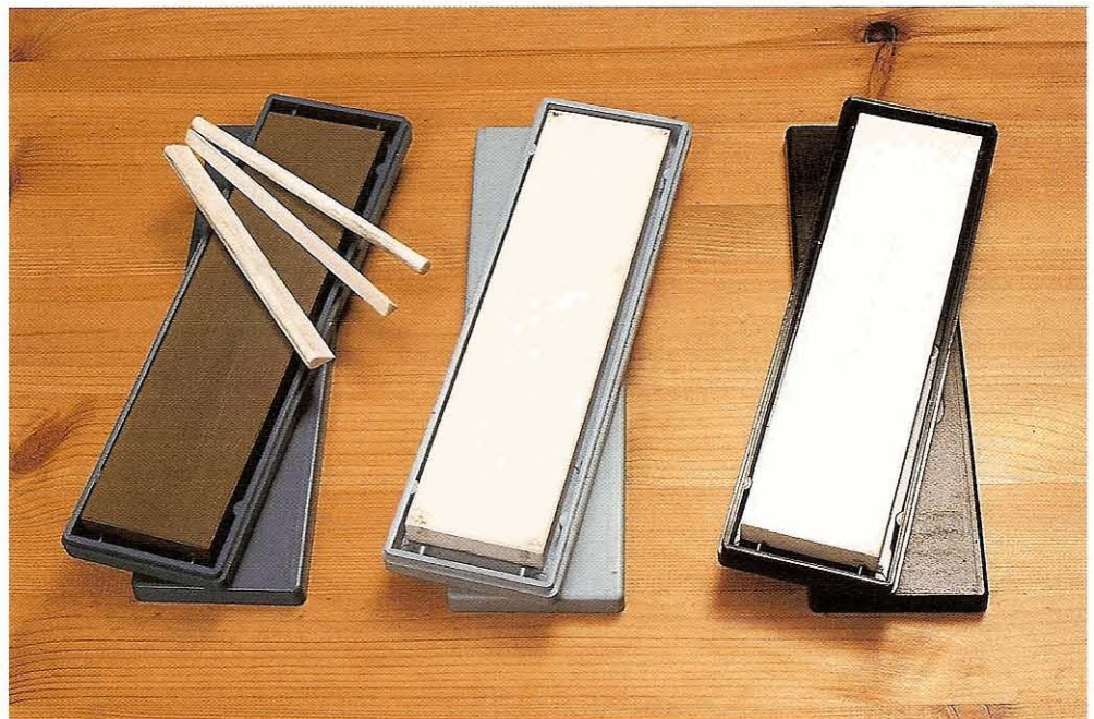
Fig 13.9 Ceramic benchstones and slipstones. The colour of the box indicates the grit
