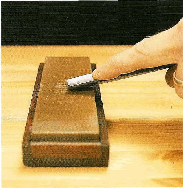
Fig 12.10 Working across the benchstone with a gouge; the stone is orientated on the bench square-on to the user
