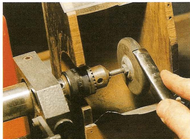
Fig 14.4 Shaping an inside bevel on a Cratex rubberized abrasive wheel. Note the dust-extraction hood
