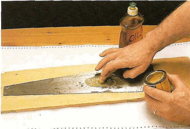
Fig 11.11 Mix some oil and grit on the flat surface . . .
