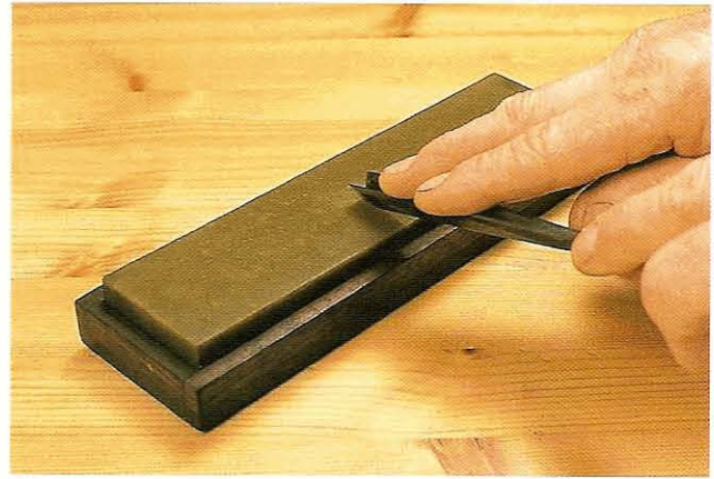
Fig 12.39 Rounding over the keel of the V-tool by careful rubbing on the benchstone. As always, present the bevel flat and keep checking the edge by its line of light
