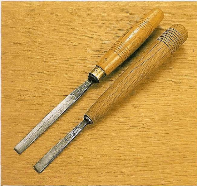
Fig 3.5 It is possible to lengthen a short tool to the normal overall length by means of a custom-made handle
