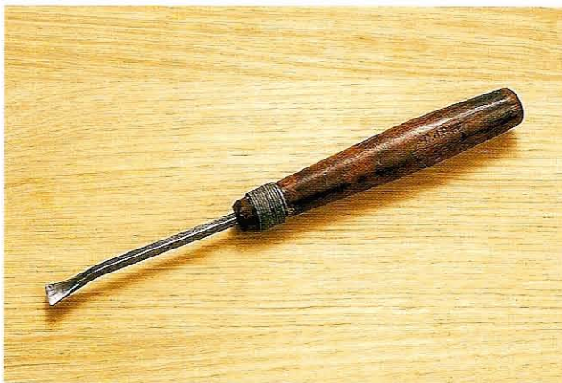
Fig 3.21 A favourite shoulderless tool benefits from a lovely bit of ferrule improvisation
