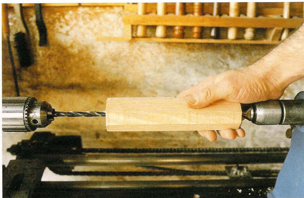
Fig 3.28 On the lathe, a hole can be drilled easily and accurately between centres
