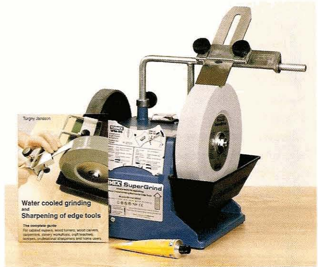
Fig 10.3 A wet grinder, showing the large, slow wheel in its trough on the right and a buffing wheel on the left
