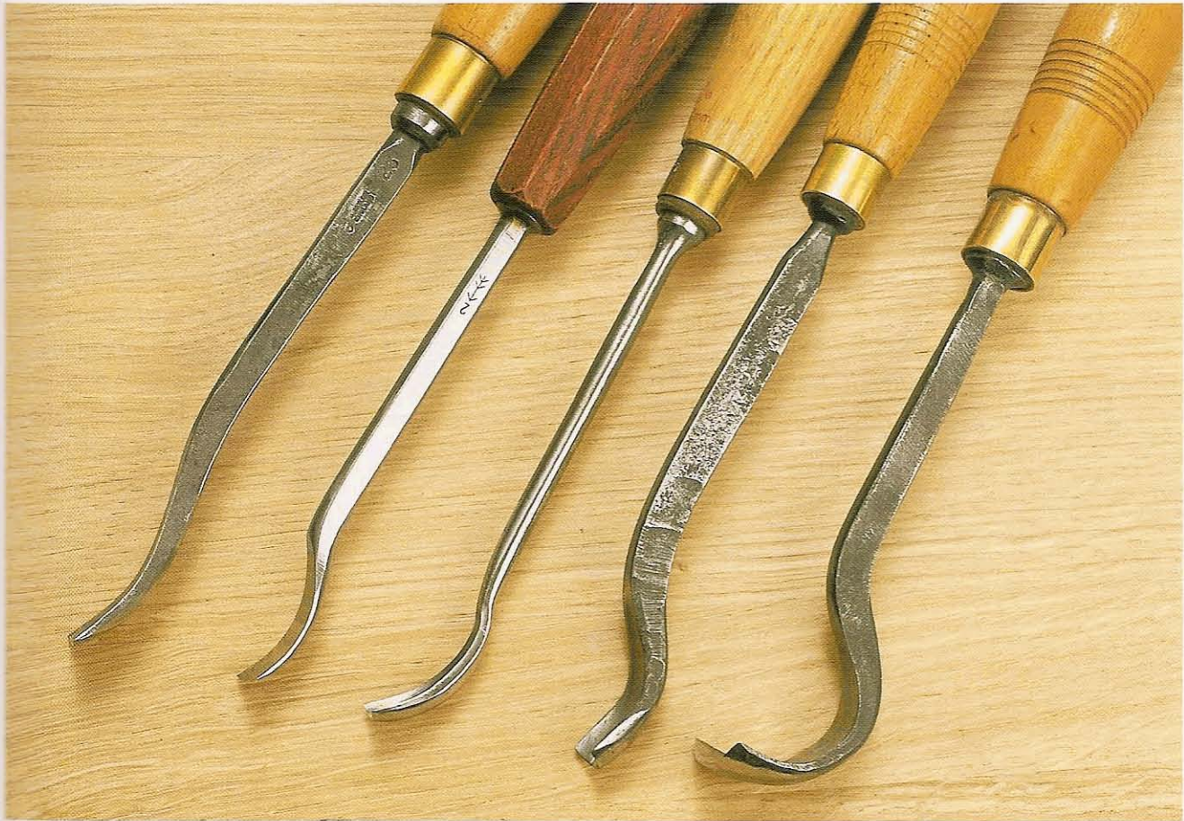
Fig 2.52 As with longbent tools, the lengthwise curvature of shortbent tools by different manufacturers varies considerably, and some versions are hardly bent at all. The right-hand one was made by the author as described in Volume 2, Chapter 3
