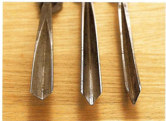
Fig 12.32 The three different V-tool angles will need corresponding angles on the slipstones
