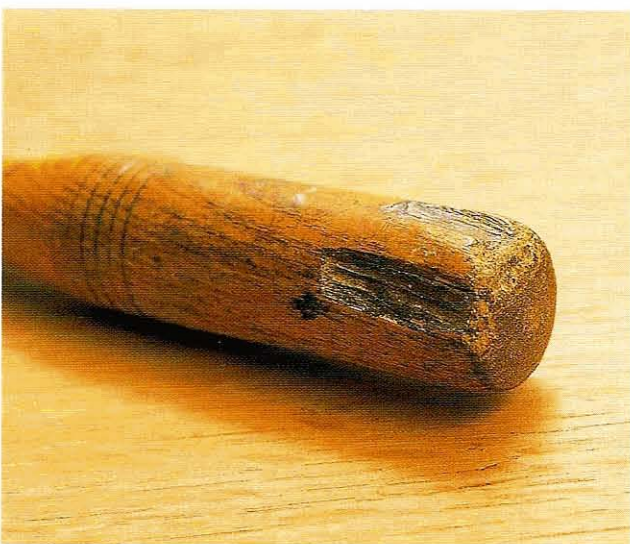
Fig 3.22 Repeated mallet blows may eventually split pieces off the end of the handle
