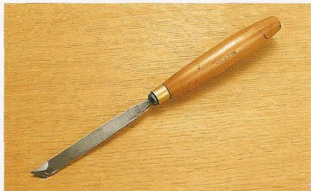
Fig 2.15 The basic skew chisel; the tip of this one has been ground as described on page 148 (see Fig 9.42)
