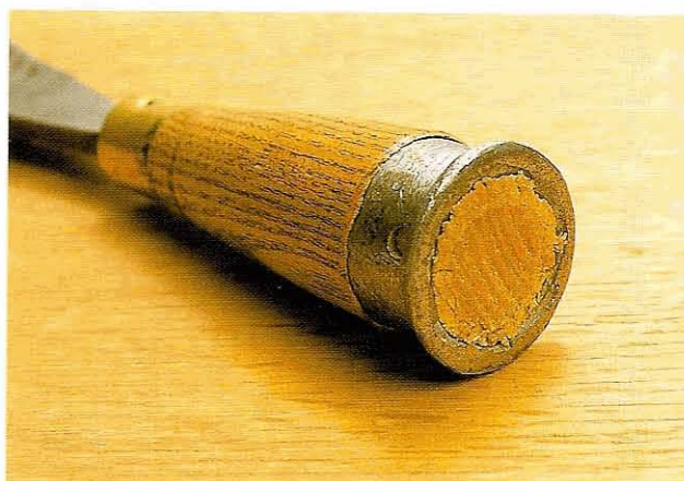
Fig 3.25 Even an iron ferrule can itself burr over after weeks of hard mallet work
