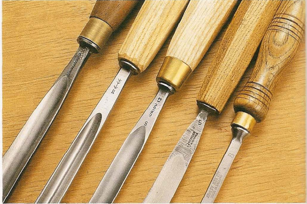
Fig 1.8 The shanks of a selection of modern tools, stamped with the names and logos of the makers, as well as a tool number
