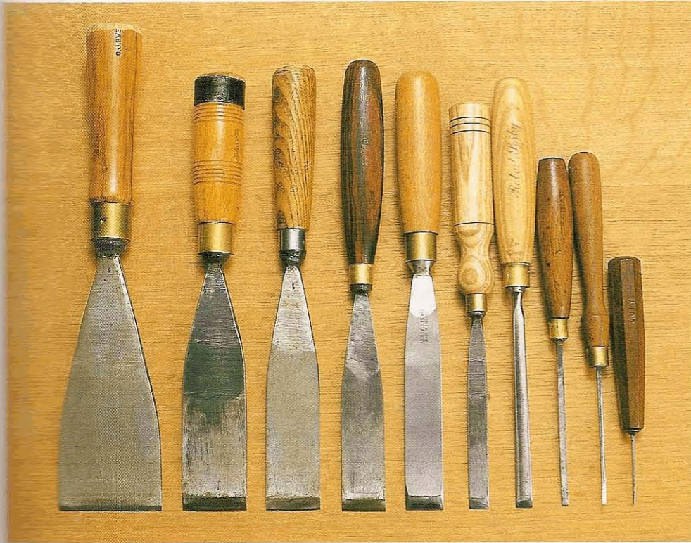
Fig 1.10 These tools all specify the same Sheffield List number (01) and differ only in the specification of the width
