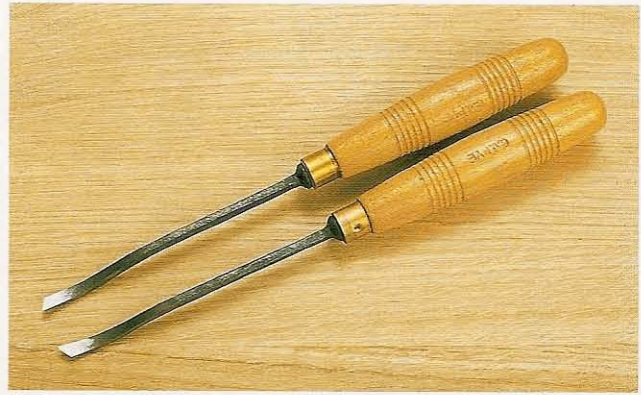
Fig 2.49 Shortbent skew chisels come in pairs, left- and right-handed, to suit different grain conditions
