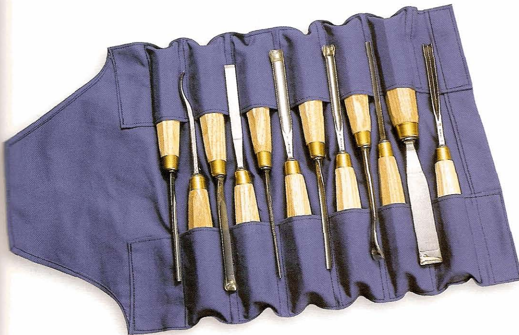
Fig 7.1 In a tool roll, the handles in one set of pockets support and protect the blades of the tools on the opposite side
