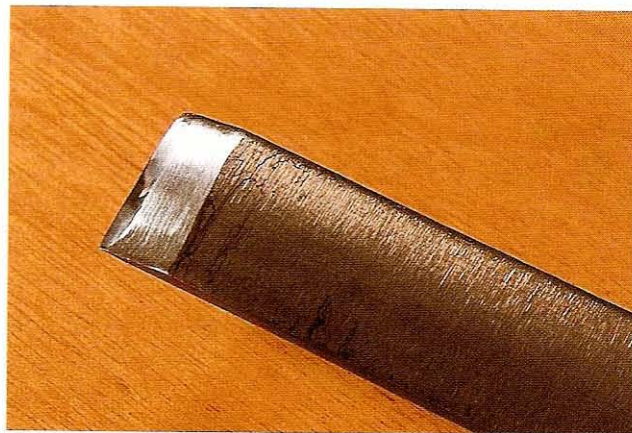
Fig 9.49 The scratches towards the heel, as well as the polished metal towards the edge, would suggest that the bevel is rounded and not flat
