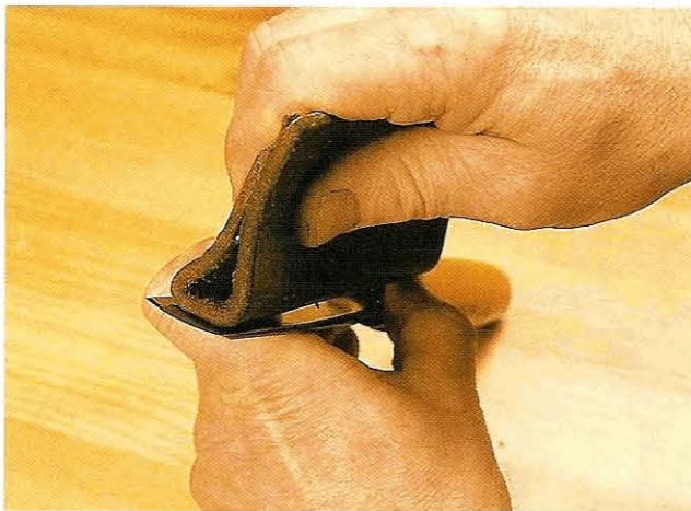
Fig 12.25 A leather slipstrop will deform to fit the sweep of the gouge as it is pushed forward
