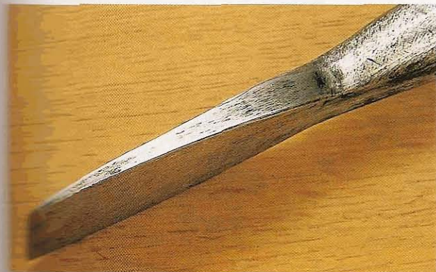
Fig 2.13 An old firmer chisel with a socketed rather than angled blade, tapering straight to the edge
