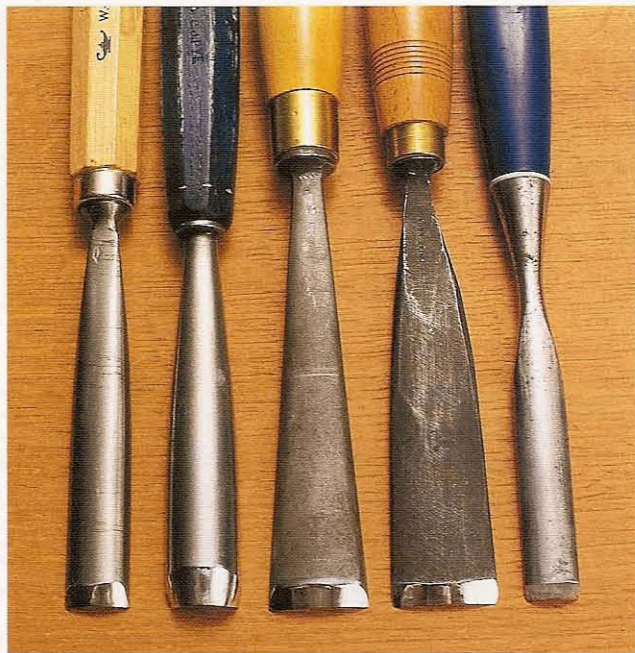
Fig 2.1 Five similar gouges from different manufacturers, each finishing the tool in a different way – how do you know what the steel is like underneath?
