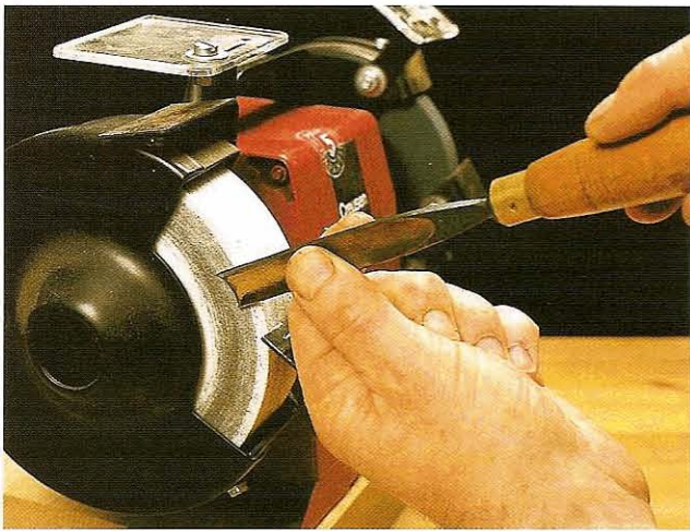
Fig 12.6 Touching the carving tool to the side of the grinding wheel; only the lightest touch is permissible
