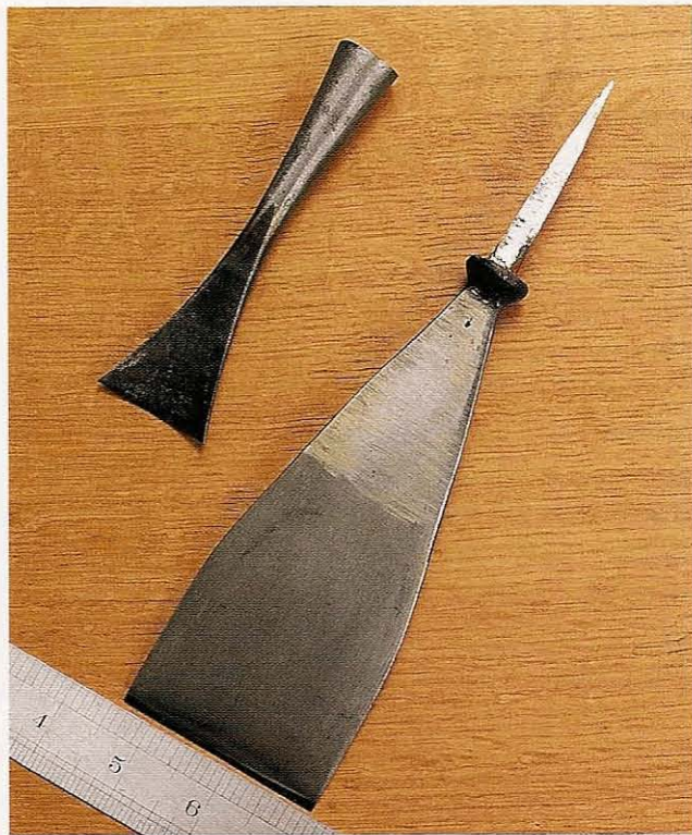
Fig 2.79 When we get to carving tools of this size – 2½in (65mm) – a tang only ¼in (6mm) wide is beginning to look a little inadequate, and a socket might be a better option
