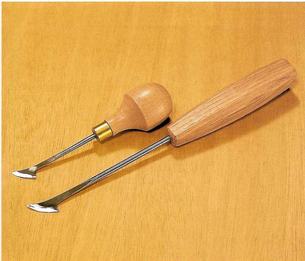
Fig 6.3 Gonzalez hooked skew chisels: palm type with mushroom handle, and regular-size tool
