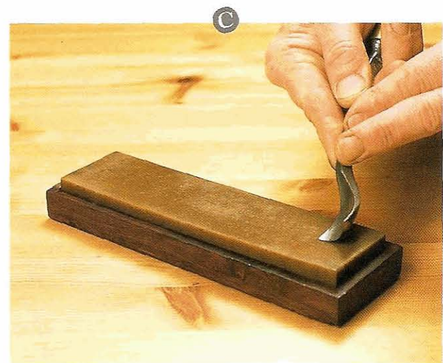
Fig 12.53 The pattern of sharpening the outside bevel of a frontbent gouge is the same as for a straight one, except that presenting the tool is a little more awkward. (For clarity the oil is not shown)
