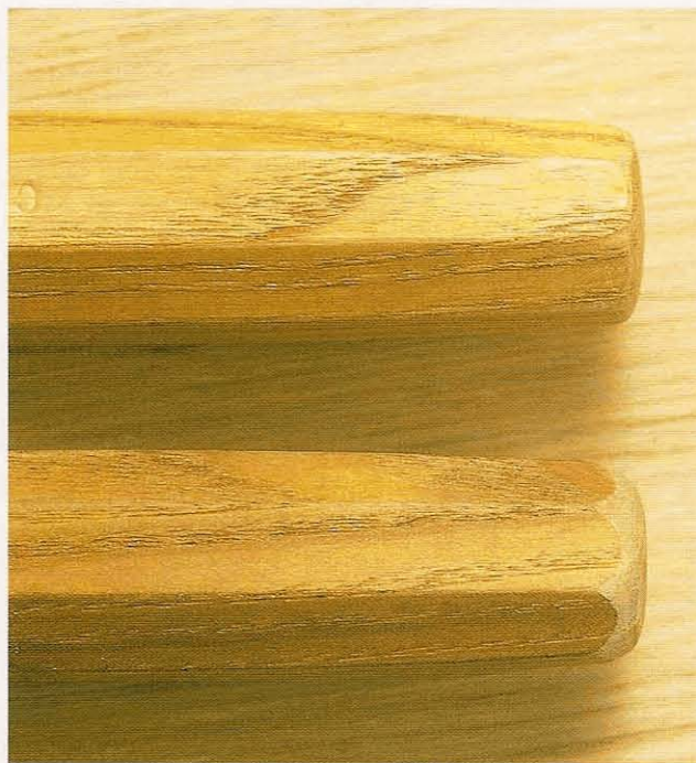
Fig 3.10 Octagonal handles can have quite sharp corners (top); round them over to make them more comfortable
