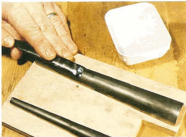
Fig 13.7 Start in the middle of the sweep, gauging where you are from the trail of black metal debris in the water on the cone surface
