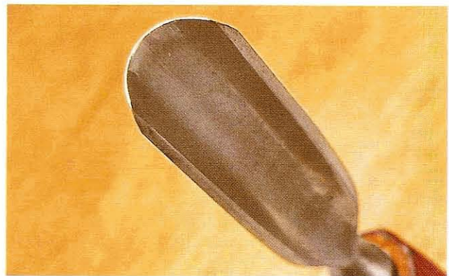
Fig 9.46 The white line of light is getting thinner and more uniform, but is still clearly visible all along the edge
