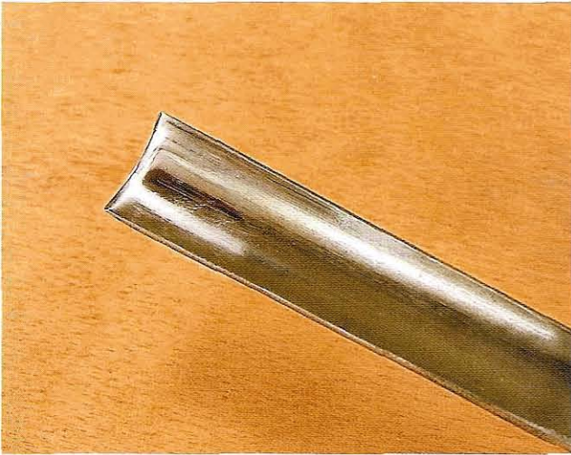
Fig 9.20 The well-stropped inner bevel, seen from above,
