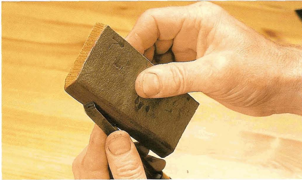
Fig 12.41 A specially made V-tool slipstrop. Keep your fingers clear
