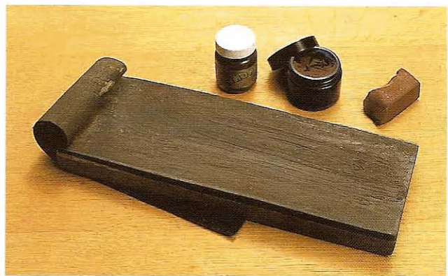
Fig 11.29 A benchstrop with its cover tucked back and ready for use. Also shown are some dressing compounds: a proprietary stropping paste (left), a home-made mixture of tallow and fine abrasive, and a block of crocus abrasive
