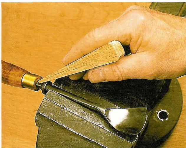
Fig 3.34 Using a wedge of hardwood to knock off the handle. Keep your hand clear of the cutting edge!
