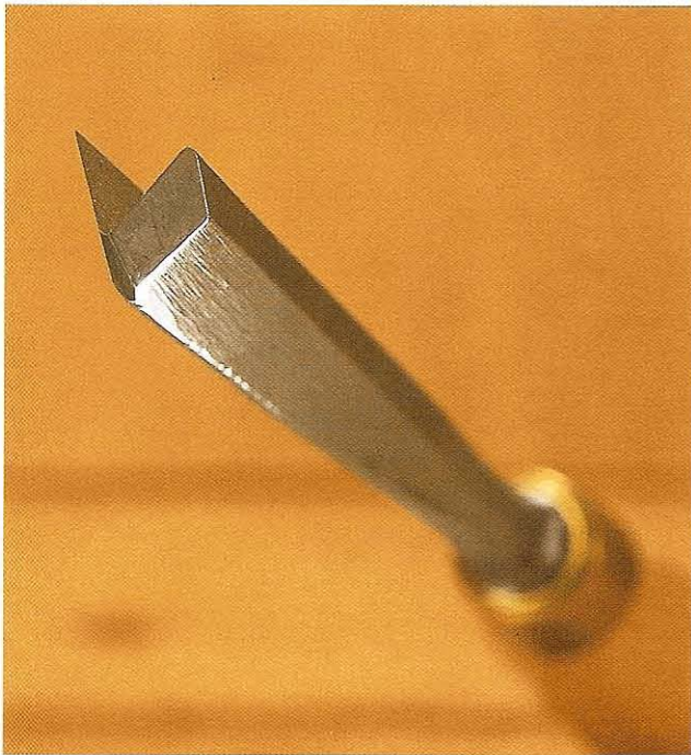
Fig 12.30 Close-up of the end of the V-tool; the apex of the V is not a sharp angle but slightly rounded
