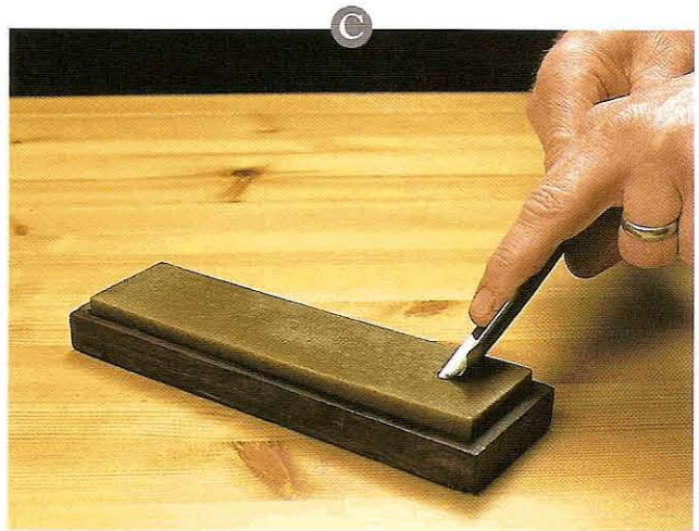
Fig 12.45 Rotating the gouge from one end of the benchstone to the other. The motion is then repeated in the opposite direction, without lifting the blade from the stone
