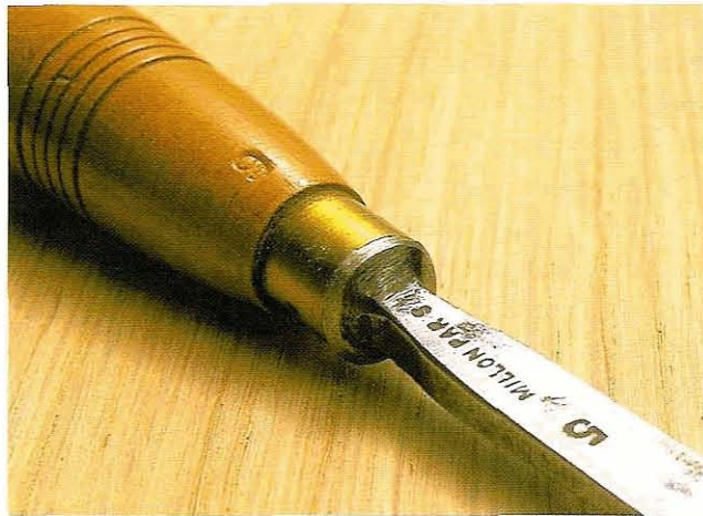
Fig 3.35 Problems in removing the handle may arise when the shoulder is very tight to the ferrule
