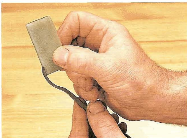
Fig 11.24 Small slipstones can be used very delicately for specific and exact sharpening
