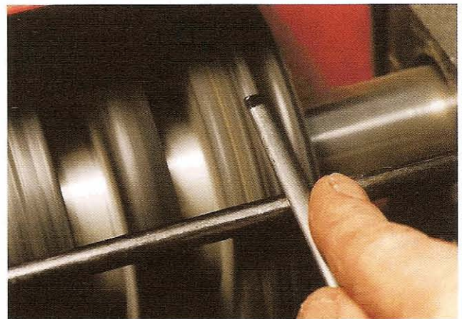
Fig 14.7 With a split wheel it is possible to hone the inside of a gouge without damaging the corners
