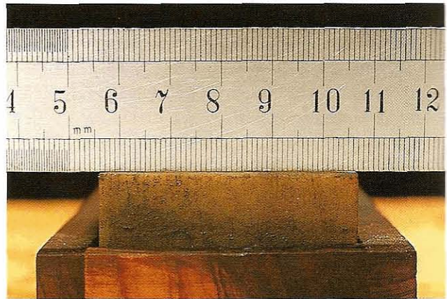
Fig 11.7 Typically, the end of a stone will be avoided and remain reasonably flat . . .
