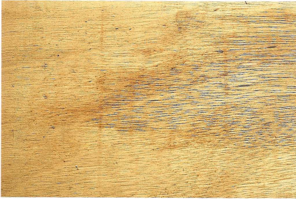
Fig 11.3 Oil stains on a bench top; clean habits are needed to avoid stains on the workpiece itself. The oil on the stone will slowly soak through the wooden box, which is a point in favour of having a separate sharpening area
