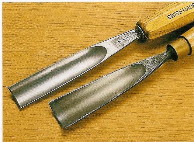
Fig 2.7 These two tools are not as different as they look. The maker of the lower gouge chooses to leave the tool black on the outside from the quenching, but polished inside to show the tempering colours; the upper one is uniformly finished all over, with the tempering colours polished out
