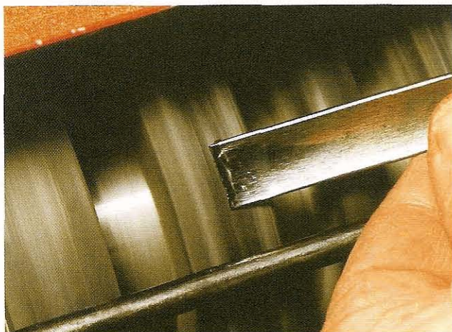
Fig 14.9 Presenting the bevel across the wheel is another option, and helps to keep the bevel flat
