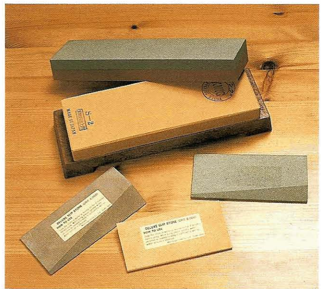
Fig 13.1 A basic set of waterstones: a combination stone lying on a polishing stone (mounted on a plastic base), and some water slipstones
