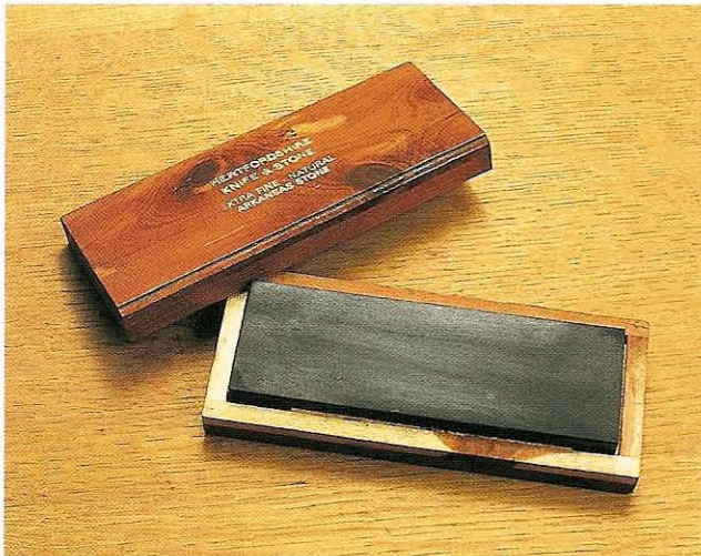
Fig 11.18 The black Arkansas stone, which is very black in appearance, is too hard for general purposes
