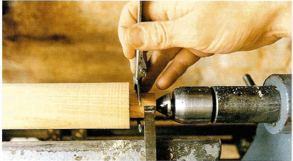
Fig 3.29 Sizing down to a close fit for the ferrule
