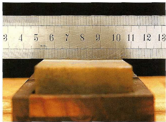
Fig 11.8 . . . but the centre will wear down. After a while this affects sharpening, and the surface then needs levelling
