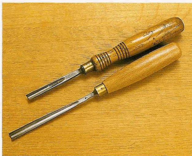
Fig 2.5 The old gouge at the top would originally have been as long as the modern one beneath. The reduction in length represents many years of carving and sharpening
