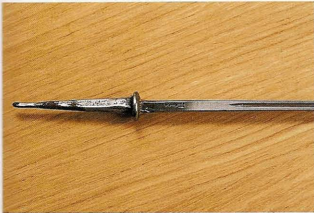
Fig 2.78 A straightedge applied to the photograph will demonstrate how far the tang is from true
