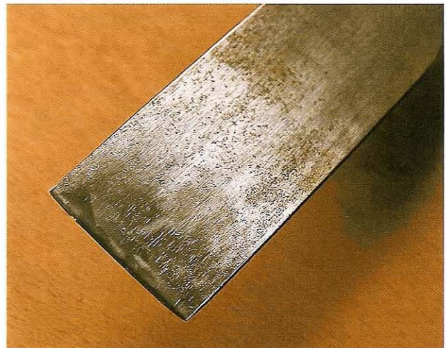
Fig 12.61 The notch in the edge of this gouge should be dealt with before putting it away
