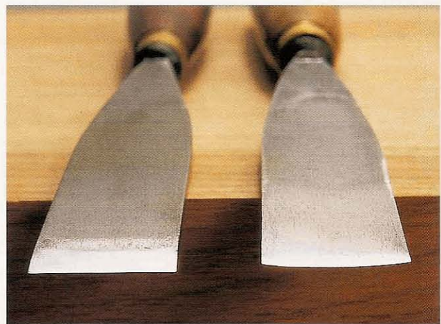
Fig 2.19 The flattest gouge (right) and a chisel (left), seen end-on. From this angle it is clear that the so-called 'flat gouge' is actually significantly curved
