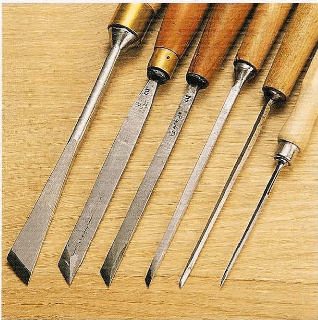
Fig 2.59 Skew chisels come in a range of widths. A newcomer should start with something in the middle (say \frac{3}{8} in/10mm) and buy different sizes only when they are actually needed – which might be never
