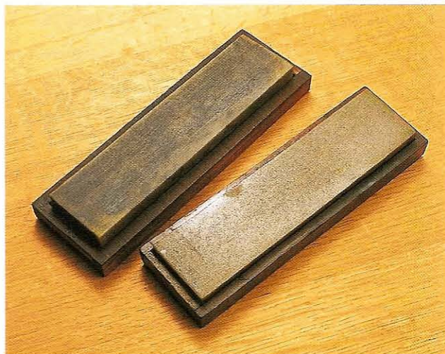
Fig 11.2 Reflections from a glazed oilstone (left) indicate that the pores are clogged with stone and metal particles
