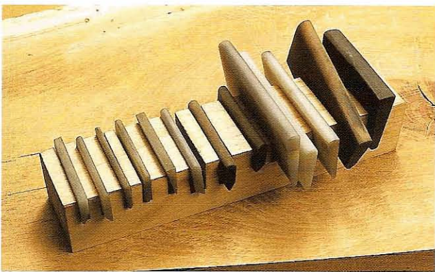
Fig 11.28 Small slipstones are quite brittle and easily chipped or broken. A rack like this will stop them damaging one another
