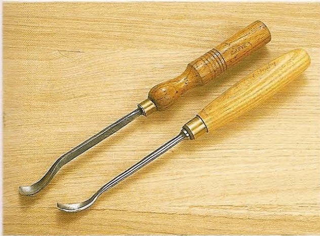
Fig 2.51 The shank of the frontbent gouge is normally rectangular, facilitating grip. The circular shape looks slicker, but I find that I can grip it less firmly. This sort of personal reason is why it is best to try tools in your own hands first, rather than depend on the catalogue photographs
