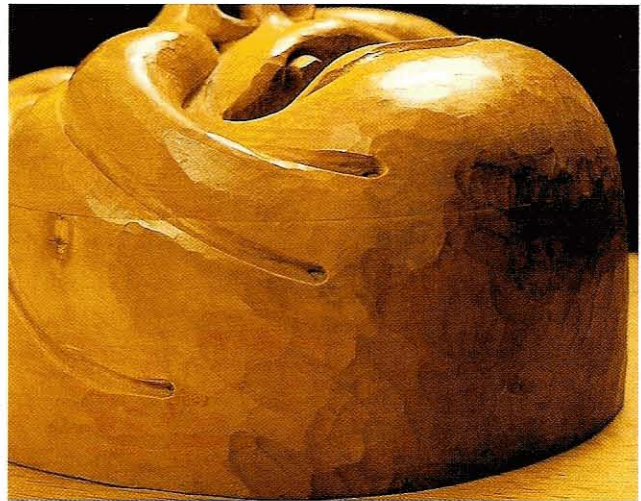
Fig 5.10 Quicker gouges will leave a pattern of deep cuts on a surface
