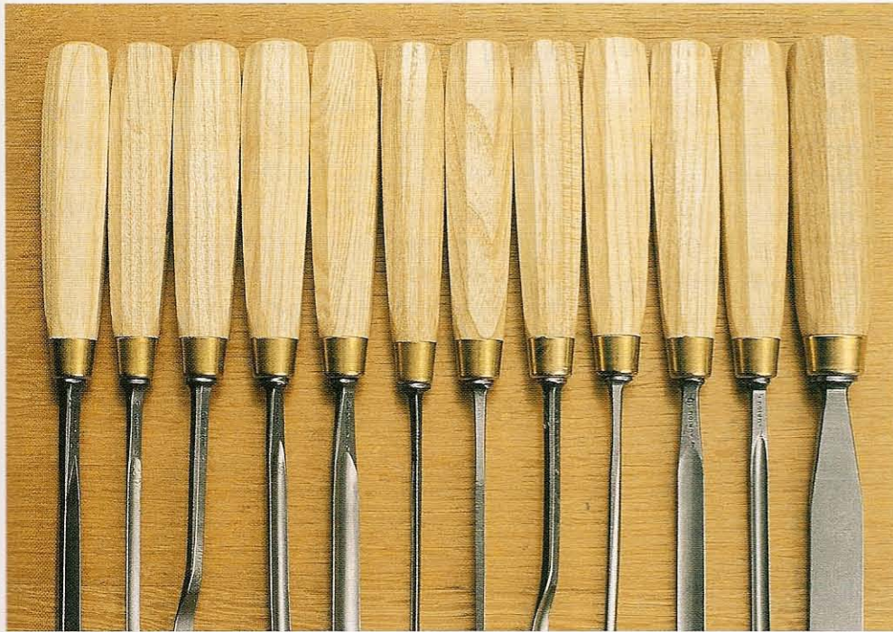
Fig 3.3 Although there is nothing 'wrong' with the handles in themselves, when such mass-produced handles are aligned on the bench, their similar appearance can be confusing
