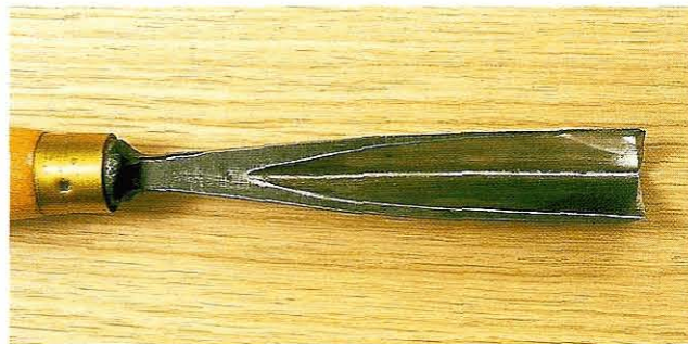
Fig 4.4 Differences in thickness between the walls of a V-tool make their equal sharpening difficult
