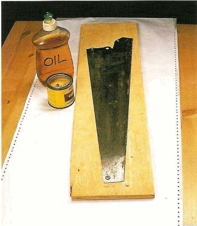
Fig 11.10 An old saw blade, with the handle removed and the teeth rendered flat and safe, is mounted on a board (preferably with a wipe-clean surface). This, together with light oil and an abrasive grit, is a simple means of flattening a benchstone
