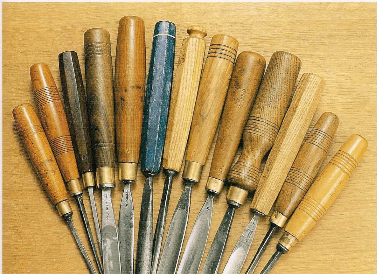
Fig 3.4 Differently shaped handles, also in different types and colours of wood, make tools more immediately recognizable on the bench
