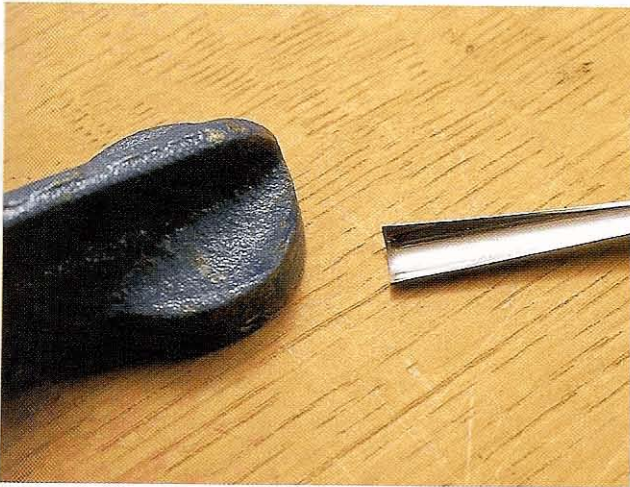
Fig 7.10 Delicate edge versus the cast-iron foot of a clamp – an unequal contest. Clamps are commonly used by carvers. Be aware that they are an easy source of damage to cutting edges which have taken time and effort to achieve
