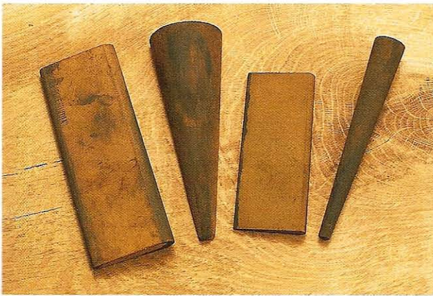
Fig 11.21 Larger Carborundum slipstones are useful for larger sculpture tools: (left to right) standard wedge shape; 'kidney' or half-conical; standard; conical
