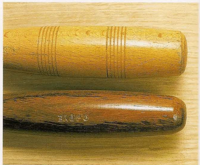
Fig 3.16 The wider end of the upper handle is a better target for the mallet than the other, which reduces towards a point
