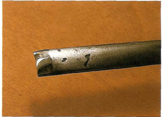
Fig 12.59 The curved reflection on this highly polished surface is a clue that the bevel has become rounded
