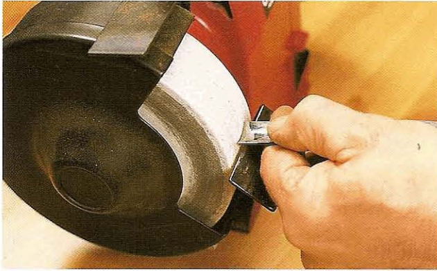
Fig 12.3 Perpendicular presentation (for clarity the grinder's perspex guards are swung up)
