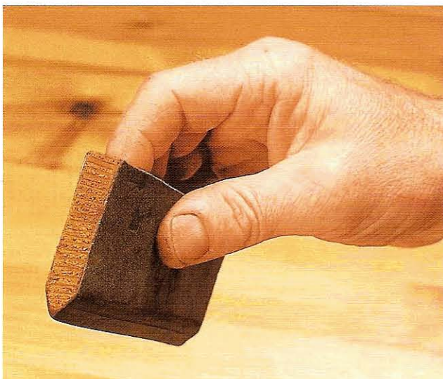
Fig 11.33 A slip of wood shaped specifically and covered with thin leather makes an excellent slipstrop
