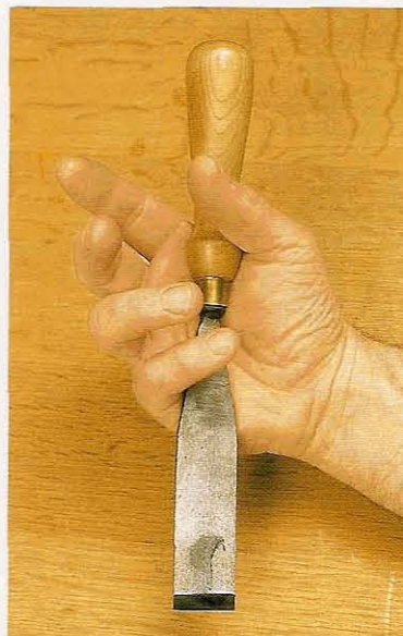
Fig 3.7 This design of handle which I have developed for sculpture gouges . . .
