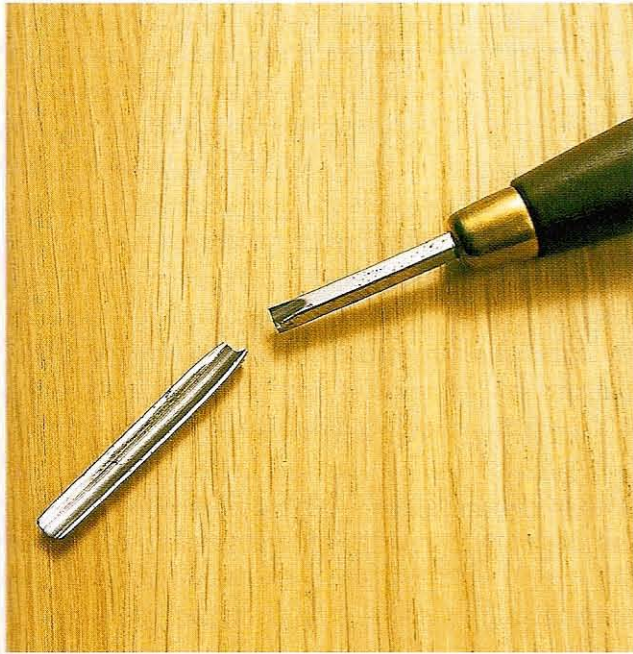
Fig 4.7 You cannot cold-bend the hardened part of a blade, however misaligned, without this happening
