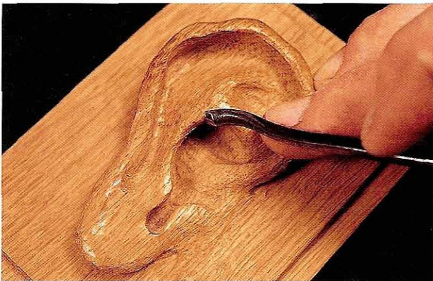
Fig 5.23 The backbent tool enters hollows in the upside-down position, shaping a surface which is concave along its length but convex from side to side
