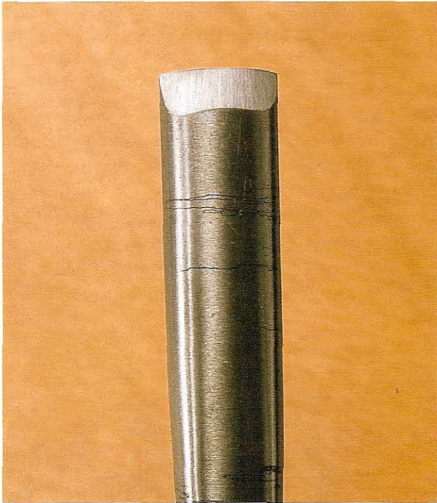
Fig 9.13 A carving tool bought with the bevel set but not sharpened usually has a flat bevel because of the large diameter of industrial grinding wheels. The bevel may also be quite even and a good size, like this one
