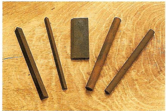
Fig 11.22 Small Carborundum slipstones: (left to right) large and small triangular; rectangular with bevelled edge; large and small cylindrical
