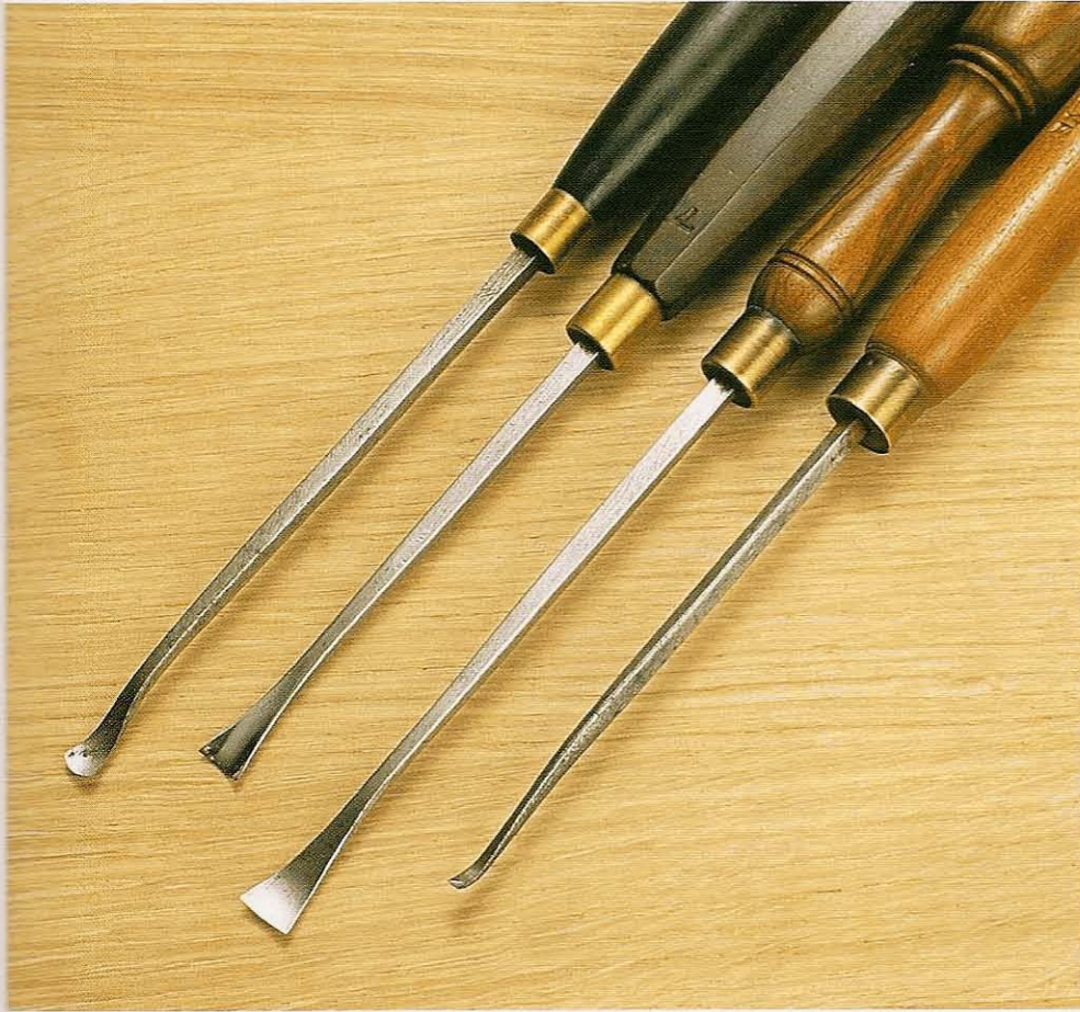
Fig 2.66 Typically, shoulderless tools are lightweight and are used for finishing and delicate work.
