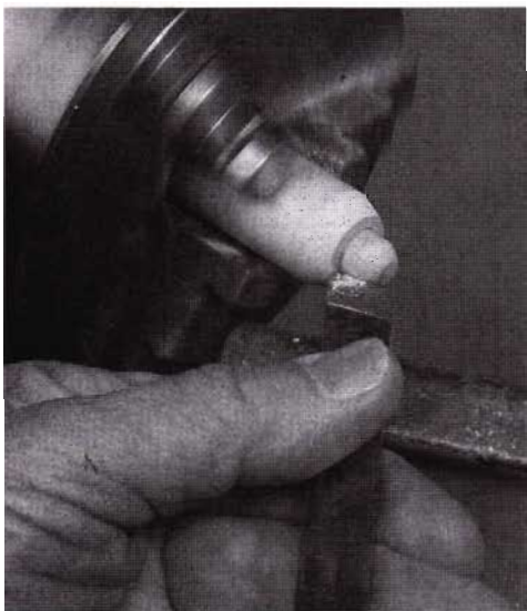
Use a wooden collet to hold the headlight while you shape the back end.
