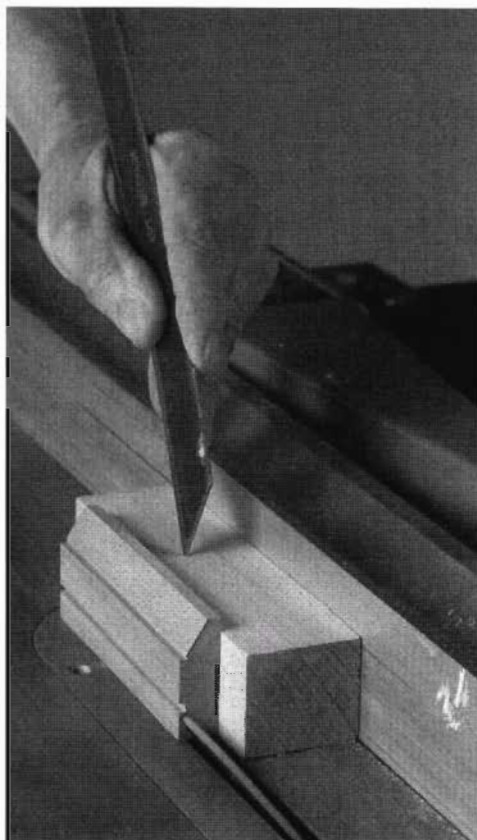
Always use a push stick when ripping small parts on the table saw. For added safety, fasten the workpiece to an auxiliary block with double-sided tape.
