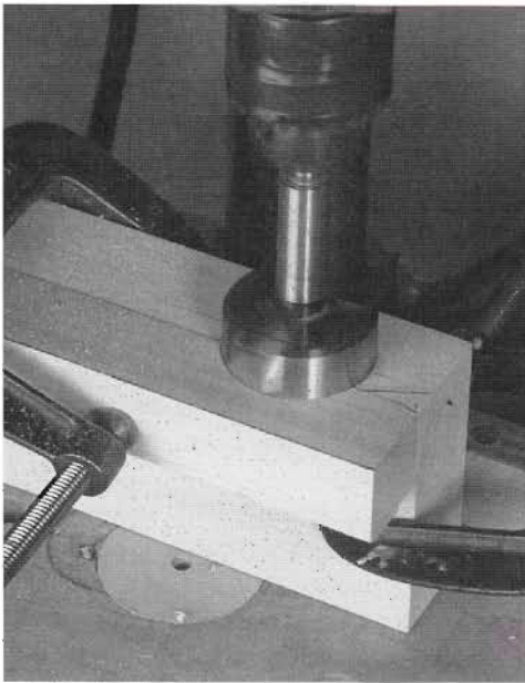
When cutting wheelwells, clamp a scrap block to the bottom of the workpiece to give the bit's center some stock to drill into and to prevent tearout along the bottom edge of the vehicle.
