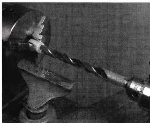
End-drill a cherry dowel to make the recessed hole for the headlight button.
