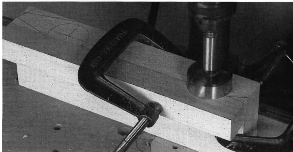
To prevent tearout when drilling the wheelwells, clamp an auxiliary block to the bottom of the body blank.
