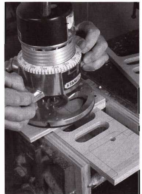
With the template clamped to the workpiece, rout the window opening.
