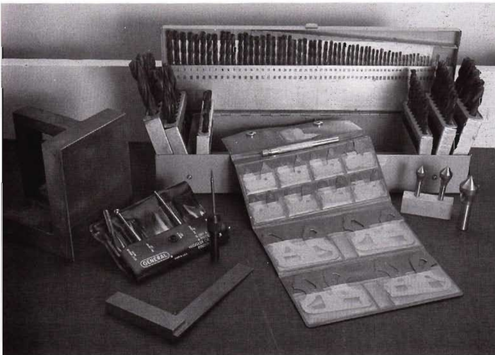
Specialty tools that come in handy for toymaking include (clockwise from top) a full set of drill bits, a set of metal-cutting countersinks, a set of radius gauges and a center finder. Also shown are a small machinist's square (foreground) and a right-angle steel block (left).
