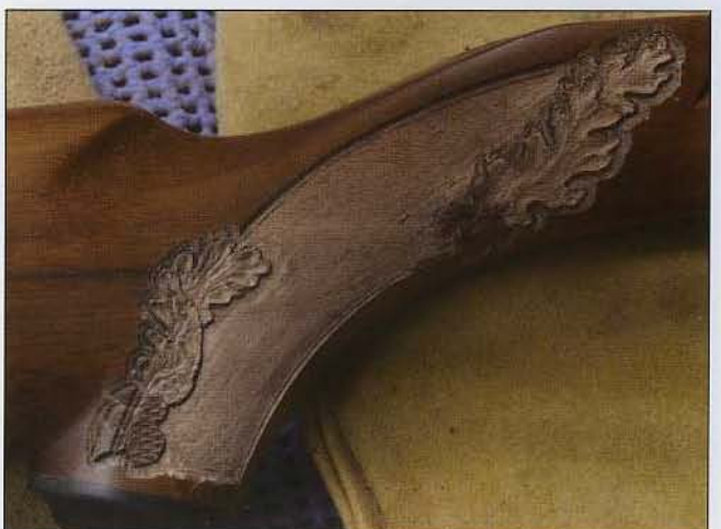
48 The leaves on both sides of the grip have been detailed. (Note that the acorns will be left until later.)
