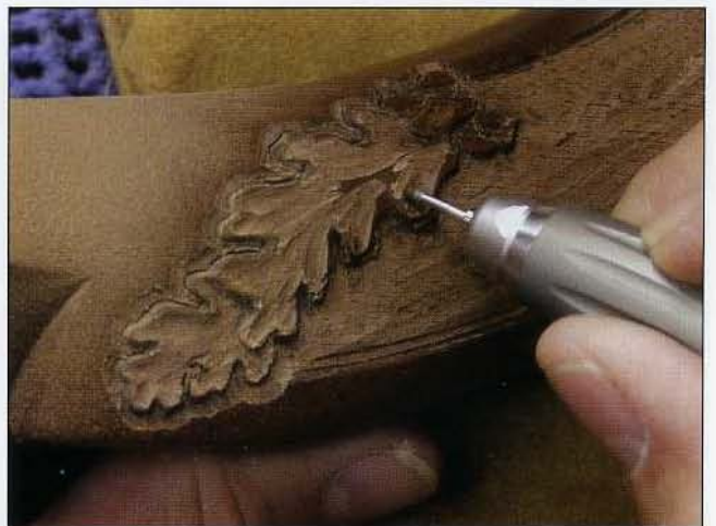
40 Remove additional wood from the lobes of the leaf to make the vein stand out more.
