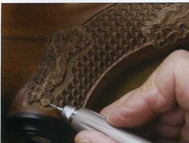
93 Remove a small amount of surface wood from the bottom half of the acorn.
