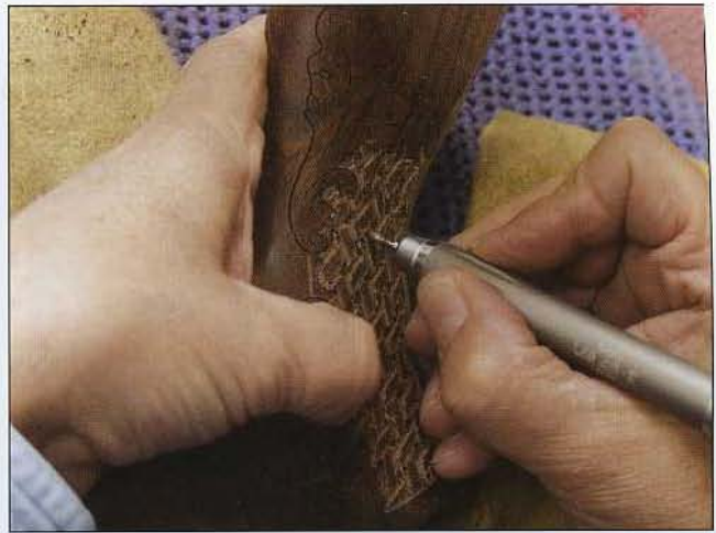
62 Turn the gun 180 degrees and make a fourth pass to remove wood on the opposite side of the horizontal weave.
