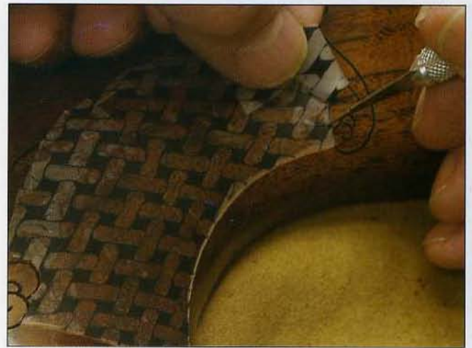
44 Carefully trim around the leaves in the bottom right corner of the design. Continue trimming around the remaining leaves.
