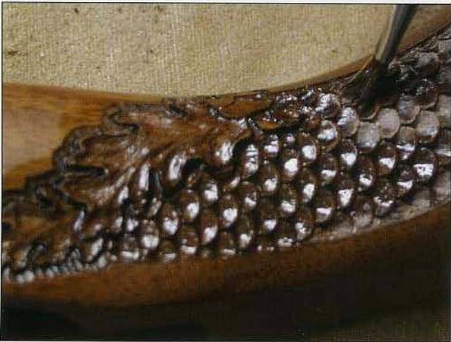
75 Apply a liberal coat of oil-based walnut stain to the fish scaled area with a flat brush. Choose a good quality 1/4-inch to 1/2-inch soft bristle brush.
