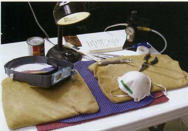
A limited number of tools are needed to carve gunstocks. I use a power engraver with a set of bits, plus the other items shown in this photograph. You can also carve beautiful guns with motorized tools and hand tools.
