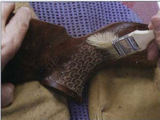
63 Use a paint brush to gently dust away and sawdust left on the surface and in the cuts.
