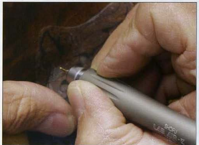
10 Fit the engraving tool with a carbide pointed bur. Begin outlining the first leaf.
