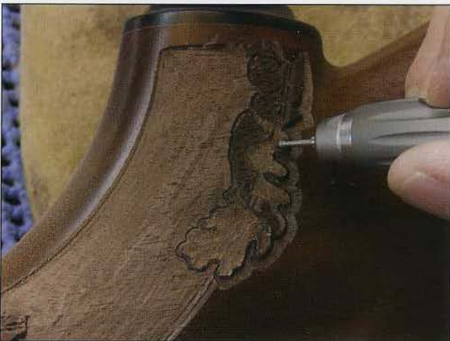
45 Remove wood from half of the lower leaf. Leave some extra wood in the center of this leaf to create the vein that runs the length of the leaf.
