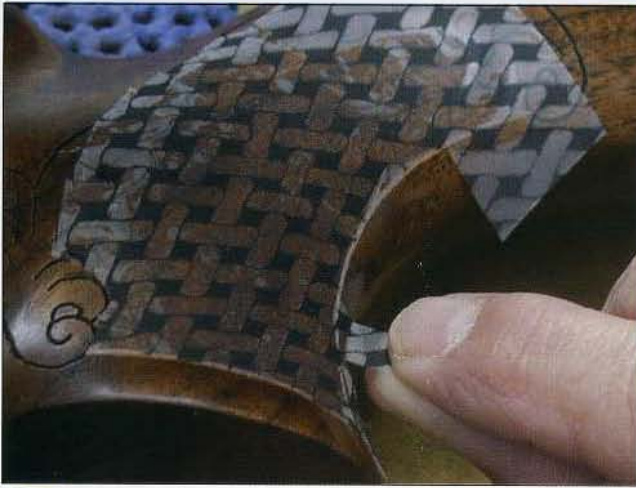
43 Using the X-Acto knife or your fingernail, gently lift the excess pattern and pull it away from the gunstock.
