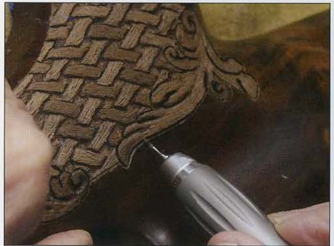
102 Using a carbide bur, very lightly trim all of the outside areas of the carving. Hold the tool at a consistent 45-degree angle.
