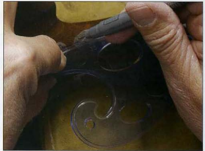
8 A French curve is used again to add the curve at the top of the design between the two leaf patterns.
