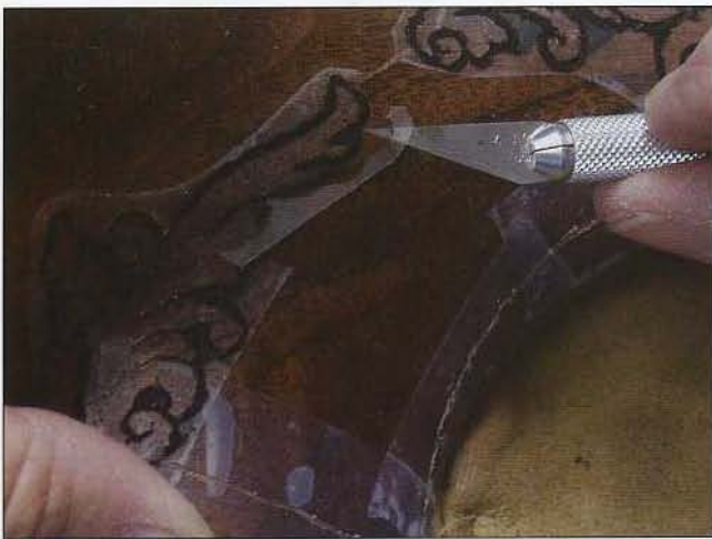
25 Carefully remove the pattern. An X-Acto knife or a fingernail may be needed to pry up the sticky-backed pattern.
