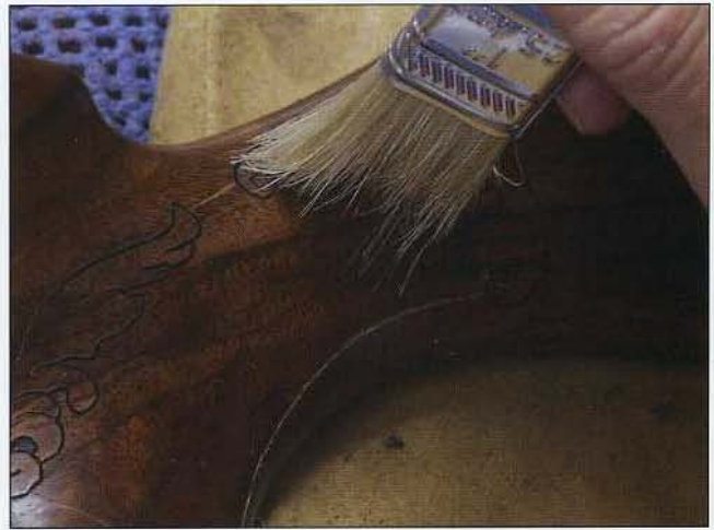
28 Using a regular paint brush, lightly dust the surface of the gunstock to remove any bits of pattern or fine sawdust left on the surface of the wood.
