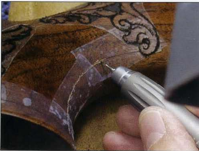
21 Hold the engraving tool at a 45-degree angle to the wood to make a v-shaped groove. This cut should be about \frac{1}{32} inch deep.
