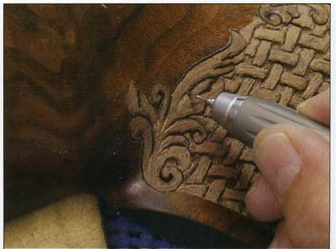
100 Hold the tool at a 45-degree angle to add a v-shaped groove to the leaf.
