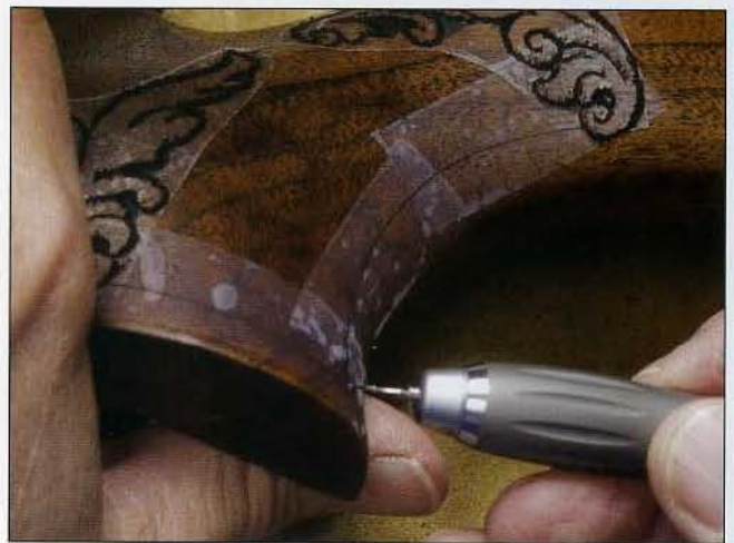
20 Switch to a carbide burr. Beginning at the lower left corner, start to cut in the line that forms the bottom boundary of the design.
