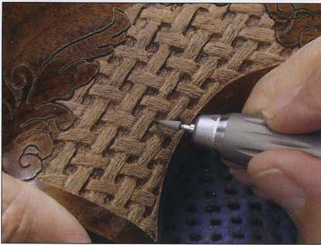
77 Slope the top of the vertical weaves in the first pass.
