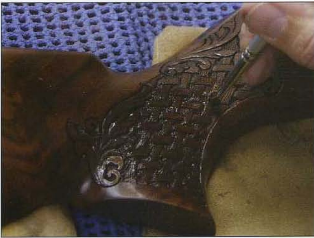
119 Allow the stain to dry 24 hours, then apply a finish to the carved surface with a paint brush. I use Tru Oil Gunstock Finish.
