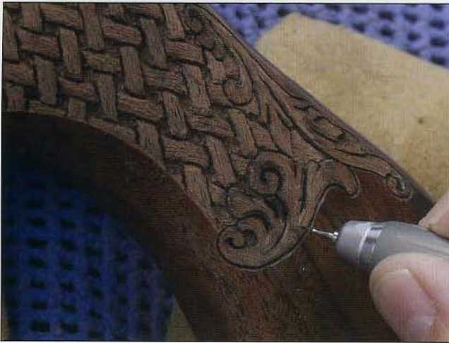
101 Make sure the angle of the tool is consistent as you create this groove.
