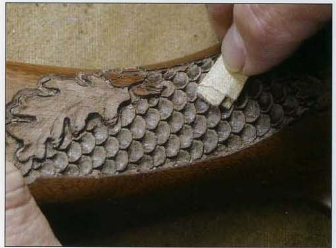
74 Sand the engraved fish scales lightly with 220-grit sandpaper. A light sanding will help to even out the fish scales.
