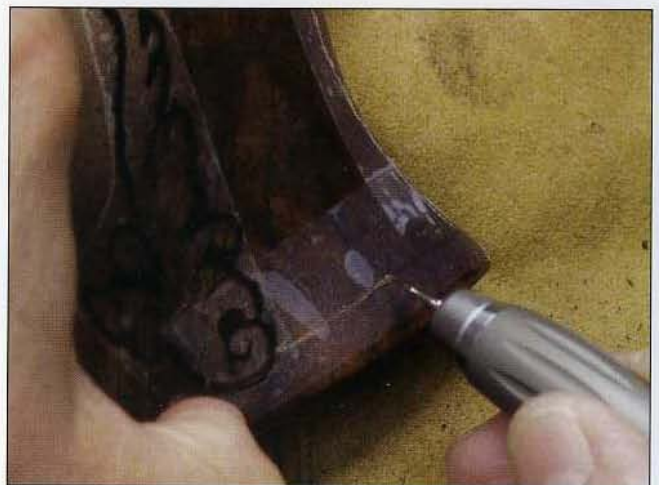
22 Next cut in the line that forms the boundary on the left side of the design.
