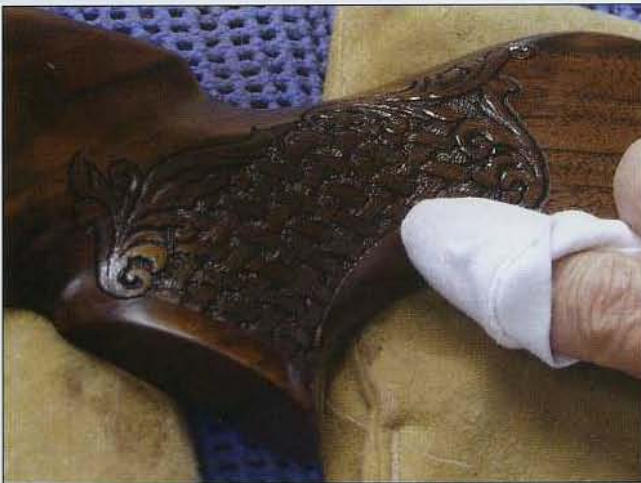
121 Wipe the excess finish off with a soft, clean rag.
