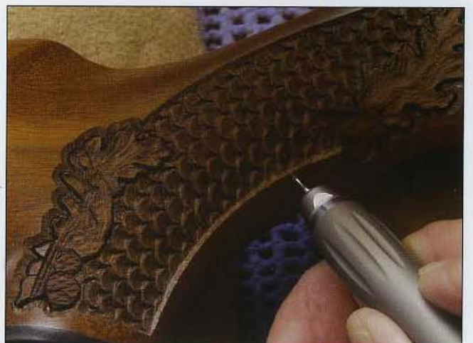
78 Using a carbide tip in the engraving tool, sharpen the bottom edge of the grip area.
