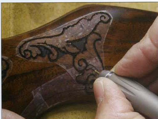
17 Cut the details in the second leaf. The detail lines are about \frac{1}{32} inch deep.
