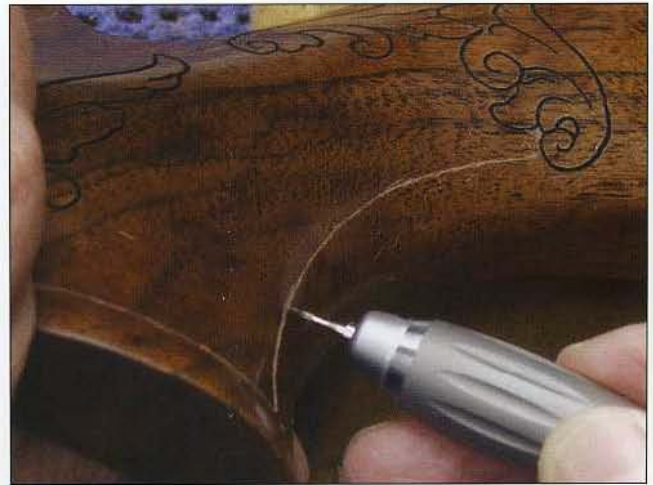
30 Make the lines that form the boundary of the design area more prominent by retracing them with the engraving tool.
