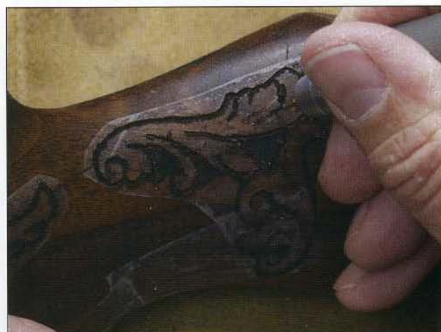
18 Be sure to cut all of the detail lines at this time.
