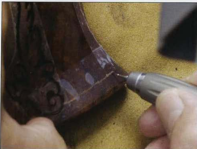
23 End this line where it meets the line at the bottom of the design. Be careful not to extend the line beyond the bottom line.
