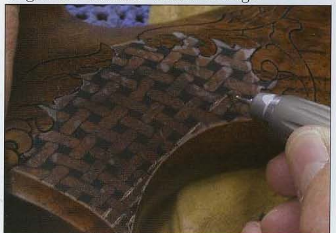
48 Fit the engraving tool with a carbide bur. Working from left to right and from bottom to top, begin cutting the horizontal lines of the basket weave pattern. Hold the tool at a 45-degree angle.
