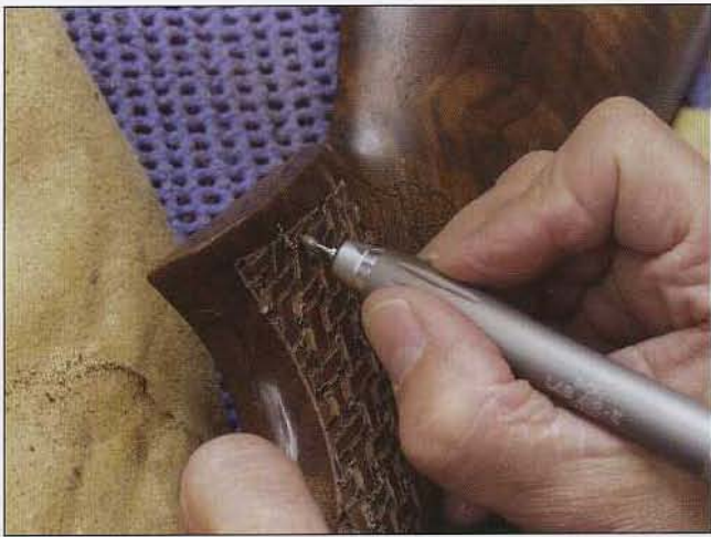
61 For the third pass, turn the gun and begin removing a small amount of wood where the vertical weave overlaps the horizontal weave.
