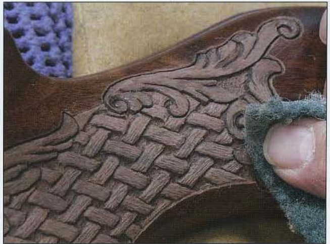
110 Rub the surface of the carving gently with a green Scotch Brite pad to remove any fuzz.
