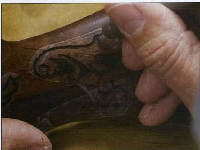
15 Continue outlining the leaf. Walnut is very hard and sometimes will burn if carved too fast.
