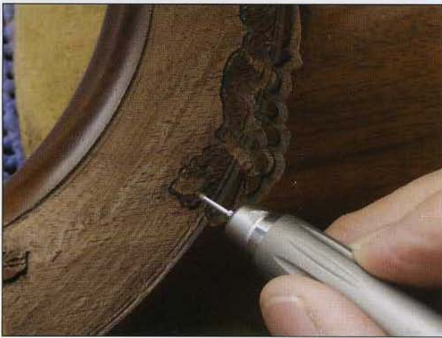
43 Turn the gun and begin to remove wood from the bottom-most oak leaf.
