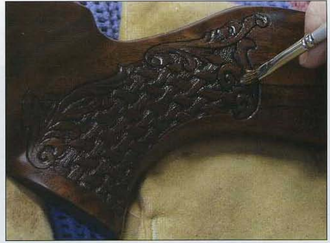
120 Work the finish into the crevices with the paint brush. Again, any finish beyond the boundaries is easy to remove and will not sink into the uncarved surface.
