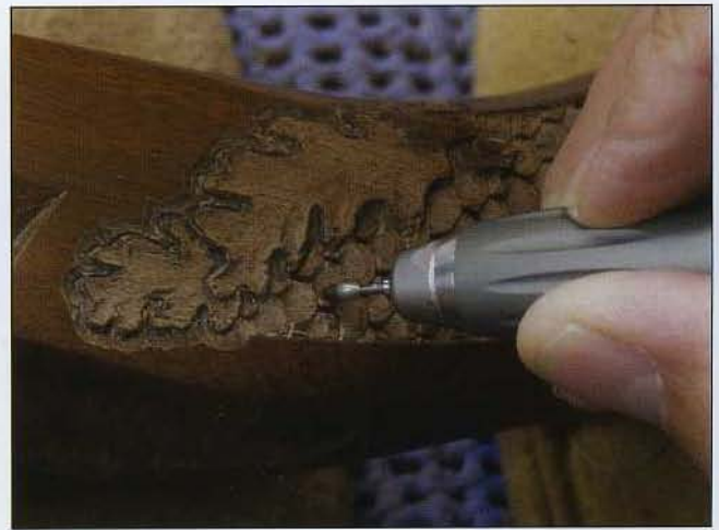
68 The final step to engraving the fish scale pattern is to burnish each scale. Switch to the large football diamond and carefully smooth the inside of each scale.
