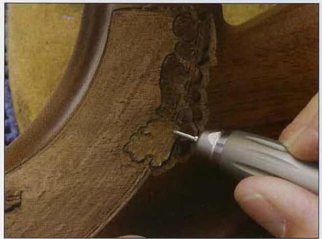
44 Remove the wood from the center of this leaf. As before, strive to make the leaf concave. The center of the leaf should dip in while the edges of the leaf remain raised.
