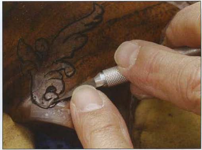
26 Because the engraving tool cut through the pattern, the pattern will not lift off the gunstock in one piece.
