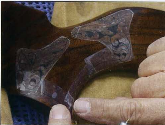
9 The pattern has been positioned and marked on the gunstock. You are now ready to begin carving.
