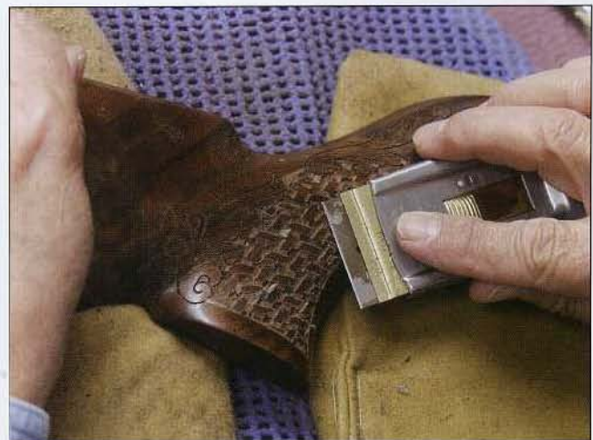
64 Used carefully, a scraper is an ideal tool to remove any remaining bits of the pattern that are still stuck to the surface of the wood.
