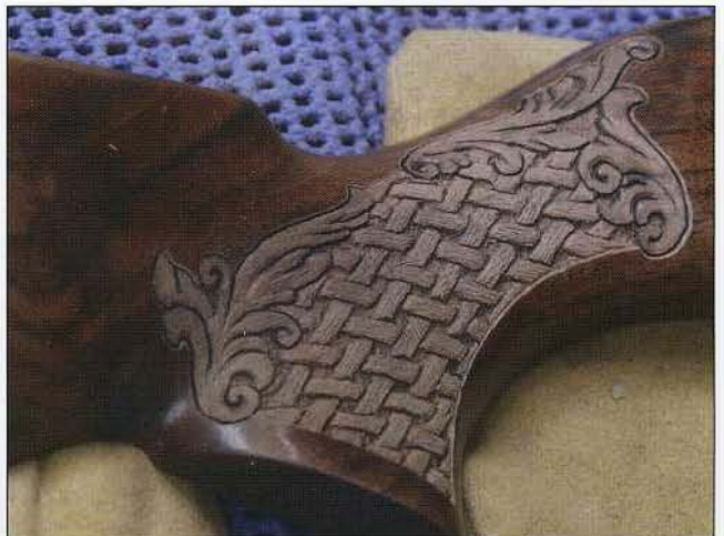
112 The sanded carving is ready for stain. Be sure to brush away any sawdust before beginning the next steps.
