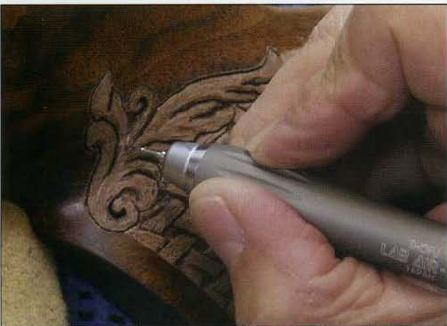
99 Fit the engraving tool with a carbide bur. Begin to add detail to the leaves.
