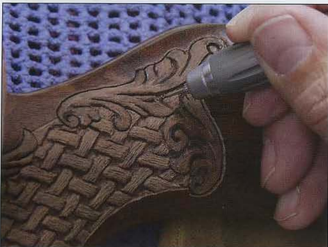
105 Clean up the spaces between the leaves with a #2 round carbide bur; then stipple those areas to create the illusion of a background.
