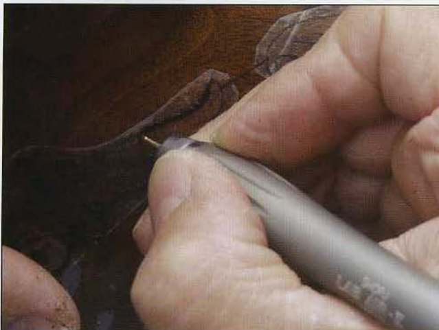
11 Continue outlining the leaf. Be sure to hold the tool perpendicular to the gunstock. The resulting cut should be about \frac{1}{16} inch deep.
