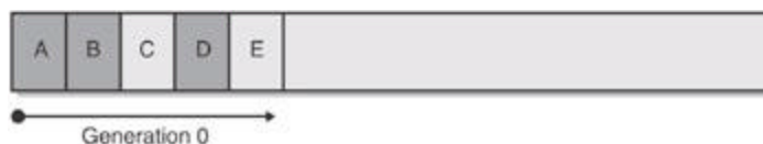
Figure 19-7 : A newly initialized heap containing some objects; all in generation 0. No collections have occurred yet.
