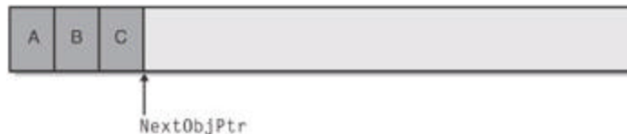
Figure 19-1 : Newly initialized managed heap with three objects constructed in it
