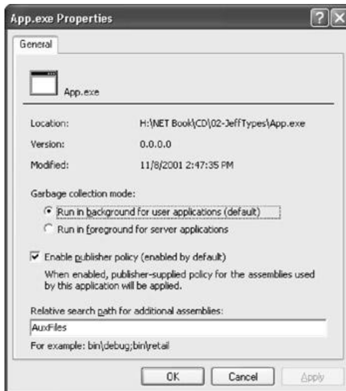
Figure 19-15 : Configuring an application to use the concurrent garbage collector using the Microsoft .NET Framework Configuration administrative tool
