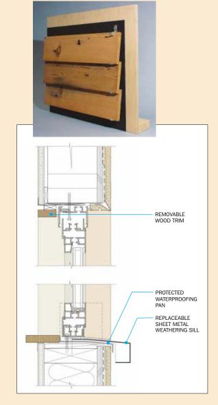
Students would be moved to portable classrooms, and the whole process was a classic example of wasted materials, time, and money. To reduce time, the windows at Chartwell are detailed for disassembly with a minimum of waste. Similarly, the wood siding is fastened with clips that are screwed into the backing for ease of disassembly.
