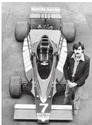
■ The Brabham BT42 (above), the BT46 with the heat exchangers instead of conventional radiators, plus the brilliant but banned BT46B "fan" car.
