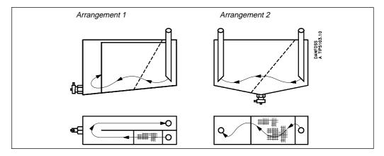
To increase the ability of the tank to separate dirt and water, the bottom must be slightly inclined (deepest end opposite the inlet/outlet end). An ordinary cock (without handle) is fitted so that impurities can easily be drained off. Increased separation of the air that is always present in the oil can be obtained by fitting an inclined coarse metal strainer (approx. 25-50 mesh/ inch) by the return line.
