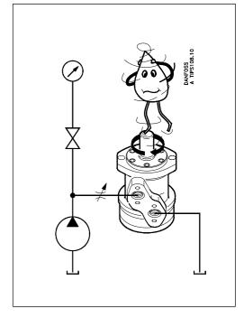
If no flow meter is available, a Danfoss hydraulic motor can be fitted instead. The displacement of the motor per revolution with unloaded shaft is very precise and to find flow all that is necessary is to count the number of revolutions per minute and multiply the figure by the displacement, as shown in the following examples:
