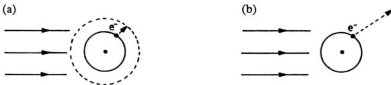
Fig. 2.8. (a) Photoabsorption out of a monochromatic beam of photons: An electron is elevated from a low-lying bound state to a higher lying bound state. (b) Photoionization: A bound electron is excited into a continuum state
