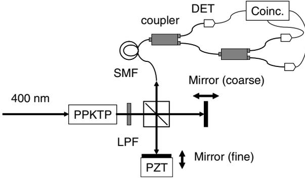
**Fig. 18.** Experimental setup for four-photon interference. SPDC photons from a PPKTP crystal were divided by two fiber couplers after passing through a Michelson interferometer composed of a beam splitter and two mirrors. The position of one mirror was tuned by PZT
