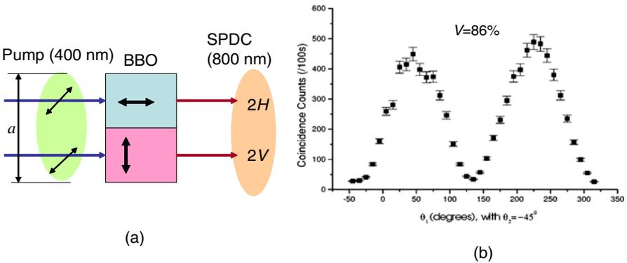
**Fig. 16.** (a) The two-crystal geometry. Two identical crystals are stacked, with their optical axes aligned in perpendicular directions.  $a$  is the diameter of the pump laser with  $45^\circ$  polarization. (b) Two-photon quantum interference for polarization variable. One polarizer is fixed at  $45^\circ$ , while the other polarizer is rotated with  $10^\circ$  steps
