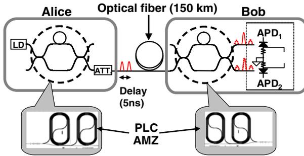
**Fig. 3.** Schematics of the integrated-optic interferometer system for quantum key distribution. *LD*: laser diode, *ATT*: attenuator, *APD*: avalanche photodiode, *DS*: discriminator, *CT*: counter, *H*: 180° hybrid junction
