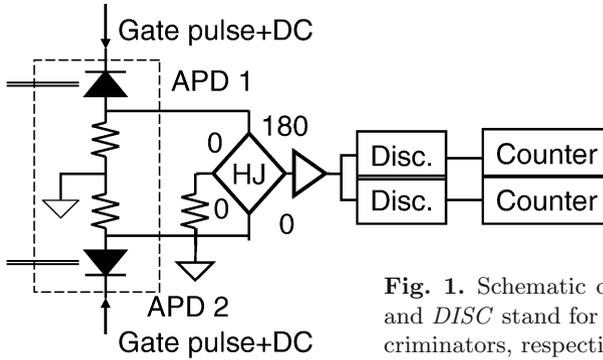
**Fig. 1.** Schematic of the photon detector. *HJ* and *DISC* stand for a hybrid junction, and discriminators, respectively
