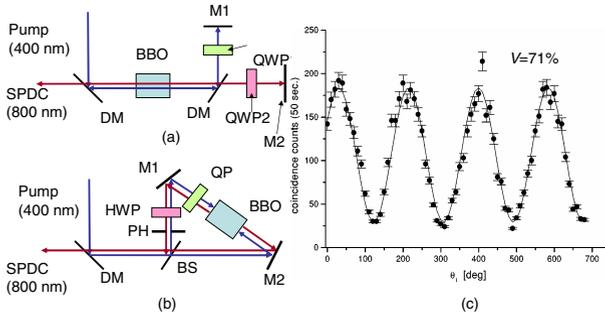
**Fig. 17.** (a) Michelson interferometer based SPDC. *QWP*: quarter-wave plate; *QWP1* for 400 nm with  $0^\circ$ , *QWP2* for 800 nm with  $45^\circ$ ; *M1*: mirror for 400 nm; *M2*: mirror for 800 nm. (b) Sagnac interferometer based SPDC. *HWP*: half-wave plate for 800 nm, *BS*: beam splitter, *QP*: quartz plate, *PH*: pin hole. (c) Two-photon interference of SPDC photon pairs generated in a Sagnac interferometer. One polarizer is fixed at  $45^\circ$ ; while the other polarizer is rotated
