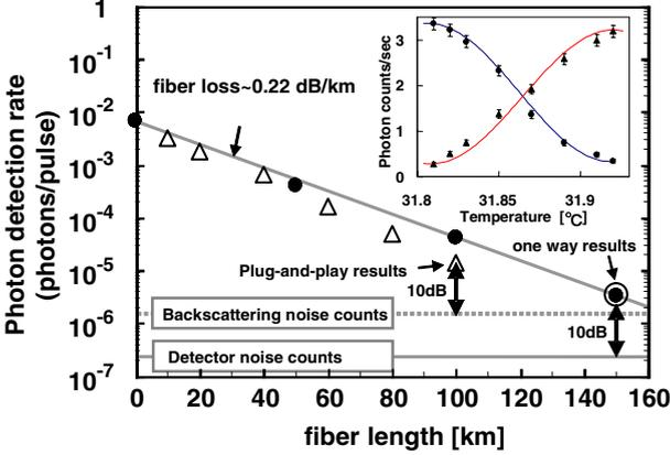
Fig. 4. Photon counting probability against transmission distance. *Open triangles* indicate the results in the P&P system. *Inset*: Fringe observed in photon count rate, obtained by changing the device temperature at 150 km
