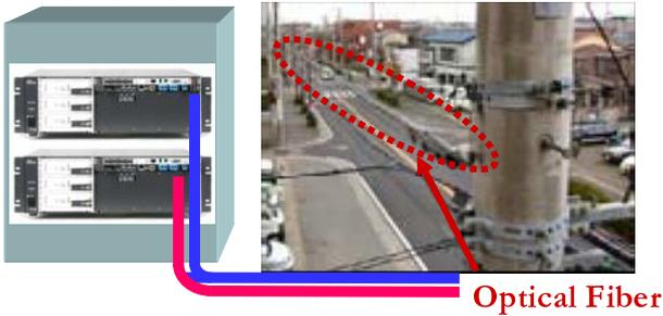
**Fig. 8.** Prototype of a QKD system fully equipped with functions for stable operation (*left photograph*). A fortnight quantum key generation field trial over commercial access fibers was done with the system. The fiber cable was installed on the electric poles (*right photograph*)
