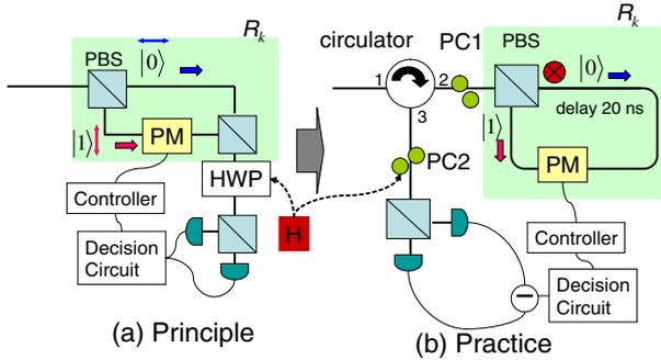
**Fig. 10.** Quantum circuit for measured quantum Fourier transform implemented by fiber optics. (a): The principle of the circuit. (b): Practical circuit. *PBS*, *PM*, *HWP*, and *PC* stand for polarization beam splitters, phase modulator, half-wave plate, and polarization controllers, respectively
