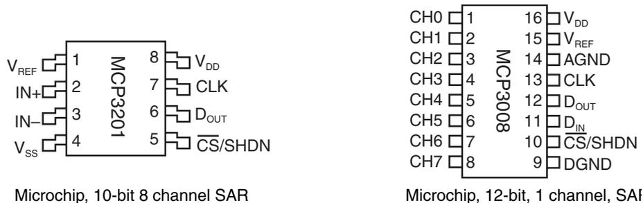
**Figure 11.13:** The SAR converter, regardless of resolution, usually has at least two ground connects; AGND ( $V_{SS}$ ) and DGND ( $V_{SS}$ ). The converters illustrated here are the MCP3008 and MCP3201 from Microchip.
