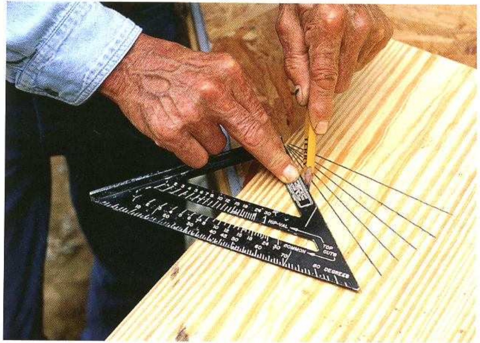
GET THE RIGHT ANGLE. A small, triangular rafter square is designed to lay out 90-degree and 45-degree angles quickly, but it's also capable of laying out just about any angle you might need.
