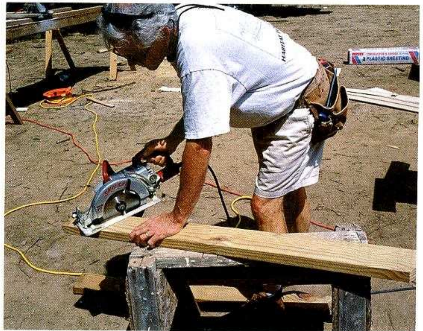
WORM-DRIVE SAW. Larger and heavier than a sidewinder saw, a worm-drive saw has its motor in front of the blade.
