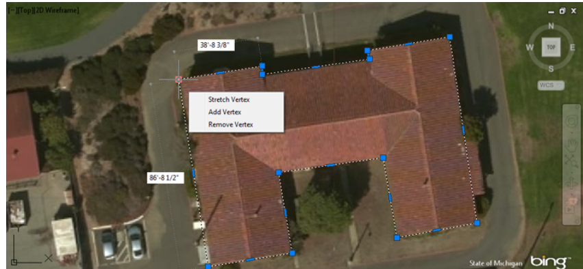
FIGURE 13.21 Dimensions from a building outline
