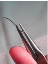
6.) Center the edge of your pliers across the back of the now-folded-over wire and the middle of the spiral. Bend up 90 degrees so the wire is coming up out of the center of the spiral.
