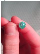
8.) Grasp directly against the bead with your needle nose pliers; then bend the wire 90 degrees against the plier edge.
