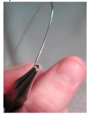
3.) Grasping the flat area of the spiral with your needle nose pliers, continue the wire around until you are on the opposite side of the first end, which is now tucked neatly in the center.
