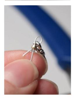
3.) Use crimp pliers (location 1) to secure crimp bead. The crimp bead will look like it has been bent in half. Turn crimp bead 90 degrees and use location 2 to compress crimp bead. This will result in crimp bead folding over on top of itself where the original bend was formed.
