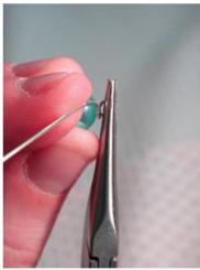
13.) Cut the excess wire from the wrapped coil, pushing the flat back end of the wire as close to the coil as possible.
