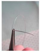
16.) Grasp a small distance from the bend; create your eye loop and wrap loop as before. Cut away any extra wire.
