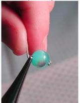
9.) Grasp the wire about 1/8th of an inch (or somewhere around 2mm) away from the bend with your round nose pliers.
