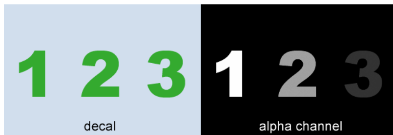
Decal masking with alpha channel to create transparent decal.
