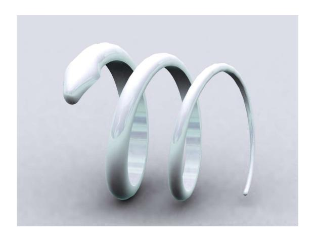
Begin by drawing a cylinder and then a curve-helix shorter than the cylinder but with the same radius and Turns 2
