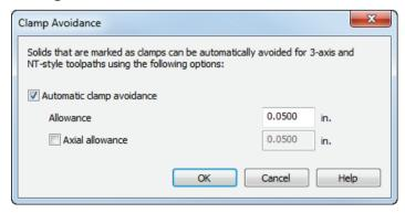
**Automatic clamp avoidance** — Select this option to automatically avoid solids that are marked as a clamp. To mark a solid as a clamp, right-click its name in the **Part View** and select **Use Solids as Clamp** in the context menu.
