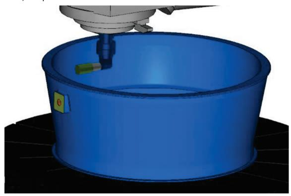
This enables you to create difficult features, such as internal pockets, and enables you to create multiple features without repositioning the part.
