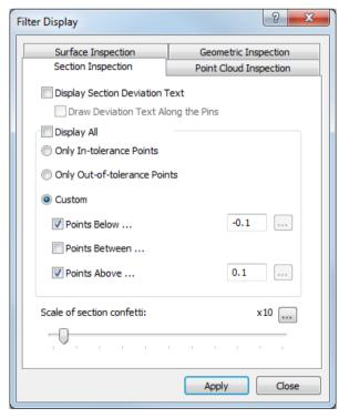
5 To show the calculated deviation of each probed point alongside its confetti, deviation line, or vector, select the **Display section deviation text** check box.
