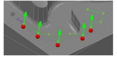
To create the probe path for a CNC Surface Points group using guided surface points:
