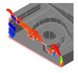
PowerINSPECT OMV Pro compares the measurement results to the CAD data and displays the deviation using colour:
