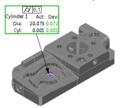
**10** Repeat steps 6 to 9 to continue displaying form tolerance requirements in the labels for other Geometric items.
