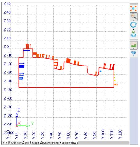
The background colour of the **Section View** tab is controlled using the settings for the **CAD View** tab. To change the colour, use the **Colours > General** page of the **Options** dialog (see page 40).
