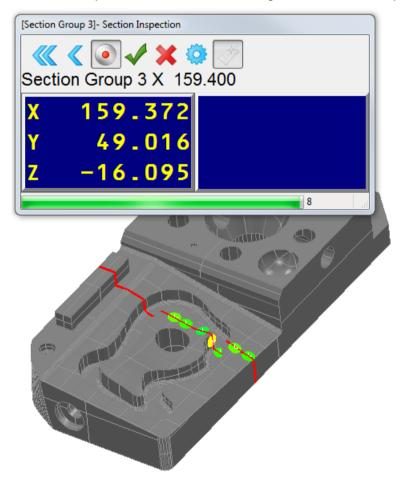
The left of the **Section Inspection** dialog displays the coordinate of the point on the section plane nearest the probed point. The progress bar at the bottom of the dialog shows how close the probed point is to the point on the section. When the probed point is in-tolerance, a coloured disc is displayed on the model, and the right of the dialog shows the distances between the probed point and the point on the section.
