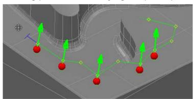
To create the probe path for a CNC Surface Points group using guided surface points:
