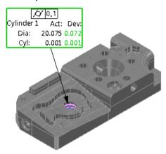
**10** Repeat steps 6 to 9 to continue displaying form tolerance requirements in the labels for other Geometric items.
