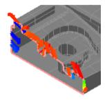
PowerINSPECT CNC compares the measurement results to the CAD data and displays the deviation using colour:
