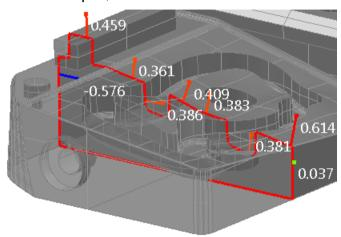
6 If the deviation of probed points are displayed as lines or vectors, select the **Draw deviation text along the pins** check box to display the calculated deviation along the length of the line or vector.
