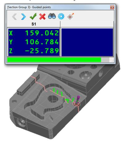
The left of the **Guided Points** dialog displays the coordinate of the current guided point. The progress bar at the bottom of the dialog shows how close the probed point is to the guided point. When the probed point is in-tolerance, a coloured disc is displayed on the model, and the right of the dialog shows the distances between the probed point and the guided point.
