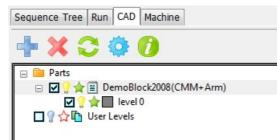
The coloured box indicates the colour with which each level is displayed in the **CAD View**. Change the colour by left-clicking the box, and assigning a new colour from the palette.
