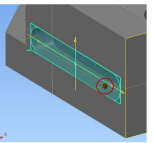
The warning referring to approach and retract distances has been addressed but, because the probe remains in the vertical orientation required for the previous feature, a probe path to measure the slot in the side face cannot be created.
