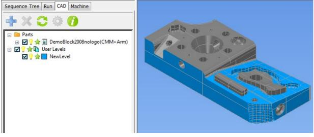
This technique can be useful if there is a large quantity of data in a view. Each layer has an associated colour, which is used when colour shading the model. To change the shading colour of a level, left-click the small coloured box to the left of the level's name, and select a new colour from the palette.
