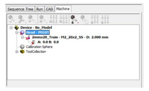
3 Select the PH10T in the machine tab probe view and click on the 'Calibrate selected item' icon
