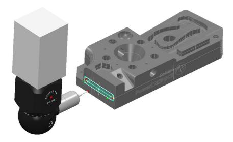
The probe path simulates without collisions, but leaves the probe in a potentially unsafe position.
