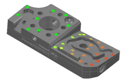
The example shows the surface used for the alignment, Plane 1, is within tolerance. However, the other top surface is out-of-tolerance towards the other end of the block. We can attempt to improve the alignment by creating a Best Fit item that includes the results of the inspection group.
