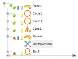
The brown icon on the slot and its reference plane indicate they have probe path collisions.
