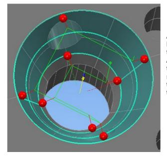
Another method of avoiding the holes in the surface is to create the probe path using an **AutoTouchTrigger** method, and then switch to the **UserDefined** method. This enables you to drag the points to a better location on the cone surface.
