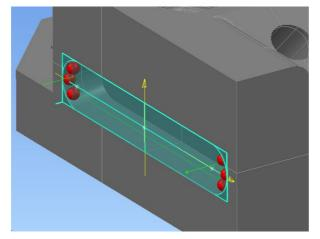
By setting the probe to Auto Orientate, a probe path is successfully calculated. Auto Orientate orientates the part or probe based on the surface normal of the first point in an inspection group, or the overall normal of a geometric item.
