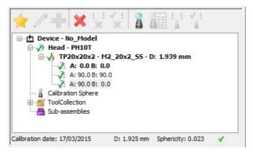
In addition, icons indicate whether the probe and probe position are calibrated  $\checkmark$ , calibrated but outside form tolerance  $\checkmark$ , or uncalibrated  $\blacksquare$ .
