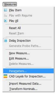
Select **Parameters** to open the **Measure Parameters** dialog. This dialog contains a series of tabs that relate to different areas of PowerInspect CNC.
