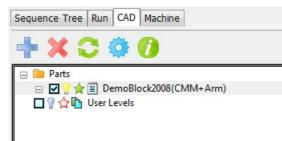
When you select the tab, the window displays the **Parts** folder and the **User Levels** area. Click the  $\Box_{\mathbf{x}}$  icon to open folder and display the sub-items.
