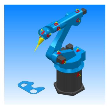
Select and activate the **Knife** toolpath and perform a simulation. The result is bad as the robot head (the F axis) doesn't follow the edge of the part:
