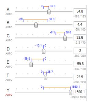
It is possible to apply additional constraints on an axis. Right click on the **-1600/1600** on the Y axis. In the menu, select and apply the value of 1200 for the maximum value and 1000 for the minimum value. Use the Enter key after entering the values.
