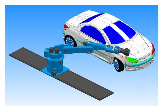
The suggested position is not very good. Hit the Play button. The toolpath cannot be executed, since a singularity appears. It should be better to move the robot on the Y axis and orient the head.
