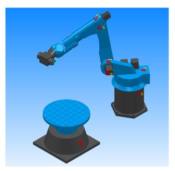
The default origin is wrong (the part is inside the robot base). To put the part on the rotary table, select the **Center Table** origin in the Robots tab:
