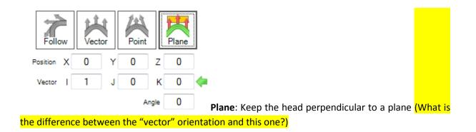
Another tool is available if you want to change manually the orientation of the head of a specific area on an existing toolpath. Delete all and open **the Surface Trimming – Bucket Seat** project:
