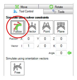
Now, the robot head will follow the toolpath, but with the wrong orientation. To orientate the tool in the correct position, we will have to add an additional angle parameter. The green arrow in the previous figure shows where it is possible to add information. By adding the 90 (**followed by enter**) value in the angle textbox, the tool knife will follow perfectly the toolpath:
