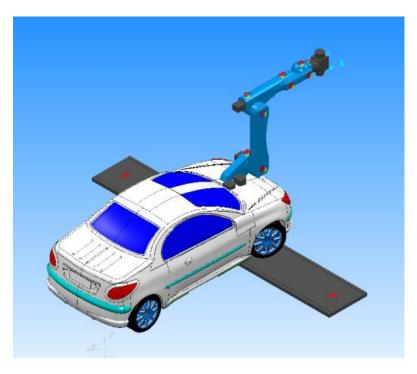
As we can see, the robot is not positioned correctly. In the **Robots** tab, select the **Center Right (Rail)** origin. Select an ISO 4 view (Ctrl + 7).
