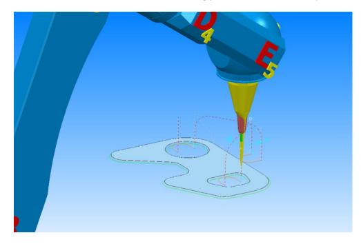
Make sure that the **Lock graphics display** is unticked and click on the **play** button. The robot will move along the toolpath.
