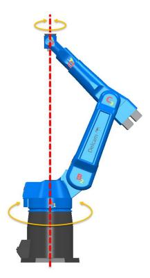
Additional constraints or modifications in the toolpath are sometimes essential to prevent the robot to have a singularity.
