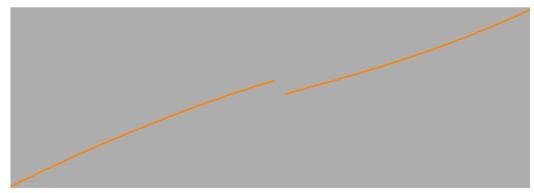
2 When creating a composite curve, PowerMILL automatically stops when it reaches the gap.
