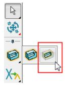
This ensures the next general edit will now apply to the selected sub-items only. In this case the **cylinder** and the **Boolean Remove** which created the hole through the block.
