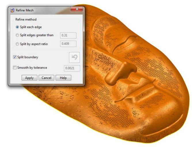
The **Refine Mesh** option can be used to increase the **density** of the triangles in the mesh by **dividing** the **existing triangles** and refining the triangles by **curving** the original **triangles** to create a **smoother mesh**.
