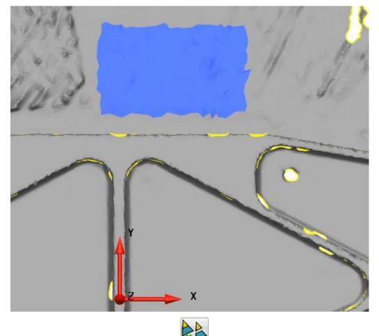
**35** Divide the Mesh by Selection **Selection** located on the Mesh Edit toolbar.
