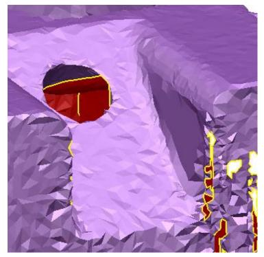
**Importantly**, taking a look at the **right hand side vertical wall** of the cut (**above**), we can see that due to some **missing data** and the **hole** being '**filled**' when the **mesh** was created, the wall is not quite vertical. We can solve this issue by **Moving** a **copy** of the **surface** we generate from the **opposite wall**.
