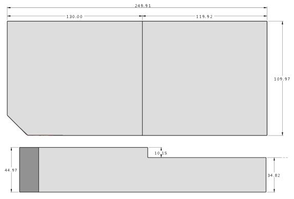
As you can see from the **above images** the data has provided a mesh that has **closely represented** the part. Any number of variables can cause these small descrepencies in **sizing**. However if we are **reverse engineering** to **recreate** the exact model we can now use the **Direct Solid Modelling** techniques shown earlier to perform **General Edits** to **individual faces** of the **solid model**.
