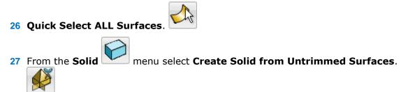
**28** This **Automatic Trimming** tool will attempt to **create** the **most relevant solid** from the **selection** of **untrimmed surfaces**.
