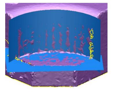
We have now successfully **fitted** and **created** a **partial cylinder**. Next, we need to check the **location** of the **centre point**. On the model this should be where the two vertical edge faces would meet, therefore we will **create a workplane** at this location and then ensure that the **X** and **Y coordinates** of the **primitive cylinder** are **0**.
