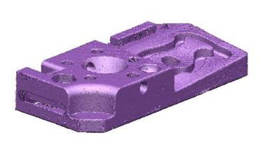
In the **graphics area** we now have the **mesh** created from the **imported/scanned point cloud** and an **alignment surface** sized to fit the **face** we have chosen to use to help **align** with **planar surface**, and therefore the **origin** of the **active workplane/world datum position**.
