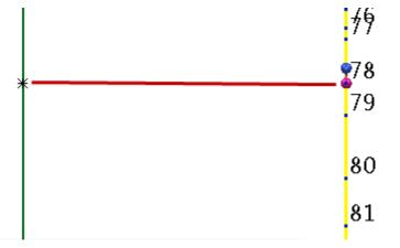
As you can see the **new point created** (**Point 78**) is **adjacent**. This means we can now create the **flat inbetween** this **point** and then end of the **curve**, which will **match** the **first curve**.
