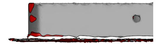
Removing any unwanted data in the mesh will reduce the overall mesh size and **complexity** and **speed** up the **software graphics**. We will do this using **limit** selection from a new workplane, and as we already have isolated a small section to provide the overall part depth and placed it on a separate level, we can remove the rest of the extra data.
