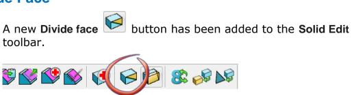
Use this functionality to divide the faces of the selected solid using wireframe. This option is useful if you need to make small, localised changes, or to limit the effect of Direct Modelling editing operations (see page 32).
