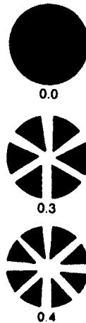
Fig. 3.6.6. Circular mode shapes of laser beams. (From A.E. Siegman, An Introduction to Lasers and Masers , McGraw-Hill, New York, 1971.)
