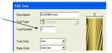
3. The simplest way is to change the tool number by first highlighting the tool in the Toolpaths Tab.
