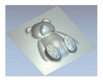
The two toolpaths in the sequence listed are simulated on screen and the final result shown (after finishing operation)
