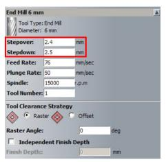
The **default tool parameters** (for Wood and Plastic 6mm End Mill) are shown. Changing values in this form do no affect the original tool stored in the database.
