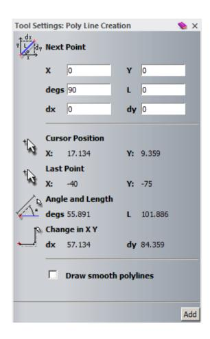
**Polylines** can be generated by entering **absolute co-ordinates** in the **X** and **Y** area, by angles and line length, as **relative co-ordinates** using the **dx** and **dy** (distance from last point) or by clicking with the cursor.
