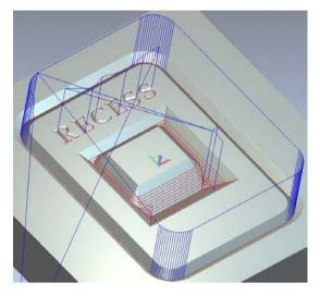
The toolpath is calculated creating 'V' shaped recesses inside or between pairs of selected vectors and text. The maximum depth of the recesses is currently unlimited but the tool does perform an area clearance at incremental depths equal to the specified Tool Stepdown value. The Area Clearance can be removed by inputting a suitably high value for **Stepdown**.
