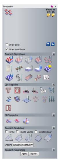
When a **Toolpath** is calculated it will be displayed in this upper area of the **Toolpaths** page. The **Toolpath Names** can be selected for **Toolpath Simulation**, **Toolpath Operations** or to re-opened for editing.
