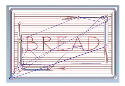
These toolpaths are going to be cut into panels using toolpath panelling.
