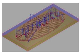
The generated **Toolpath** components are colour coded to assist with both visualisation and identification for postprocessing.
