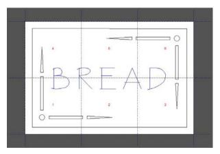
The panels can be seen clearly defined by the dashed lines. If required, the panels can be manually modified by dragging (for example if the panel goes through a feature in the wrong place) details as shown.
