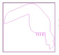
A single closed vector has been generated on the primary colour(s) boundary. **Adjusting the pixel tolerance** will define how close the vector will follow the primary colour boundary.
