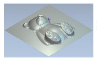
The simulation ends at the final toolpath **Ball Nose 3mm Finishing.**
