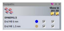
The **Toolpath** appears at the top of the **Toolpaths** page. The **Toolpath** can be shown or hidden by ticking or unticking the relevant **Show in** -2D/3Dcolumn boxes.
