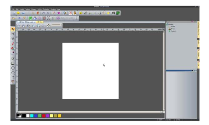
ArtCAM opens up displaying the 2D view, with any Relief and Toolpaths displayed in the 3D View. You can toggle the views by selecting 2D View-Bitmap Layer × 3D View (or F2 or F3 shortcut key).
