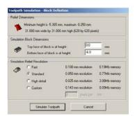
**Relief Dimensions:** shows the overall dimensions of the relief. **Simulation Block Dimensions:** gives the size of the block. This should be at least as big as the minimum and maximum height of the relief plus any height (or depth) of the engraving features.
