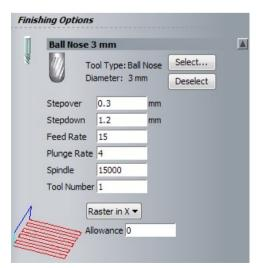
The **default tool parameters** (for Aluminium 3mm Ball Nose) are shown. Changing values in this form do no affect the original tool stored in the database.
