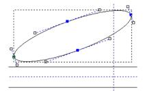
By pressing N on the keyboard on a selected vector, you will switch between Node Editing mode and Select Vectors mode.
