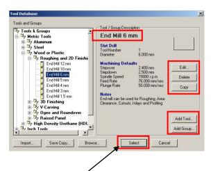
When a tool is **selected** (highlighted) in the left hand window, the tool data and description is displayed on the right-hand side of the form.
