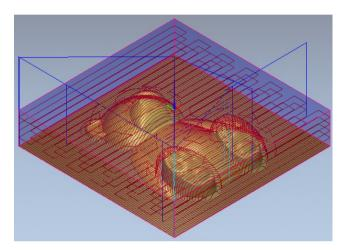
The generated **Toolpath** components are colour coded to assist with both visualisation and identification for **post-processing**.
