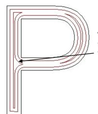
The **Inlay toolpath** has been generated. Note at the **corners** the **toolpath** is **rounded**. This is to ensure that it will be able to accommodate the **Male** insert.
