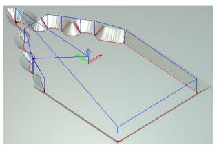
Small V-Bit 12mm 90degree tool With corner sharpening on, the tool will ramp along internal corner intersections to produce the sharpened and completed shape.
