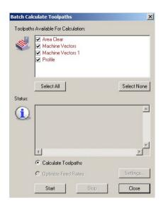
The form appears with all of the **toolpaths** listed. By default all of the toolpaths are ticked, ready to be included in the **Batch Calculate** process.
