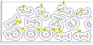
The toolpath ordering form appears and the current ordering is displayed on the toolpath.
