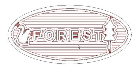
The **2D Area Clearance** toolpaths will appear as shown above. As the primary tool (**End** Mill 6mm) had a default Stepdown value of 2.4mm, all of the machining has been performed at the single depth of -2mm. If the above **Stepdown** value were 1mm then the machining would have been performed at depths of both -1mm and -2mm.
