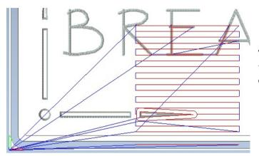
The toolpath is shown in the job with the extended toolmoves from the left corner datum.
