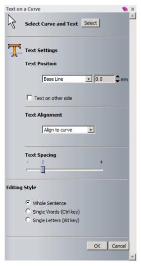
The **Text on a Curve** page appears, which allows you to align an existing **Text Vector** to a **Curve Vector**.
