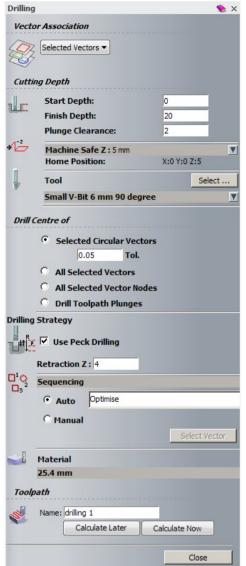
Enter a Start Depth of 0, a Finish Depth of 20mm and a Plunge Clearance of 2mm.
