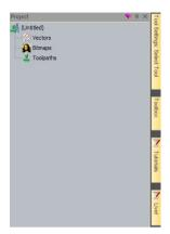
The **Project Panel** serves as a central area to manage the main design and machining aspects of the **ArtCAM model**.
