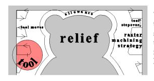
With the **Raster** strategy, the tool moves across the **Z Slices** in parallel, straight line moves separated by the **Stepover** distance. The toolpath is automatically limited away from the relief / Vector by the **tool radius** plus the **Material Allowance**, as shown.
