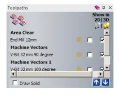
This **ArtCAM** model contains **four Toolpaths**, one of which requires a closed **vector** to control the area to be machined. When a **Template** is **Saved/Created**, all **toolpaths** that exist in the model are included in the output file.
