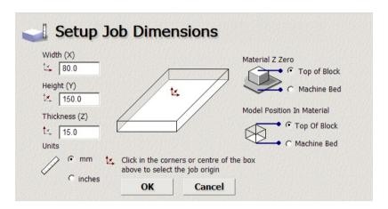
• A **new** ArtCAM Model (sheet) is generated based on the parameters defined above.
