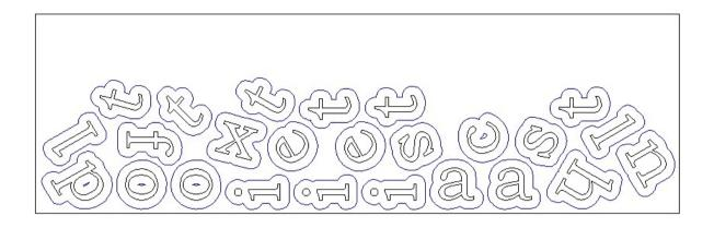
The vector group is machined. The order or machining can be modified to suit either from within the Toolpath or separately from the Toolpaths Tab.
