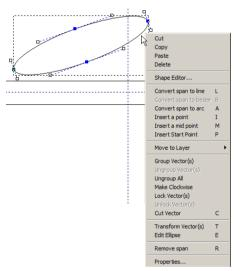
The part of the vector between two node points is called a span. If a span was removed, the vector will become open.
