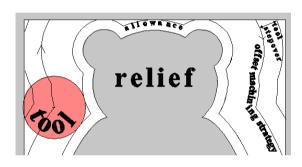
With the **Offset** strategy, the tool moves are offset inwards from the shape of the **Complete Relief** or limiting **Vector**, and outwards from the shape of the **Relief / Vector** contour. Individual tracks are separated by the **Step over** distance.
