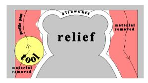
The **Raster** process on its own tends to leave steps around the **Relief**. If required these can be removed by applying a **Profile Pass** either before (**First**) or after (**Last**) the **Raster** moves.
