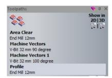
The Unprocessed **toolpaths** are displayed in the Toolpaths Tab. In addition, there are no 'display toolpath' tick boxes below 'Show in 2D/3D' indicating that they have not yet been calculated.
