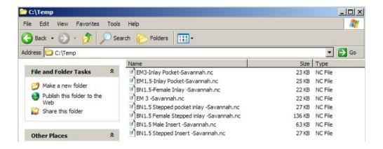
All the **post-processed Toolpaths** have been saved outside **ArtCAM** and translated in the format required for an **Axyz machine controller**. These files can now transferred to the machine controller itself, ready for manufacture.
