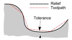
**Tolerance** determines how accurately a cutter path follows the true shape of the **relief**, the actual value being the maximum permissible deviation from the **relief** form.
