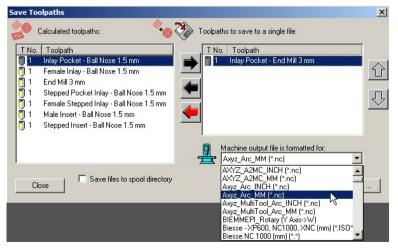
Note: this machine does not support an automatic tool changer hence only Toolpaths that use the same tool can be included in the ncdata output file.
