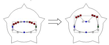
Selecting X on the keyboard edits the selected points with the X coordinate of the last node.
