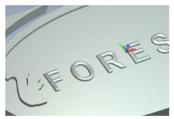
The **1mm chamfer** can clearly be seen on the embossed 2mm high text.
