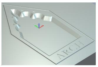
The **outer** limit of the component has been 'scribed' with the 1.5mm Ball Nosed tool.
