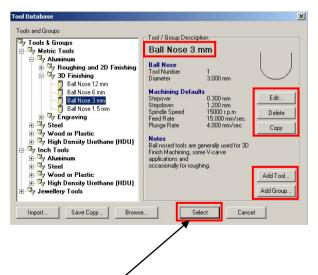
When a tool is **selected** (highlighted) in the left hand window, the tool data and description is displayed on the right-hand side of the form.
