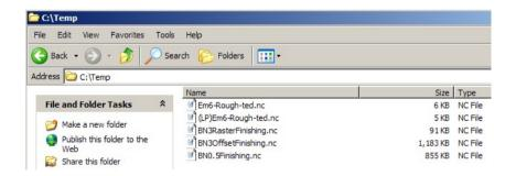
All the **post-processed Toolpaths** have been saved outside **ArtCAM** and translated in the format required for an Axyz machine controller. These files can now transferred to the machine controller itself, ready for manufacture.
