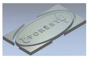
The simulation steps the **2D Profiling** pass down to a total depth of 10mm. If it is required to keep the sign attached to the outer material then **location lugs** (**Bridges**) can be applied retrospectively along the **toolpath**.
