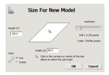
• A **new** ArtCAM Model (sheet) is generated based on the parameters defined above.
