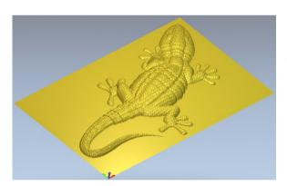
The lizard Relief now has a Maximum **Height** of **35mm**. You can invert it negatively for generating a mould as shown below.
