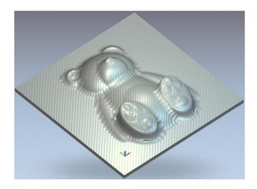
The three toolpaths in the sequence listed are simulated on screen and the final result shown (after finishing operation)
