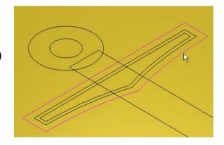
Select a Flat Plane shape with a Start Height of 0.5mm.
