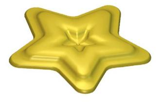
The shape of the **Relief** is controlled by cross sectional, **vector 3** running from the **outer star vector** inwards as well as from the **centre** outwards. The maximum height (5mm) occurs exactly half way between the outer **star vector** and the **centre**.
