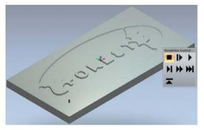
The End Mill 6 mm is simulated.
