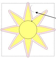
A smooth **Lead In** and **Lead Out** Arc had been added to the toolpath
