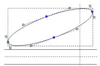
By pressing **N** on the keyboard on a selected vector, you will switch between **Node Editing** mode and **Select Vectors** mode.
