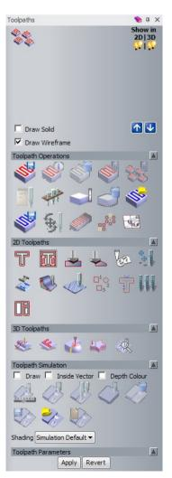
When a **Toolpath** is calculated it will be displayed in this upper area of the **Toolpaths** page. The **Toolpath Names** can be selected for **Toolpath Simulation**, **Toolpath Operations** or to re-opened for editing.
