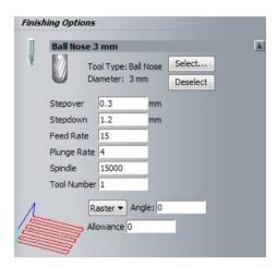
The **default tool parameters** (for Aluminium 3mm Ball Nose) are shown. Changing values in this form do no affect the original tool stored in the database.
