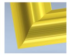
If the option **Move anchor point to other end** was selected, then the **profile vector would be reversed** during the extrusion. The result would then be as shown to the right.
