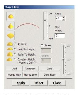
A **Dome shape of 45 degrees** has been created within the selected vectors. The **final height** of the dome was dictated by the defined angle (as No limit was selected)
