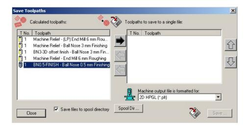
When the **Save Toolpaths** form is opened all existing toolpaths are listed in the **left hand** window. **Toolpaths** are selected and transferred from one side to the other using the central **Arrow** buttons.
