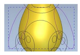
Select a Dome shape, with an Angle of 45 degrees with No Limit and select the Merge High button.
