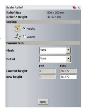
Enter a New Height of 35mm, leave the other Parameters as None and select Apply.
