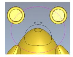
Select a Dome shape with an Angle of 60 degrees with No Limit and select Merge High
