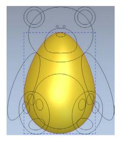
Using the left mouse button, select the outer ears vectors, then hold down the Shift key and select the inner ears vectors.
