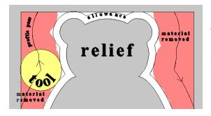
The **Raster** process on its own tends to leave steps around the **Relief**. If required these can be removed by applying a **Profile Pass** either before (**First**) or after (**Last**) the **Raster** moves.
