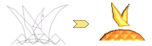
• Use the **outer leaf vectors** and generate a **Merge High Dome Relief** with an **Angle** of **45 degrees**, **Start Height** of **0.4mm** with **Limit to Height** at **1mm**. Select **Close**.
