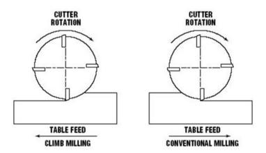
In **Conventional Milling**, the teeth of the tool meet the block of material at the bottom of the block. With this action, the teeth of the tool slide along until sufficient pressure builds up to break through the material surface.
