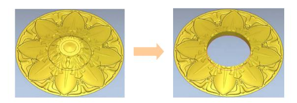
• Select the outer most Circle vector, open the Shape Editor and Add a Plane of Height 20mm to the Relief form.
