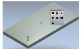
With this option the highlighted tool is drawn (End Mill 6mm first), along with a control panel to control the speed of the simulation.
