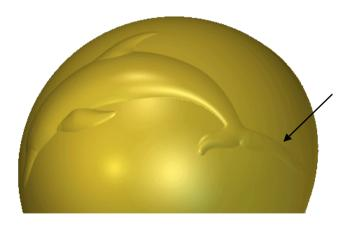
The default option, **project down Z** when applied to a very rounded shape, such as this **Sphere** has caused the resulting relief to be elongated as it is projected onto a steep area. It is especially noticeable on the tail area.
