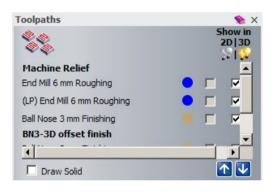
This **ArtCAM** model contains **five Toolpaths**, two of which require closed **vectors** to control the area to be machined. When a **Template** is **Saved/Created**, all **toolpaths** that exist in the model are included in the output file.
