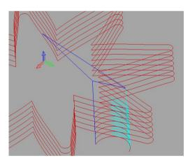
The **light blue moves** on the **toolpath** are **ramping moves** onto the **profile passes**. These only apply to the **Lead In** moves. At the end of the **Lead out** the tool finishes with a **rapid retract** to **Safe Z** followed by a **rapid move** to the **Home Position**.
