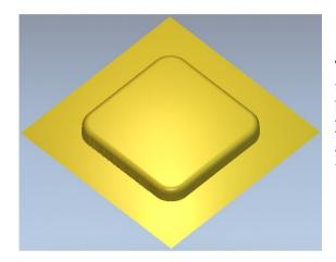
The new **Relief** is automatically assigned to the default **Relief Layer**. A **Relief Layer** can be switched **off** as required by clicking the **light bulb** icon. Any **Relief** operations assigned to a **Relief Layer** that is switched **off** will be temporarily hidden from the model.
