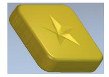
The complete model can be exporting for manufacture. ArtCAM can export a complete assembly as triangulated mesh data (.stl) to another CAD/CAM system or directly to a Rapid Prototyping system.
