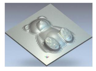
The simulation ends at the final toolpath **Ball Nose 3mm Finishing.**
