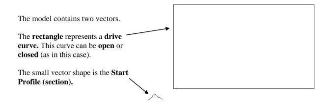
Note: The profile vector is the exact size that is required and can be located anywhere in the **2D View**. Also it must be a **single open vector** (not Grouped).
