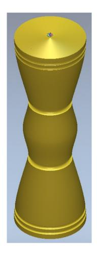
ArtCAM has converted the .3dm surface model and placed it into the Assembly tree.
