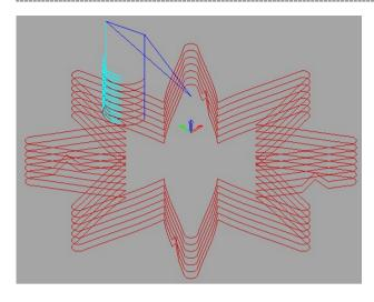
The **4 Bridges** are formed with a triangular movement in the **Z Plane**.
