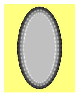
On opening the **Relief**, **ArtCAM** automatically generates both a **Bitmap** (colour) and **Greyscale** representation in the 2D view.
