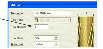
3. The simplest way is to change the tool number by first highlighting the tool in the Toolpaths Tab.
