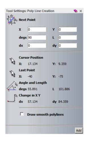
**Polylines** can be generated by entering **absolute co-ordinates** in the **X** and **Y** area, by angles and line length, as **relative co-ordinates** using the **dx** and **dy** (distance from last point) or by clicking with the cursor.
