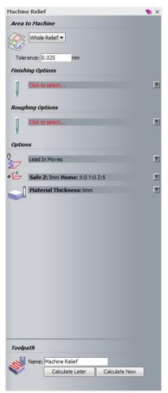
**Area To Machine** – this either applies to the **Composite Relief**, the area within the **Selected Vector** or an **Automatic Boundary**.
