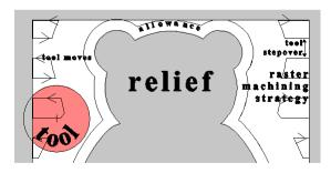
With the **Raster** strategy, the tool moves across the **Z Slices** in parallel, straight line moves separated by the **Stepover** distance. The toolpath is automatically limited away from the relief by the **tool radius** plus the **Material Allowance**, as shown.
