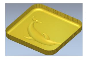
The dolphin has subtracted from the inverted relief, which once assembled to the front (as one half) will result in a positive form.
