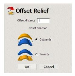
The Offset Relief button allows you to offset the Relief by a certain distance either **inwards** or **outwards**.
