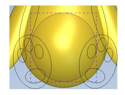
The Relief from the **feet vectors** will be generated using an **angled plane**. This will slope the feet at a specified angle making the toes point forwards and the heels lean back.
