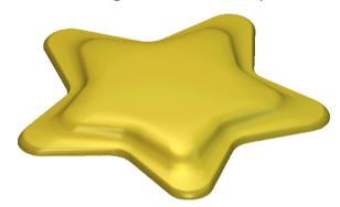
The new **Relief** has been produced as the scaled **vector 2** between the **inner** and **outer vectors**. It then continues at constant height (5mm) across the area inside the **inner vector**.
