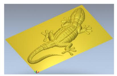
The overall height of this lizard can be reduced by using the **Scale Relief Height** function. The option, **Preserve Detail** if selected will take longer to process but will retain features which otherwise may be erased with a general scaling.
