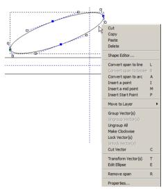
The part of the vector between two node points is called a **span**. If a **span** was removed, the vector will become **open**.
