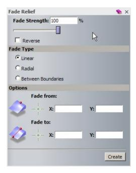
**Fade Strength** can be set anywhere from 1 to 100%, with 100% being faded down to 0 and 50 % down to half the current height in Z.
