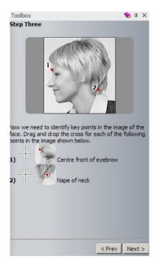
**Step Three** of the **Face Wizard** appears and indicates where to pick the two locating points for this command. This tells **ArtCAM** which way the relief if facing (to the left or right) and also where the main features are.
