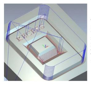
The toolpath is calculated creating 'V' shaped recesses inside or between pairs of selected vectors and text. The maximum depth of the recesses is currently unlimited but the tool does perform an area clearance at incremental depths equal to the specified Tool Stepdown value. The Area Clearance can be removed by inputting a suitably high value for **Stepdown**.
