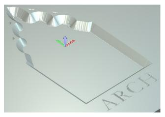
The small features and text have been machined using a single operation with the V-Bit tool.
