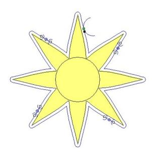
The **four Bridges** are added to the **3D Cut Out toolpath.**
