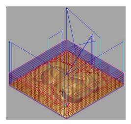
The generated **Toolpath** components are colour coded to assist with both visualisation and identification for **post-processing**.
