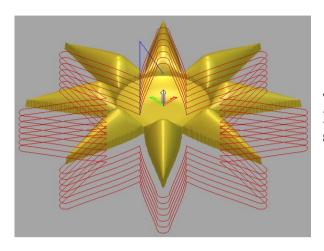
The **toolpath** has been generated at **2mm Z height slices** calculated using the tool **stepdown**.
