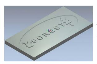
The **End Mill 1.5 mm toolpath** has successfully rest machined the remaining areas inaccessible to the previous cutter and removed the final **0.25mm stock allowance**.
