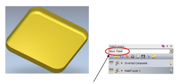
An **inverted copy** of the front composite relief has been created and placed on the **Back Relief**. The Toolbar shows the Back Relief as active, and also creates a new layer called **Inverted Composite**.
