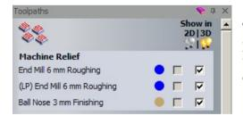
The **Toolpath** appears at the top of the **Toolpaths** page. The **Toolpath** can be shown or hidden by ticking or unticking the relevant **Show in - 3D** column boxes.
