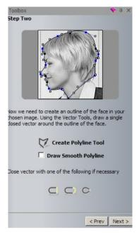
A **Polyline** needs to be created to select the area where the **Relief** is to be generated. A saved polyline can be imported, if required.
