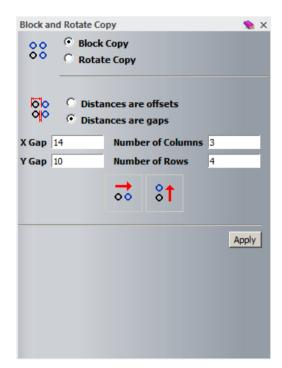
The **Block and Rotate Copy** allows you to create a **block copy** in **X** and **Y** or a **rotated copy** around a point.
