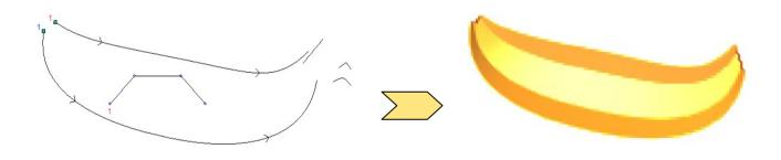
• Generate an Extruded Relief using the line as a Drive Curve, the arch as the first section and the angle as the end section. Select Merge Highest.
