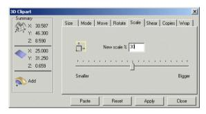
The **Relief** could also be scaled manually by dragging the corner handles of the relief vector, with shift held down to maintain the proportion.
