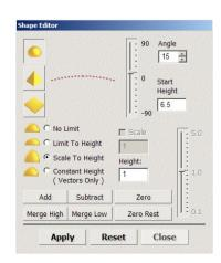
The Start Height value is the actual height from the Z0 of the Relief. By setting the value higher than the leaves, the petal forms are raised above. Using Merge High, the petals are blended into the surrounding Relief.
