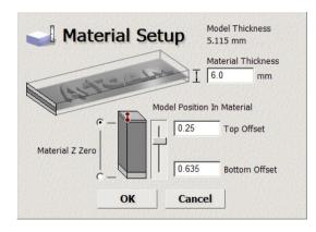
The Material Thickness allows you to input the thickness of the material to be machined. The current relief height is also displayed (5.115). If the Material Thickness is greater than the Relief Thickness, a value for top or bottom offset can be entered.
