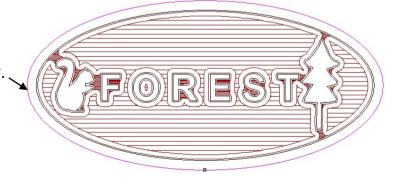
A **2D Profiling** strategy will be used to drive the tool around the outside of the sign.
