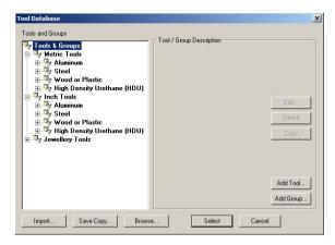
The default **Tool Database** contains a large selection of tools and associated parameters for a variety of materials. The selection can be modified, deleted, or added to by the user as required.
