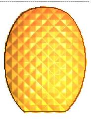
Use the left middle leaf vector and generate an Added Dome Relief with an Angle of 45 degrees, Start Height of 0.1mm with No Limit selected. Select Close.
