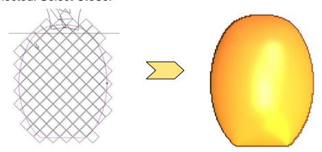
Use the overlapping diamond vector group and generate an Added Pyramid Relief with an Angle of 25 degrees, Start Height of 0 and with No Limit selected. Select Close.
