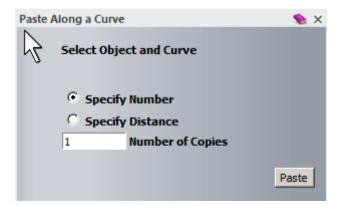
The **vector** is pasted incrementally along the curve either by dividing the curve equally (**Specify Number**), or by a fixed distance, leaving any surplus at the end of the curve (**Specify Distance**).
