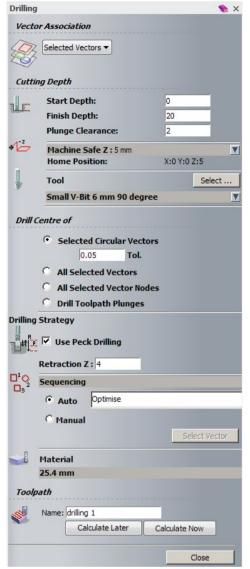
• Enter a Start Depth of 0, a Finish Depth of 20mm and a Plunge Clearance of 2mm.
