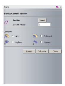
The **Turn** page provides an option for **vector selection** (**Profile**), **Z Scale Factor** for the **Z Height** and **Combine Relief** creation method.
