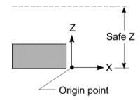
**Safe Z** is the user defined height in Z above the material where the tool can safely perform rapid moves to and from plunge positions.
