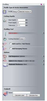
A **Profiling** toolpath can be generated to the defined depth, on the **Inside**, **Outside** or **Along** a closed vector. There is also the option to apply a **Climb Mill** or **Conventional** direction of cut. For an **open vector**, **Inside** will offset the **toolpath** to the **right** of the **vector direction** whereas **Outside** will offset the toolpath to the left of the vector direction.
