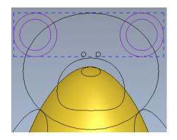
From the Shape Editor form, select a Dome shape with No Limit, an Angle of 45 degrees with a Start Height of 0.5mm followed by Add.
