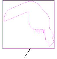
A single closed vector has been generated on the primary colour(s) boundary. **Adjusting the pixel tolerance** will define how close the vector will follow the primary colour boundary.
