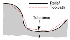
**Tolerance** determines how accurately a cutter path follows the true shape of the **relief**, the actual value being the maximum permissible deviation from the **relief** form.
