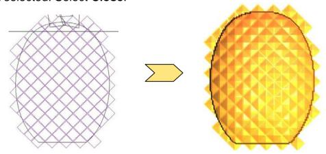
The generated **Relief** goes over the edge of the pineapple. This 'excess' relief can be removed by applying **Zero Rest** in the **Shape Editor.**
