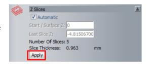
**Start/Surface Z** at **0** (this is the initial height from where the first **Step Down** value will be subtracted).
