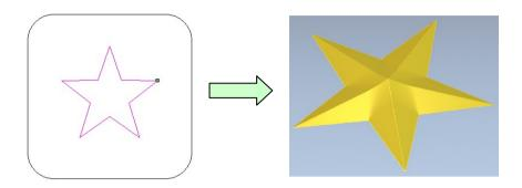
The **Relief Layers Toolbar** allows the **Combine option** (Add, Subtract, Merge High etc) to be changed between layers. This can be achieved by selecting the required option in the icon adjacent to the **Relief Layer name**.
