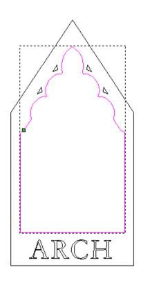
The **Smart Engraving** options provide for finishing of sharp internal corners for the finishing tooplaths using the 'V' **Bit Cutters**.
