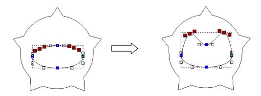
Selecting X on the keyboard edits the selected points with the X coordinate of the last node.
