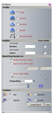
The **3D Blend** assistant page appears providing a comprehensive range of the options. The **3D blend Relief** is either generated from a single vector to a central or user defined point, or across to an inner vector using one of the **Profile** types, displayed in the page.
