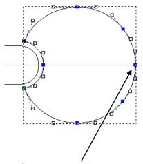
The addition of these extra node points will allow you to move the node point in between the new points and it will only stretch the vector within that region.
