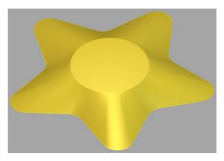
The **Relief** has a **Linear** blend from the **outer** to the **inner vector**. It then continues at constant height (5mm) across the area inside the **inner vector**.
