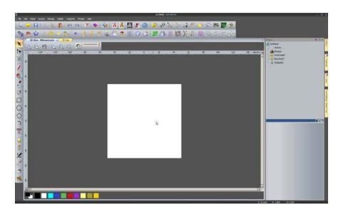
ArtCAM opens up displaying the 2D view, with the Relief displayed in the 3D View. You can toggle the views by selecting 20 View - Bitmap Layer x 30 View (or **F2** or **F3** shortcut key).
