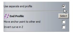
This area of the page enables you to include a **Z** modulation Vector. This controls the **Relief Height** along the **Drive Curve**. As above, this must be selected to reveal the selection options.
