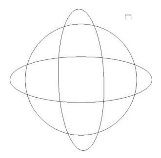
The **overlapping vectors** will be used as the **centrelines** for the **Drive Curve**. The **smaller vector** will be the **Cross Section** of the **Weave** pattern and must be an **Open** vector. The small vector section is actual size of the desired relief.
