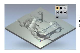
The simulation stops (and retracts) at the end of the second Toolpath (LP) End Mill 6mm Roughing.
