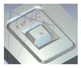
The toolpath has created the same end result, but without performing area clearance at 3mm incremental depths (the tool Stepdown is now 10mm).
