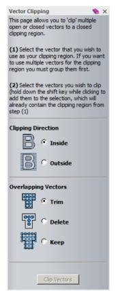
The vector clipping form appears with instruction on how to use the command and the different results available with the options given.
