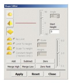
There are 6 options to control how the Relief is combined with the existing ArtCAM model. These comprise Add, Subtract, Merge High, Merge Low, Zero and Zero Rest.
