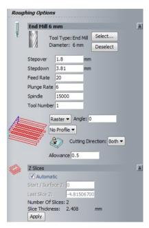
As before, the **Feed Rate**, **Plunge Rate** and **Spindle Speed** are based on the tool manufacturer recommendations but can be adjusted to suit the machine tool, and material used and how rigidly it is clamped down.
