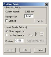
This form allows the guideline to be accurately positioned, deleted or further guides to be inserted.
