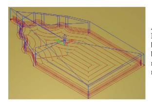
All of the 3 toolpaths created by the Smart Engraving options are displayed and could all be simulated at the same time. It would however be better to simulate them one at a time to see more clearly what each one is actually machining.
