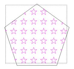
The stars that are whole within the polygon are retained and those that cross the polygon are trimmed back as shown.
