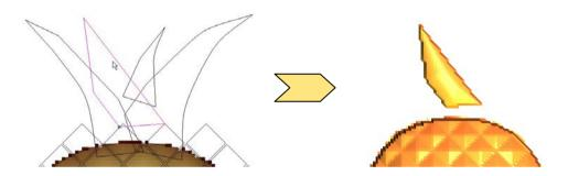
• Use the **right middle leaf vector** and generate a **Merge High Dome Relief** with an **Angle** of **45 degrees**, **Start Height** of **0.2mm** with **No Limit** selected. Select **Close**.
