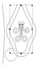
The **vector** outline appears in the **2D View** and the **Paste along a curve** page appears in the **Tool Settings Tab** along with the **3D Clipart** dialog box in the graphics area. The **3D Clipart** box is not used in this case as the **Mode** is already set to **Add**. It must remain open until the **Paste along a curve** process is completed.
