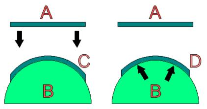
In the above diagram the **vector A** is wrapped onto the **relief B**.
