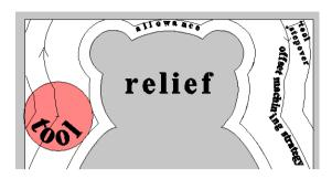
With the **Offset** strategy, the tool moves are offset inwards from the shape of the **Complete Relief** or limiting **Vector**, and outwards from the shape of the **Relief** contour. Individual tracks are separated by the **Step over** distance.
