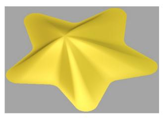
A **smooth blend Relief** is produced with an **offset vector blend** producing an **offset centred star shape**.
