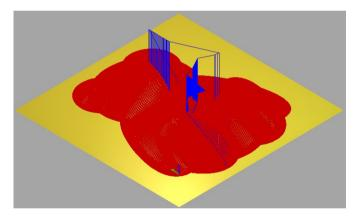
The **3D Offset** with small stepover is displayed. The Selected vector has **limited** the **machining boundary**.
