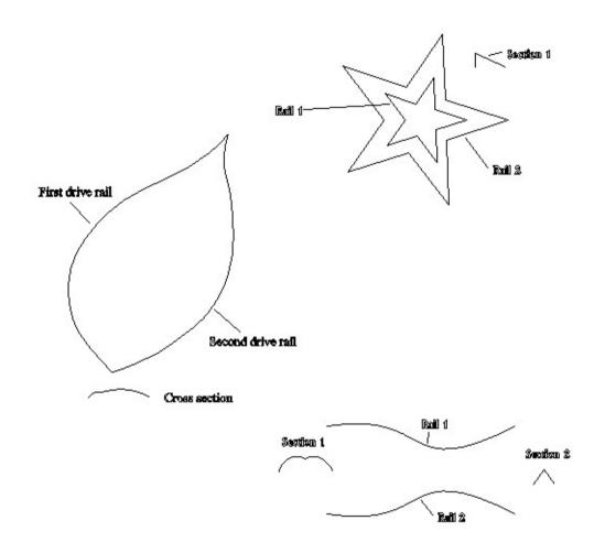
These three examples will introduce the two rail sweep function capability.
