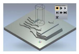
The simulation stops (and retracts) at the end of the first Toolpath **End Mill 6mm Roughing**.
