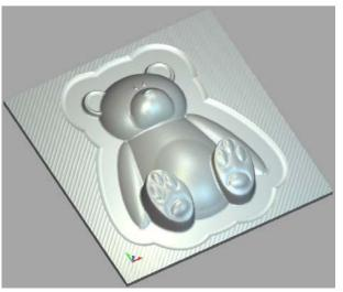
Sharper detail in the corners has been produced by removing previously inaccessible regions to the 3mm Ball Nose tool.
