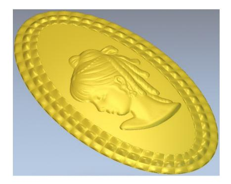
The new **Relief** has been **added** to the original pendant adding an additional height value of **0.5mm** to the model.
