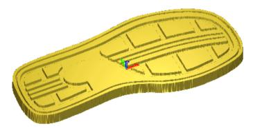
This **shoe sole Relief** was generated from **vectors**, created by opening a picture file. The sole needs to be **faded** to generate a better design.
