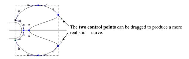
• Select each **control point** and move around as shown in the image below.
