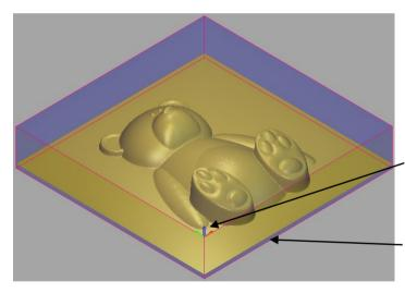
The material is displayed in blue around the **Relief** in the **3D View**.
