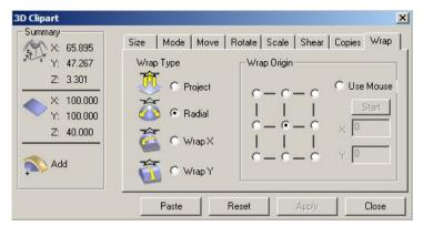
There are four types of Wrapping - **Project** (default), **Radial** (for **Sphere** shapes), **Wrap X** and **Wrap Y**. The **Wrap Origin** can also be set.
