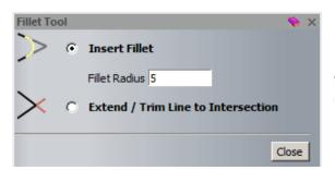
The **Fillet** is generated at a node point or from two Polylines that would intersect.
