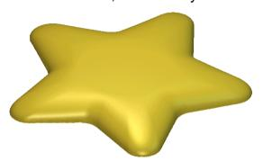
A new **Relief is created** from cross section, **vector 1** scaled between the **inner** and **outer vectors**. It then continues at constant height (5mm) across the area inside the **inner vector**.
