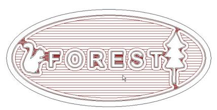
The **2D Area Clearance** toolpaths will appear as shown above. As the primary tool (**End Mill 6mm**) had a default **Stepdown** value of **2.4mm**, all of the machining has been performed at the single depth of **-2mm**. If the above **Stepdown** value were **1mm** then the machining would have been performed at depths of both **-1mm** and **-2mm**.
