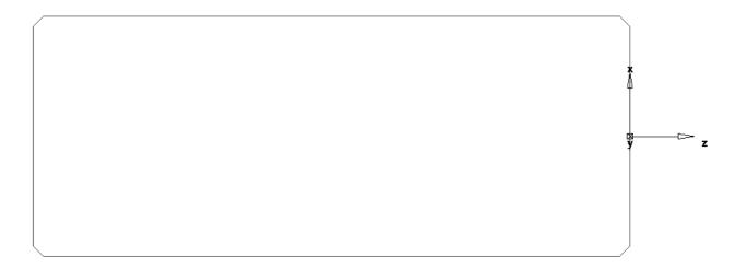
30 We now need to draw a line from 2 points. Snap to the top part of the left hand chamfer. Type in the values as shown. Use the Tab key to move to the next field and type in an Angle of 180 and a length of 0.5mm
