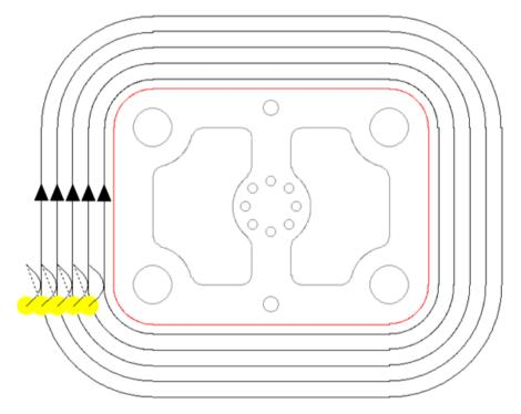
When **Bi-Directional** is selected, the tool does not retract to the Rapid Plane between passes. Instead, the tool completes one pass of the toolpath in one direction, before starting the next pass in the reverse direction:
