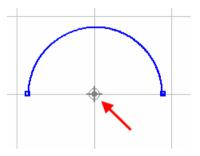
7 Click **Mirror**. PartMaker mirrors the selected geometry using the selected center point:
