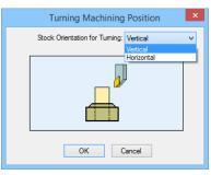
The Turn machining function uses conventional turning tools moving in the X and Z-axes. This machining function includes on centerline drilling where a drill is held stationary while the spindle holding the part rotates. All drilled holes must therefore be on the rotational centerline of the part.
