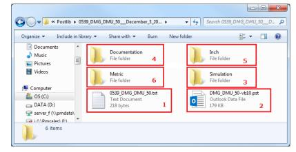
*Tip: If using Advanced and/or Full Machine Simulation, placing the \*.FMS and \*.MCH in the same directory as the \*.PST file will allow your simulation files to open automatically when loading the post processor.*
