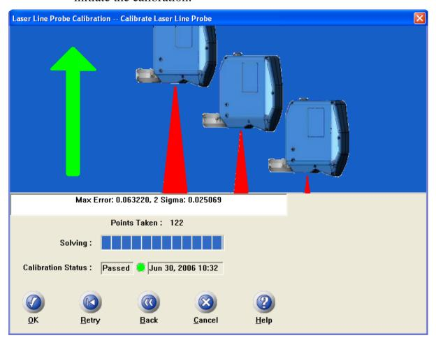
10.If the calibration is successful, the **Calibration Status** shows as **Passed**, and you can click the **OK** button. If the **Calibration Status** is set to **Failed**, click **Retry** to restart the calibration of the plane.
