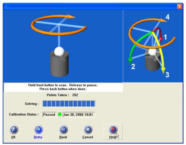
If the **Calibration Status** is set to **Failed**, click the **Retry** button and follow the prompts until the probe has been calibrated.
