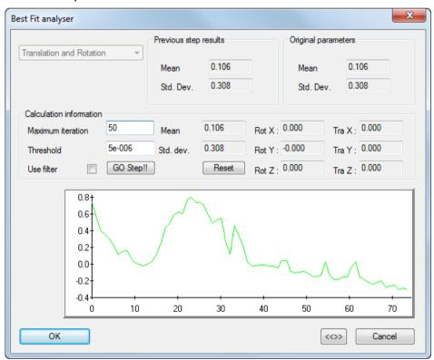
7 Click **Go Step** to calculate the best fit. A graphical representation of the points' deviations is shown. The green line shows the measurement results before the best fit calculation; the red line shows the results after the best fit is applied.
