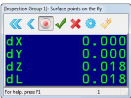
The **dL** value shows the distance from the point to the nominal surface; the **dX**, **dY**, and **dZ** values show the deviations of the measured location from the nominal in the X, Y and Z axes.
