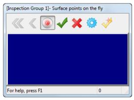
5 Take a point on the irregular sloping surface on the top of the part. PowerINSPECT compares it against the CAD model and updates the dialog, for example:
