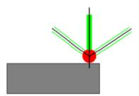
Incorrect orientation of the probe relative to the surface.
