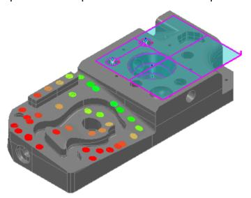
The colour of each spot indicates whether it is within the tolerance specified for the inspection group:
