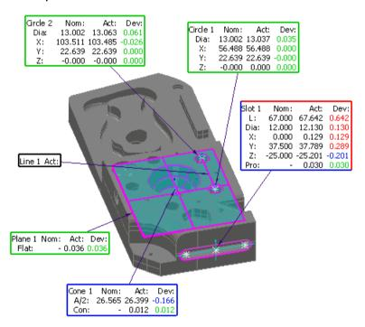
The measurements associated with each item are displayed in labels, together with an arrow that identifies the feature the item refers to. If you have chosen to compare an item's measurements with its nominals, the labels can also display the nominals, and the values are colour coded to indicate each measurement's status:
