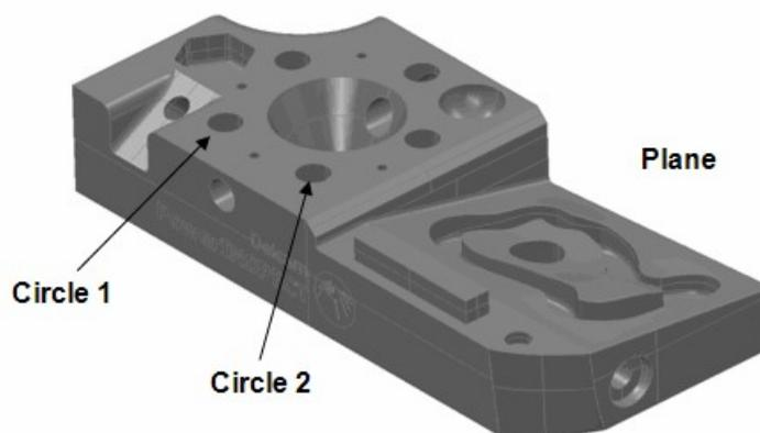
The two circles chosen are indicated, and the plane will be the top flat face. The line will be between the centres of both circles, and the point will be taken from the centre of circle 1.
