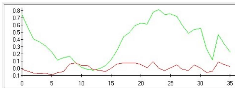
By using the Best Fit, PowerInspect determines the surface profile is correct, and when the calculated translations and rotations are applied, all the measured points are within tolerance.
