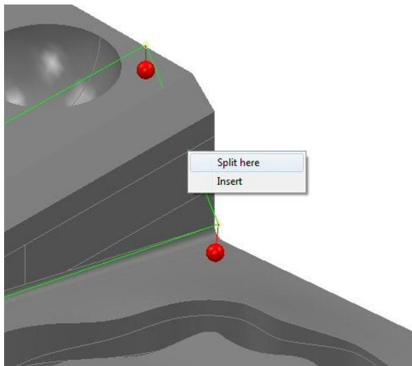
An intermediate point, indicated by a yellow diamond, is on the path mid-way between the probe points.
