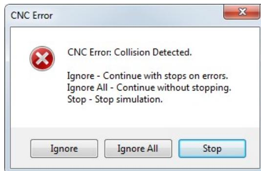
This warning is produced as the connecting move between the last point of the probed cone and the first point of the plane results in a collision between the probe and work piece. You can rectify this by inserting an intermediate path between the cone and plane features.
