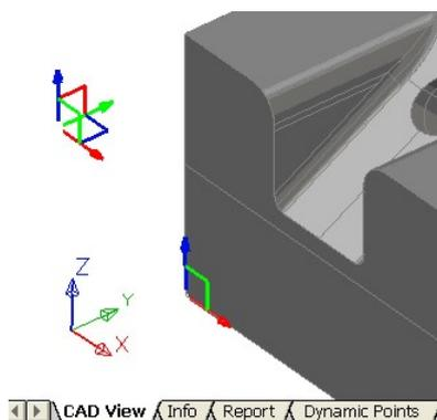
In addition to the datums, a graphical representation of the coordinate system of the active alignment (the PCS Datum, by default) is displayed at bottom left of the CAD view. It allows you to identify the axes of the active alignment when the active alignment is not visible on screen.
