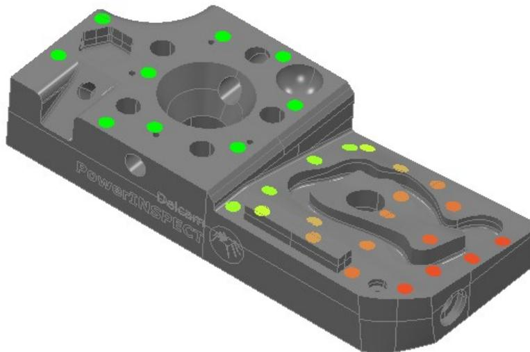
The example shows the surface used for the alignment, Plane 1, is within tolerance. However, the other top surface is out-of-tolerance towards the other end of the block. We can attempt to improve the alignment by creating a Best Fit item that includes the results of the inspection group.
