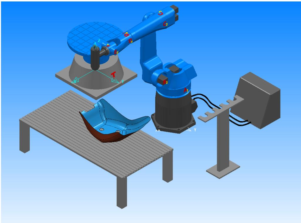
Create and perform a simulation on the **Holes (original)** toolpath. The simulation works perfectly, but we will modify the head orientation for each hole, in order to put the robot wrist in the middle of the part.
