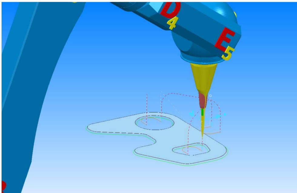
Make sure that the **Lock graphics display** is unticked and click on the **play** button. The robot will move along the toolpath.
