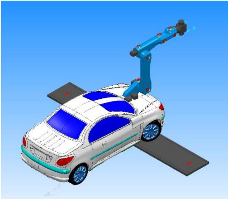
As we can see, the robot is not positioned correctly. In the **Robots** tab, select the **Center Right (Rail)** origin. Select an ISO 4 view (Ctrl + 7).
