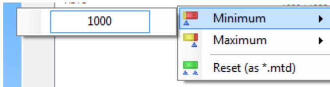
The motion range of the Y axis is now limited from 1 000 to 1 200 mm. To reset the values, select the **Reset (as \*.mtd)** option.
