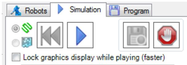
Tick the **Lock graphics display** option and click on **Play**. The simulation will be recorded into the RobFile. The **Lock graphics display** option allows saving time (The calculation will be 100 times faster). After the simulation, click the **Stop recording** button.
