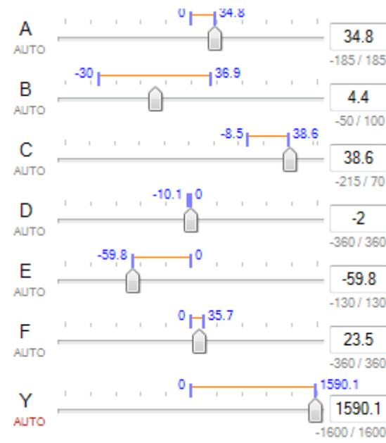
It is possible to apply additional constraints on an axis. Right click on the **-1600/1600** on the Y axis. In the menu, select and apply the value of 1200 for the maximum value and 1000 for the minimum value. Use the Enter key after entering the values.
