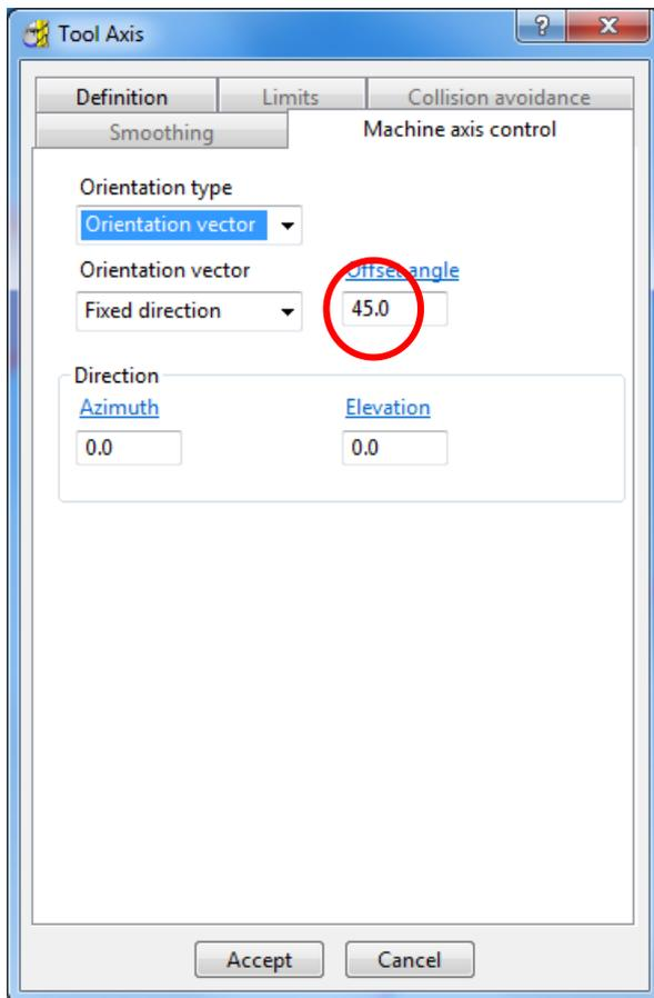
Select an **Orientation vector** orientation type and a **Fixed direction**. Add an **offset angle** of 45 deg in order to change the head orientation.
