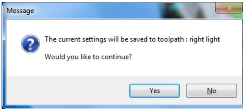
Say **Yes**. The robot position is saved as user parameters in the current toolpath. In the explorer, right click on the **Right Light** toolpath and select **Settings...** and **User defined settings**. The values are stored here:
