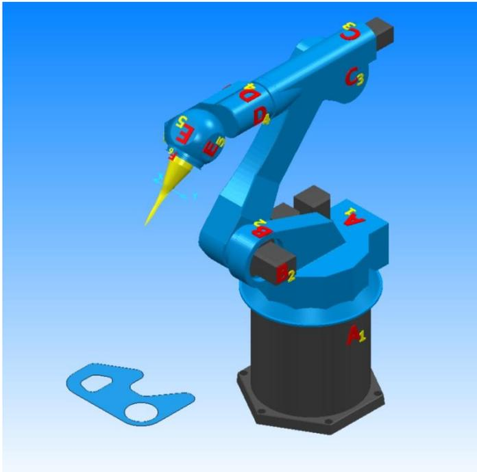
Select and activate the Milling toolpath. Then, select the **Attach a tool to start** button in the **Simulation** tab. The robot will move on the starting point on the selected toolpath:
