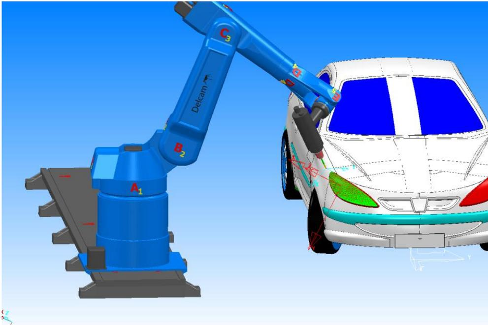
Click again on the **Attach tool to start** button. The robot is moved to a beginning position near as possible from the previous one. Play the simulation. The robot is now able to perform all the milling toolpath without singularities.
