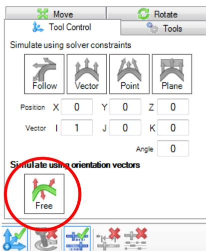
We will add orientation constraints in order to force the knife to follow the tool path. Select the **Follow** option and perform a simulation:
