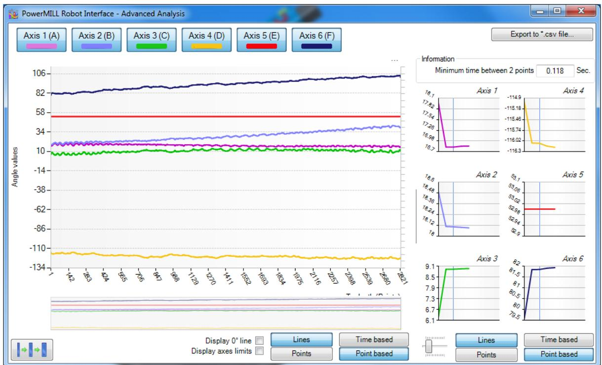
It shows the evolution of axis values against the point's number. To change this, the **Time based** / **Point based** buttons can be used to draw the information against the time or against the points numbers.
