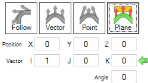
**Plane:** Keep the head perpendicular to a plane (What is the difference between the “vector” orientation and this one?)
