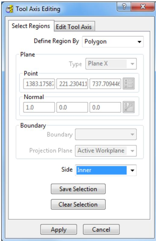
The first step consists in selecting the area to modify. Select Define region by **Polygon** and click on the main view to create a polygon around the top right hole:
