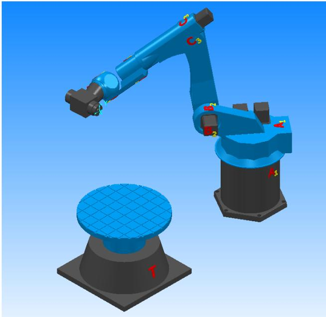
The default origin is wrong (the part is inside the robot base). To put the part on the rotary table, select the **Center Table** origin in the Robots tab:
