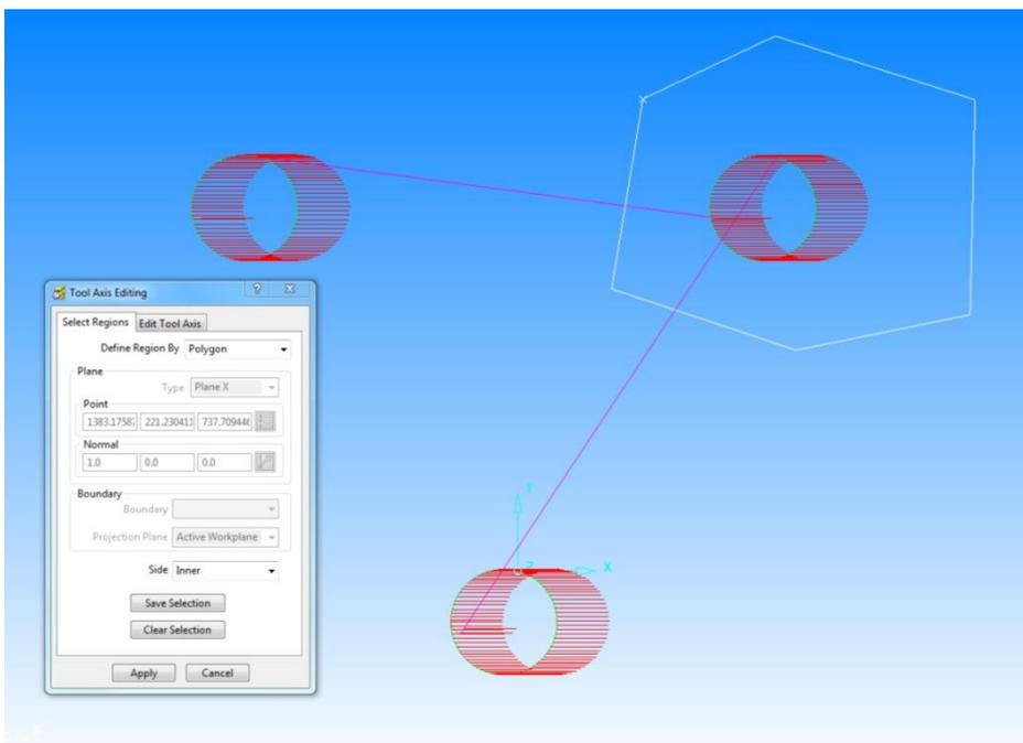
Select the **Edit Tool Axis** tab and select the **Tool Axis** button,
