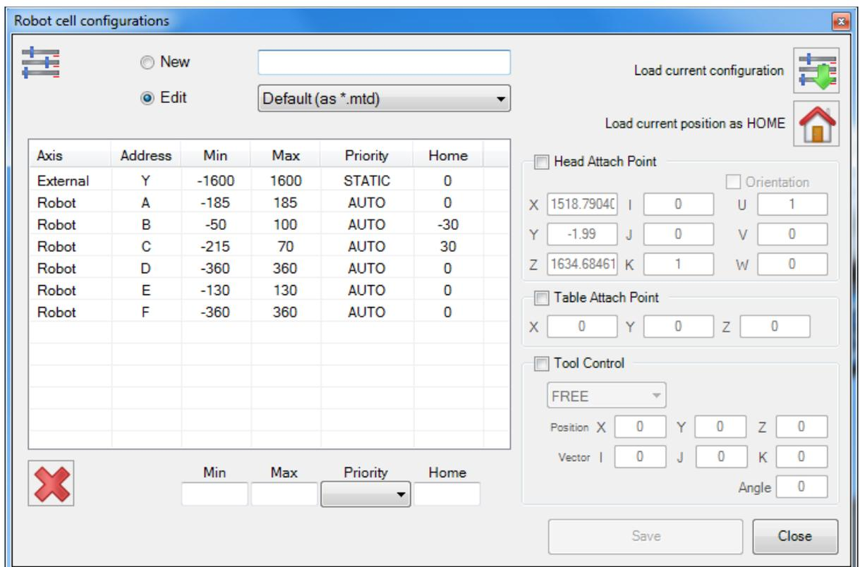
Select the **New** option and type **LowRailPriority** as a name. Select the Y line in the table and change the priority to **Low**, then click the **Save** button. Rename the **LowRailPriority** into **LowRailMotionRange** and modify the **Min** and **Max** values to 1000 and 1200. Restore the axis priority to **AUTO**. Click **Save** and **Close** the dialog.
