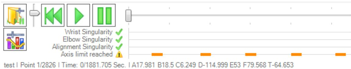
This tool shows information about the singularities and the axis limits. In this example, no singularities are detected and some axis limits are reached. To add more information, open the
