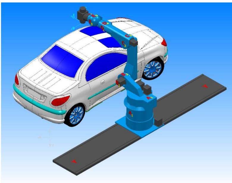
Select and activate the **Back window 3+2** toolpath (in the **Milling** folder), then create and record a simulation. As you can see, the motion range of the Y axis rail is wide. We'll see how to fix that.
