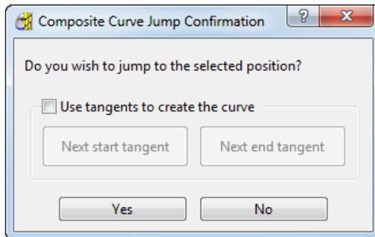
Deselecting the **Use tangents to create the curve** option joins the curve with a straight line.
