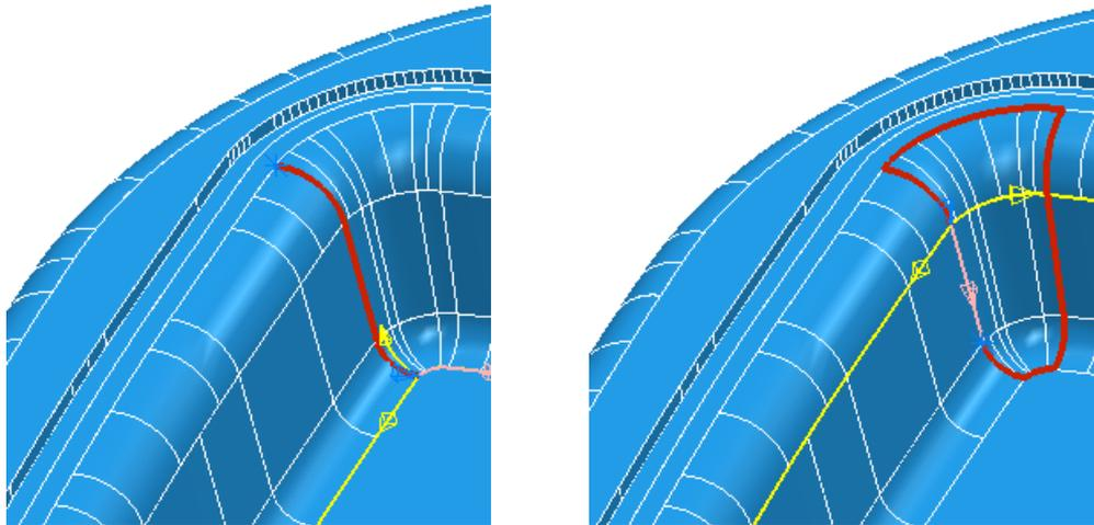
**Gap jumping multiplier** — Enter a value to determine if PowerMILL can automatically jump the gap. This value is multiplied by the **Closure tolerance** to give an actual value. If the gap is larger than this value the **Composite Curve Jump Confirmation** dialog is displayed. If the gap is smaller than this value PowerMILL works as if there is no gap (see page 15).
