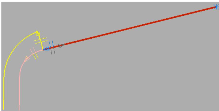
If you select the surface around ②, the composite curve looks the same, but the curve used to create the composite curve is the surface edge of the vertical face.
