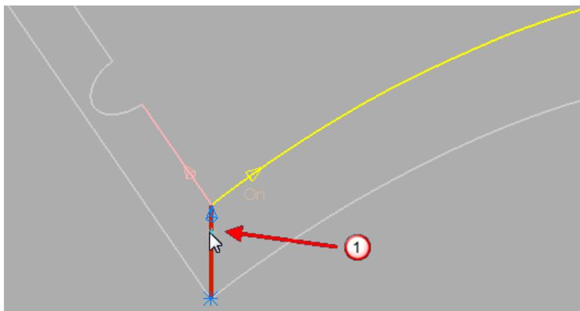
Selecting the curve at point ②, gives a forward direction of downwards.
