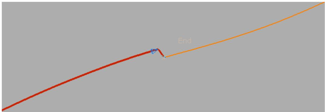
Selecting the **Use tangents to create the curve** option joins the curves with a tangential curve.
