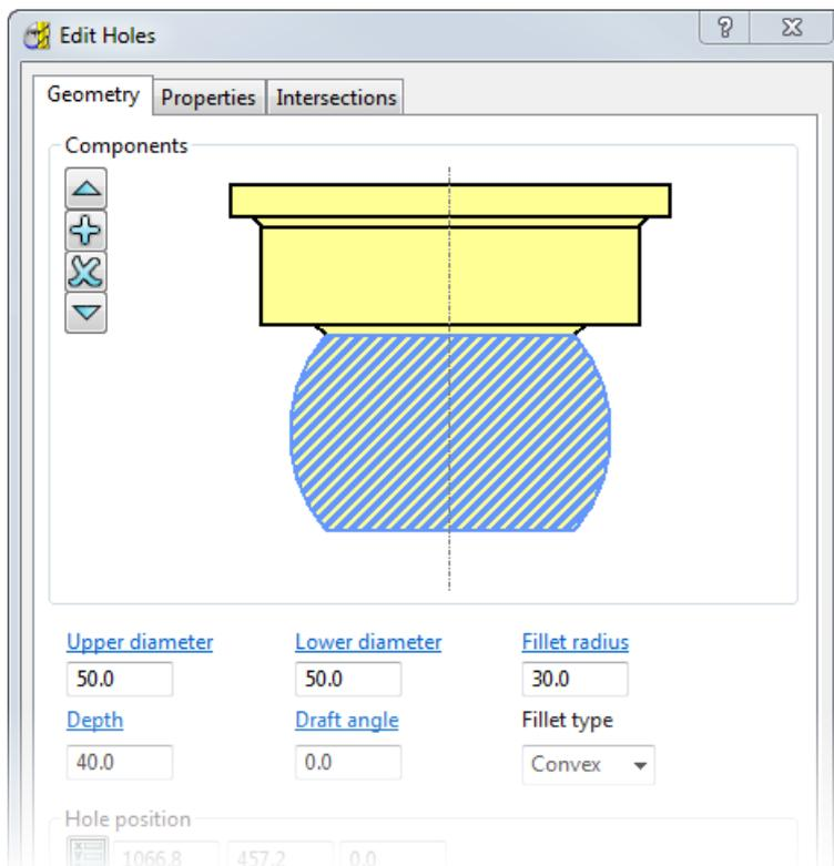
**Hole position** — Enter the x, y, z coordinates of the centre of the hole.
