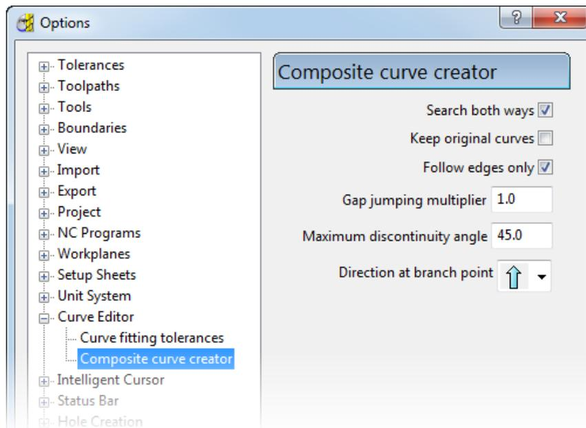
**Search both ways** — When selected, the **Composite Curve Creator** searches both ends of the curve to find adjacent segments. When deselected, the composite curve creator searches only the current curve to find adjacent segments.
