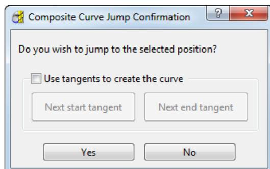
**Use tangents to create the curve** — When deselected, joins the curves with a straight line. When selected, joins the curves with a tangential curve.
