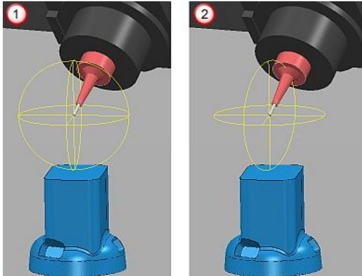
When you hover the cursor over a drag-handle, the drag-handle is highlighted. You can then drag the machine tool into a new position.
