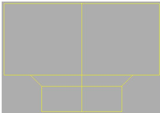
Selecting a **Top component** of 2 and a **Bottom component** of 3 or **Last** produces a toolpath on the bottom two components.
