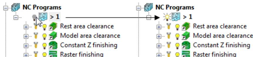
Drawing a toolpath, which is in an undrawn NC program, automatically draws the NC program, so the toolpath is displayed.
