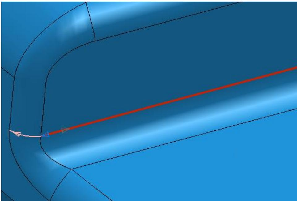
This is the same as **Straight**
