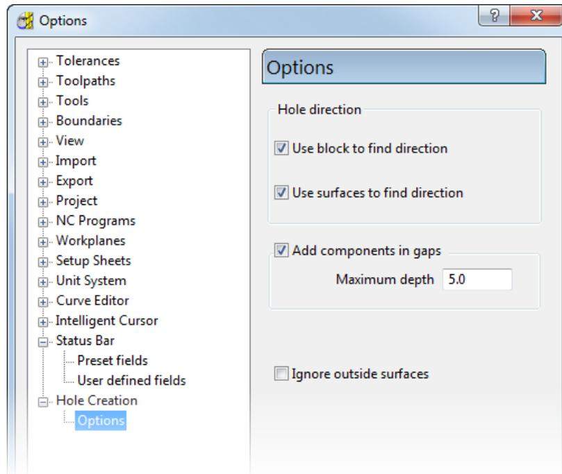
**Use block to find direction** — Select to use the block to determine the direction of holes. When selected, holes point towards the block centre.
