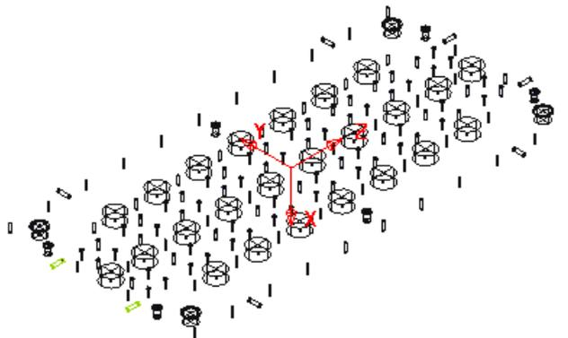
**Find holes in both directions** — When **Group by hole axis** is selected, places holes from both directions into a single multi-axis feature set. When **Group by hole axis** is deselected, splits the holes into two feature sets (one for up and one for down).
