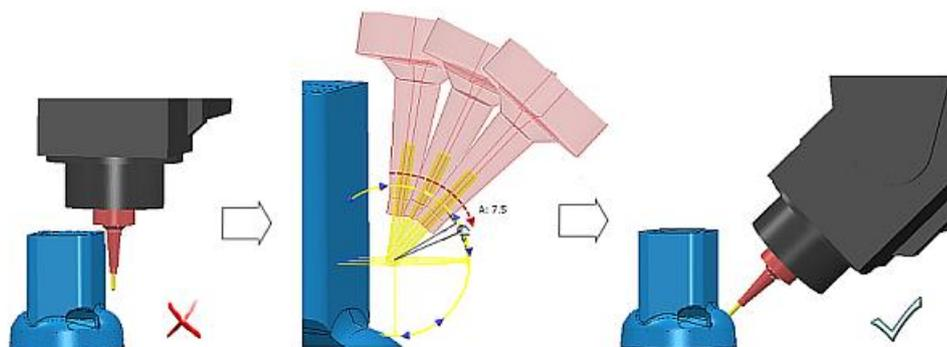
In this graphic, access to the workpiece is improved by rotating the grab-handle to adjust the machine tool's configuration and tool axis.
