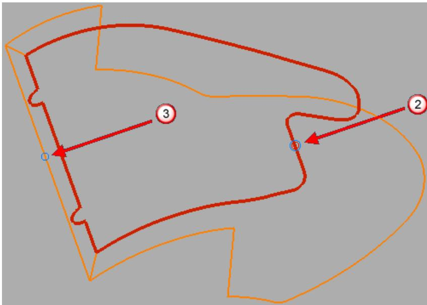
② The first marker point shows the start and end point of the closed composite curve.
