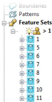
Selecting **Combine Holes** converts the individual hole components, which share a Z axis, to a compound hole.
