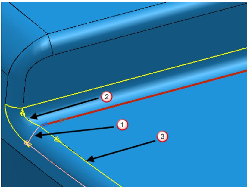
**Direction at branch point** — Select the default direction displayed on the **Create Composite Curve** mode toolbar (see page 12).
