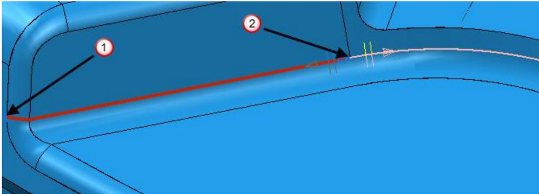
In this case, the composite curve extends as far as point ①. Because the angle at the branch point is greater than the discontinuity angle, the composite curve creator extends the curve from the other end (point ②).
