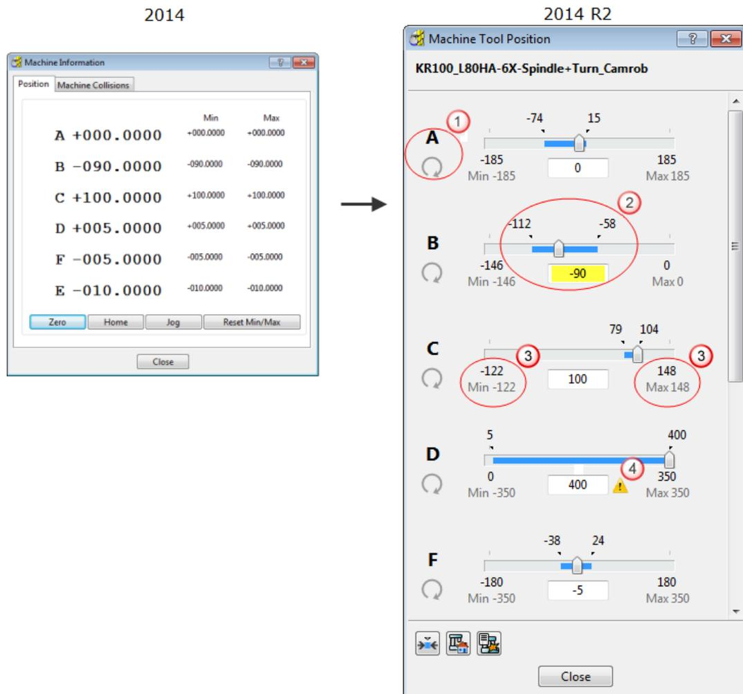
① The axis address (**A**) and the icon indicates the axis and the axis type.
