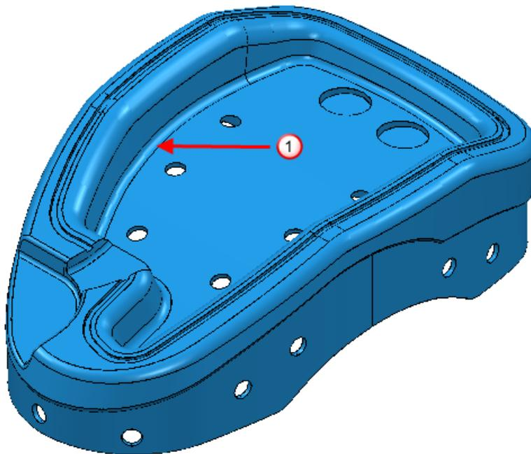
PowerMILL creates a composite curve using the default options. The resulting curve is highlighted.
