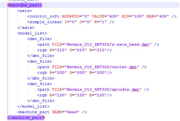
You can use different colours for each part, but can't use different OPACITY. OPACITY are applied for all parts in one <model\_list>.
