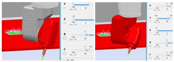
When a collision occurs, the colliding parts of machine are coloured and a warning message is displayed:
