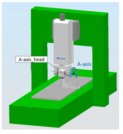
The arrow shows the part of the machine where the A axis component is attached. The A axis component rotates around a centre point of this part so in PowerSHAPE we isolate this part.
