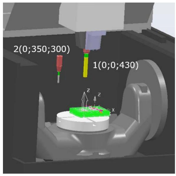
Point number one indicates the position of the head\_attach\_point. Point number two indicates the position of the tool\_change.
