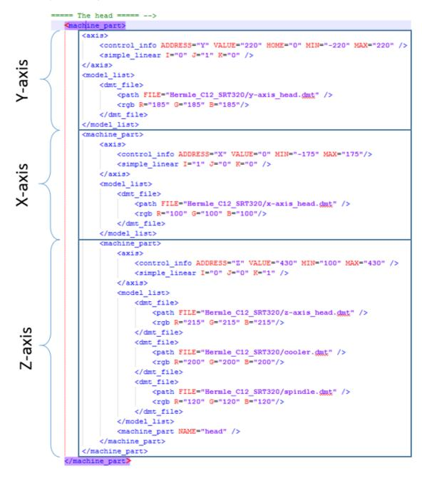
This Hermle machine tool has: Centre of table: X=0; Y=0; Z=0. Centre of spindle: X=0; Y=220; Z=430.
