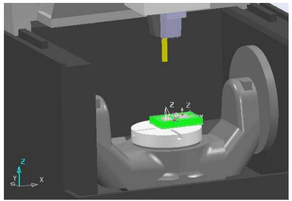
If you change the direction of the vectors in line head\_attach\_point for this machine, I="0" J="0" K="1" on I="1" J="0" K="0" then this gives:
