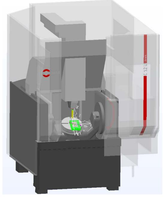
Now you can move on to creating the <machine\_part> definitions. As mentioned before, there are two <machine\_part> definitions: one for the head of the machine and one for the table. This example defines a machine tool that has a Table-Table configuration.
