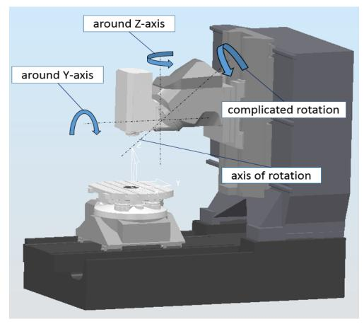
Such rotation is called the complicated, because consists of two rotational movements (around Z-axis and around Y-axis).
