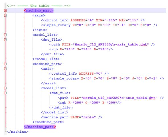
The a-axis\_table is the primary (or parent) component for the table assembly. Therefore, before you close the a-axis machine\_part, open a new machine\_part for the c-axis\_table component.
