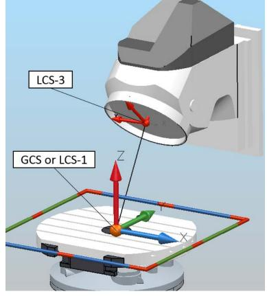
Then, additionally create local coordinate system (LCS-3) at the point **A**, oriented perpendicular created arc (Z-axis should be perpendicular created arc). See below:
