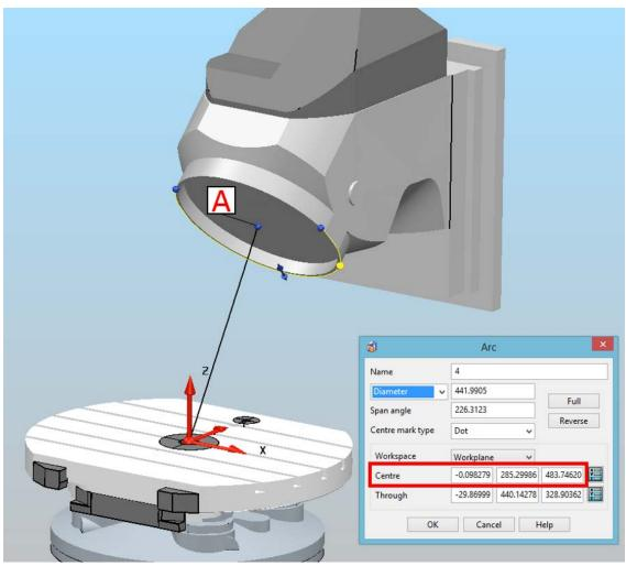
Let us create new local coordinate system (LCS-1) in the centre of table X=0 Y=0 Z=0. We then create some simple arc where we can note the exact location of the centre of rotation:
