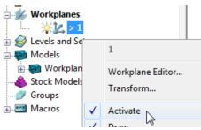
The next step will be to rotate the new **Active** - **Workplane** - **1** to re-orientate the model such that the longer side is aligned to the **X-Axis**.
