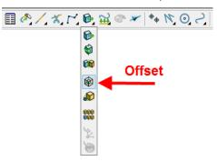
3 In the **Offset** toolbar, select the **3D Smooth** button, input a **Distance** of 1 and then press the **Return** key.
