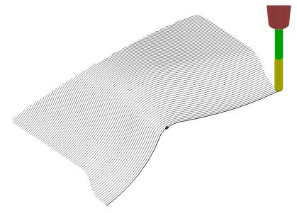
Leads and Links are not displayed to provide a clearer view of the toolpath.
