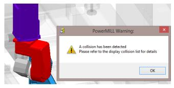
After several passes the machine tool head is in collision with the component. The machine tool head changes colour to **red** and a **PowerMILL Warning** box appears as soon as the first collision is detected.
