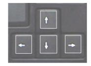
11 On the keyboard hold while holding down the Shift key, press the left hand Arrow key to perform continuous, incremental -ve X moves on the machine tool model.
