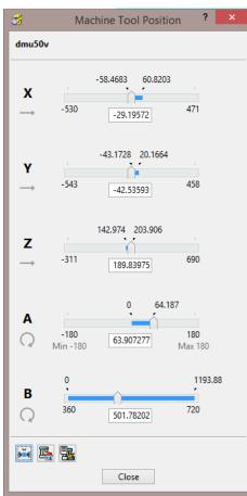
The current positional values are displayed in the **Machine Tool Position** dialog.
