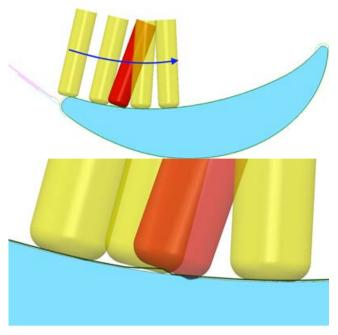
If you enter a **Model defect tolerance** that is greater than the defect size (for example, **0.5** mm), PowerMILL ignores the defect and produces a smooth toolpath:
