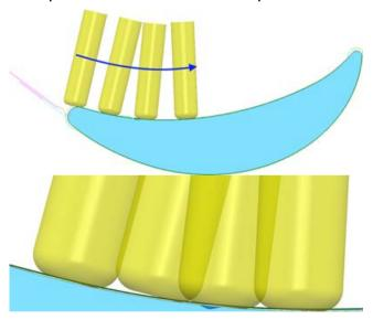
**Tolerance** — Enter a value to determine how accurately the toolpath follows the contours of the model.
