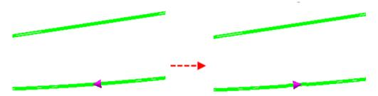
Reverse side to machine —Toggles the side of the curve that is machined. For example, click to toggle the creation of toolpaths from the area between the two curves, to the area outside the two curves. A tool is displayed to indicate which side of the curves is machined.
