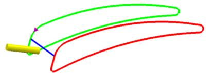
Change cut direction —Changes the cut direction from conventional to climb milling or from climb to conventional milling.
