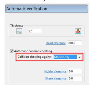
The **Model Only** option is usually faster to calculate than the **Model** and **Stock** option. However, this option does not check for collisions between the tool holder and the stock so take care when running these toolpaths.
