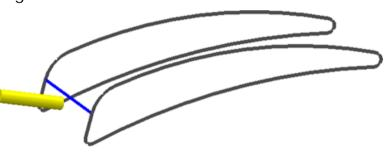
To minimise the likelihood of leaving a dwell mark on the machined component, the seam curve should be located by the leading or trailing edge of the blade.
