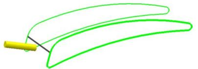
Select end curve — Select a closed curve where you want the machining to end.
