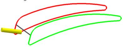
Select seam curve — Select an open curve that joins the start and end curves. This curve defines the start point of each toolpath segment and must connect to the start and end curves.
