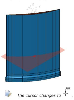
3 Click on the model to define a point which the slicing plane passes through. The orientation is determined using the principal editing plane of the active workplane. The coordinates of the curve are displayed in the **Origin** area of the **Planar Section** dialog.
