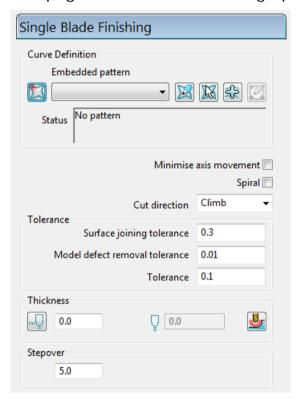
**Curve definition** specifies the curves bounding the area you want to machine and adds the machining properties to those curves. The pattern must contain two or more curve segments.
