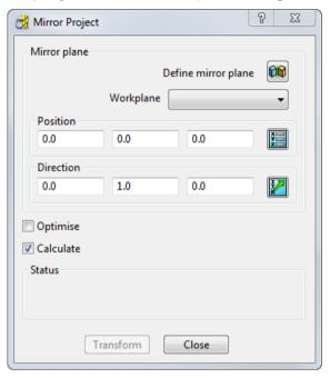
2 Select a workplane from the list. This represents the coordinate system that you want to mirror the project along. In this example, select 2 from the **Workplane** list.
