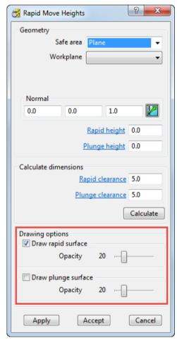
**Draw rapid surface** — Select to draw the surface of the safe area. Use the slider to set the level of opacity of the rapid surface.
