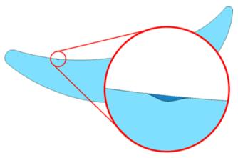
If **Model defect tolerance** is set to **0.01** mm (default) PowerMILL generates a toolpaths where the tool tip rolls into the defect. The tool axis wobbles, which results in an unacceptable machine motion:
