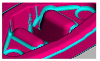
This compares the previous finishing toolpath which left some material in the corners.
