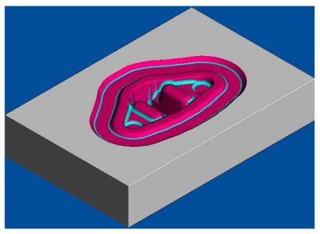
6 Zoom into the machined areas to view the cleaning up of the non-tangential surfaces.
