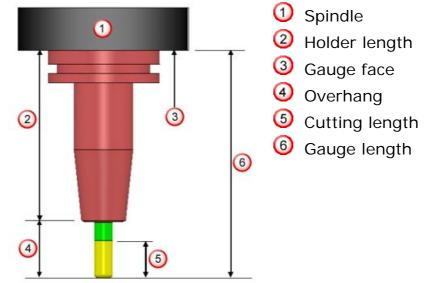
The **Cutting length** represents the part of the cutter that removes material. This is the **Tip length**.
