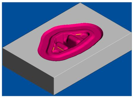
6 Zoom into the unmachined areas. You can see that some of the corners need cleaning up, particularly between non-tangential surfaces.
