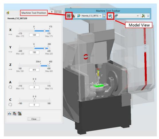
Use the **Machine Tool Position** dialog to check the direction of movement is correct.
