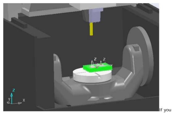
change the direction of the vectors in the head\_attach\_point line for this machine, I="0" J="0" K="1" on I="1" J="0" K="0" this gives:
