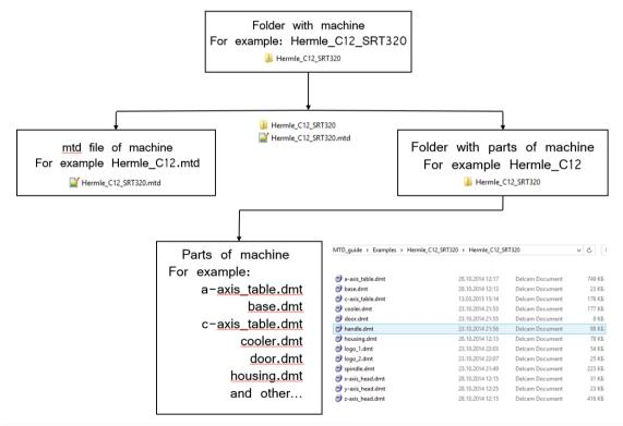
You can include all static parts on one <machine\_part>:
