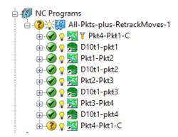
This can be fixed by using different positional move toolpaths at the ends of the **NC Program** that will start well within the main machining areas and then re-track the tool back to the original start position.
