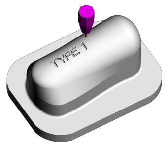
The text **`TYPE 1**' is machined to a total depth of **-3** with the tool aligned to the *Surface Normals*.
