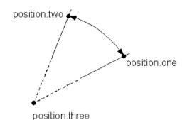
A radial dimension has a text position (*position.text*), *position.one*, *position.two* and *position.three*.
