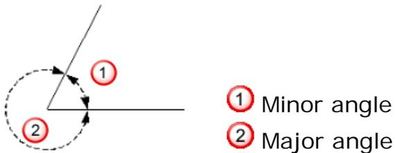
The intersection position of the two lines defines the pivot of the angle.
