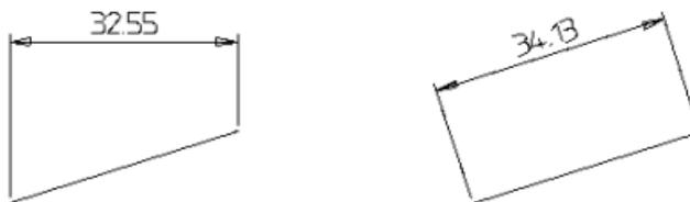
A linear dimension measures the length of a line or the distance between two points.
