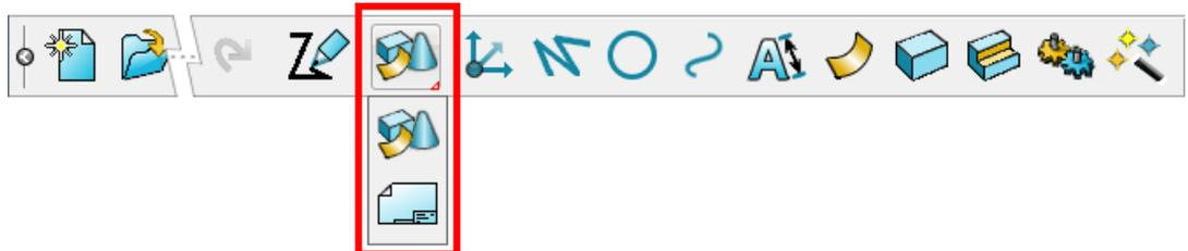
The **Drawing Selector** dialog is displayed where you select an existing drawing or create a new drawing. The **Drafting** toolbar is also displayed.
