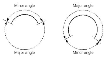
When you hover the mouse over an arc, both the minor and major angles are displayed, where the type not required is in brackets.
