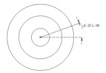
It is not necessary to select the centre of the arc directly.
