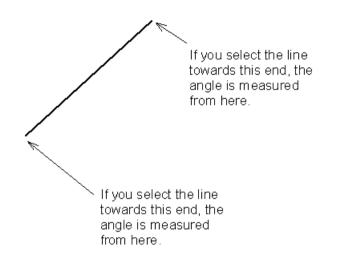
If the top end of the line is selected, the angle is measured from the top part of the line. As you move the mouse cursor, the rubber-banded angle moves too.
