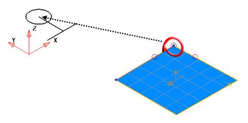
The example below shows the corner point dragged and snapped to the circle centre.
