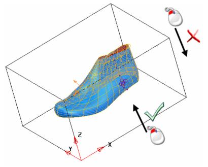
When a bounding box is created, the Arm cursor is only displayed if it is within the bounding box. You can only define points within the bounding box. If you try to define a point that is outside the bounding box, it is not registered.
