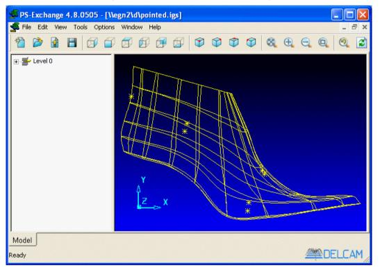
In order to import the file into PowerSHAPE you must first export it in **Delcam Exchange**. The file type you export to is automatically selected by **Delcam Exchange**.
