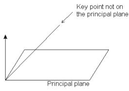
then the new position is projected onto the principal plane.
