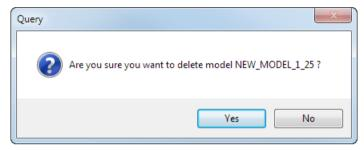
Click **Yes** to remove the model from the database and return to the **Delete Model** dialog. If the **Use Recycle Bin** option is selected on the **Model** page of the **Options** dialog, the model is sent to the Recycle Bin (providing the bin is not full). Otherwise, the model is permanently removed from the system.
