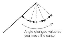
Use this rubber-banded angle as a guide to determine the angle you want to measure.
