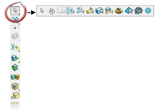
Access a flyout toolbar using a flyout button. Flyout buttons have a small triangle icon in the bottom right corner. There are two types of flyout buttons:
