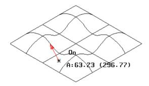
By default, only draft angles of positions on the surface curves are measured. You can measure the draft angle of positions within a surface patch by holding down the **Shift** key. The draft angle is measured from the principle plane to the normal of the point on the surface under the cursor.
