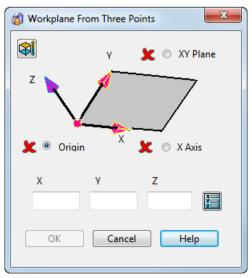
If you do not wish to define a workplane at this point select Cancel on the dialog. You can define a workplane later, if required, by selecting Workplane from three points option (Workplane menu).
