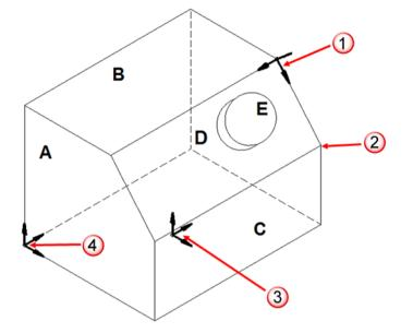
U Local coordinate system (Workplane). Convenient for:
