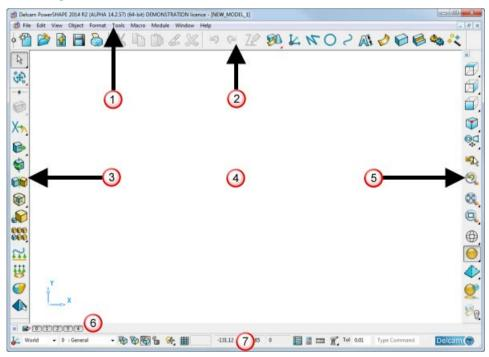
PowerSHAPE uses a Windows-style interface with menus and toolbars. The areas of the screen are identified as follows:
