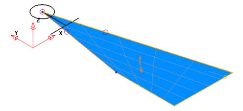
The example below shows the corner point dragged to the circle centre, but using the  $\mathbf{X}$  key to lock the X axis.
