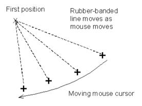
2 Use the rubber-banded line to enter the second position. A rubber-banded angle is displayed, shown in the image below.
