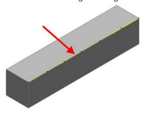
4 Click on a point and use the curve handles to change the shape of the curve. The distortion is applied so that the points on the original curve are moved to the corresponding point on the edited curve and the model is distorted in a similar way. The graphics will update when the curve handles are released. The original model is displayed in wireframe and the distorted model in shaded graphics.
