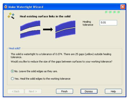
**Healing tolerance** - Enter a value to change the number of gaps outside the healing tolerance. The default value is the working tolerance.
