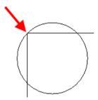
**Default Hole Definition** - Creates a default plain hole, based on the current height of the pocket.
