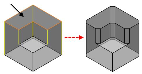
**Variable** — This option is only available once you have clicked **Apply** to create a chamfer (see page 217). If you have only selected the path, but not created the chamfer, you can select the **Advanced** button to create a variable distance chamfer (see page 215).
