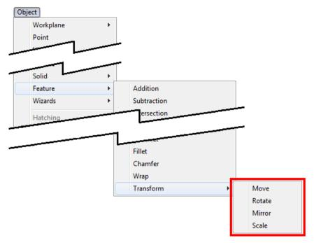
The following specific dialogs are displayed when using this method to create the transform feature:
