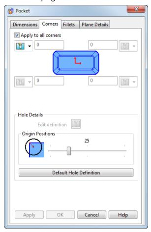
**Edit definition** - Click on to make changes to the size and type of hole using the **Hole** dialog.
