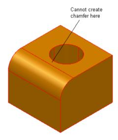
This option will allow you to create the chamfer onto the continuous surfaces.
