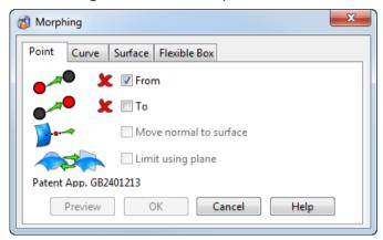
When you create the morph, the bulge that is produced by the distortion is centred on the origin point and the height and direction of the bulge is determined by the distance from the origin point to the distortion point.
