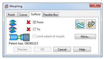
The two surface method provides more control over the shape of the result than the single point methods. It can be used to make substantial changes to a model, for example to stretch or bend in a controlled manner, or to project one shape onto another.
