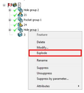
The group is removed and the features are moved into the main tree.
