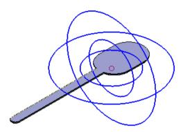
To create the bulge you require you must modify the distortion point, origin point, size and shape of the morph using the methods below.
