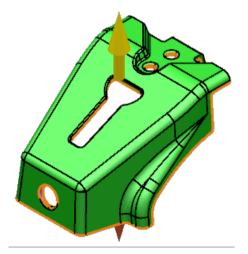
The part is split into the cavity and core sections.
