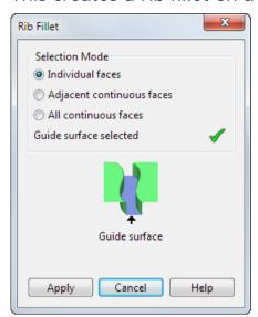
**Selection Mode** - Select a face on the solid as a guide surface. The fillet is created along this surface.
