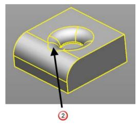
Select Add All Continuous Faces when you need the fillet to spread onto all surfaces that are tangent plane continuous.
