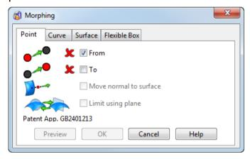
**From** — This allows you to select or modify the origin point that usually lies on the surface of the model. It is shown as a small blue circle.
