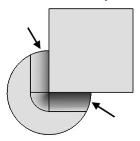
The bottom of the fillet is tangential to the cylindrical part of the solid and the top of the fillet touches the edge of the block at an angle.
