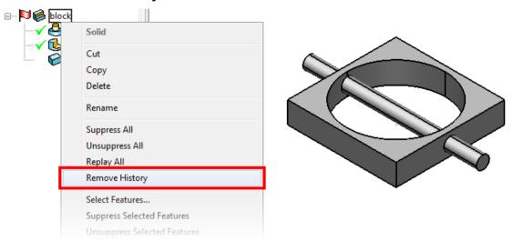
The features are permanently removed from the tree.
