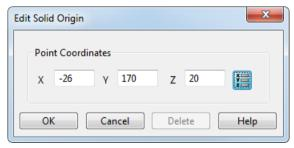
Use this dialog to define a reference point for a solid, to be used as a reference point during in grading.
