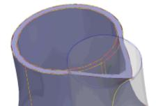
Points are moved depending on the distance from their corresponding point on the **From** curve and the distance from the closest point on the selected limit curve or surface. The closer the point is to the limit curve or surface, the less the point moves. Beyond the selected curve or surface, the points are not moved at all.
