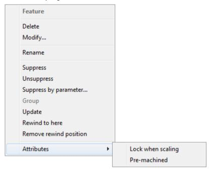
**Lock when scaling** behaves slightly different for each feature.and is not available for some features.
