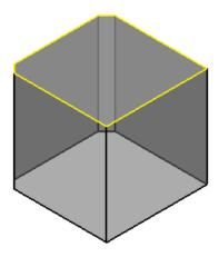
**Chamfer Away From A Face** — With this option selected, selecting a face on the model will cause all the edges that will be chamfered to be highlighted. The highlighted tracks will be chamfered when you click **Apply**.
