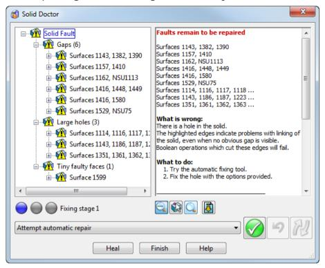
**Fault Tree** - This lists the faults in the solid. Faults can be selected in the Fault Tree or the model window. If you select a fault in the tree, it will be highlighted in the model. You can also select a fault in the model to highlight it in the tree.
