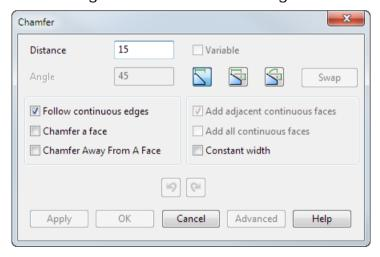
Enter the **Distance** to be used to create the chamfer as shown below.
