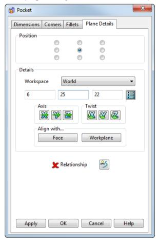
**Position** - The location of the workplane on the feature is defined using this panel.
