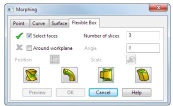
The distortion buttons on the dialog let you edit the model dynamically by manipulating the drag handles on a box. As you move the drag handles, you distort the box. You can select different slices within the bounding box and morph the section using a combination of twist, bend, stretch and shear until you achieve the desired result.
