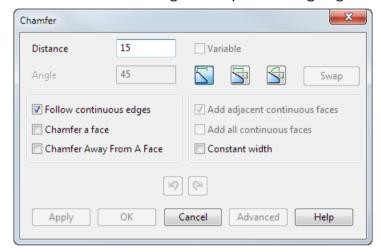
If one of the options Follow Continuous Edges, Chamfer a Face or Chamfer Away From A Face are selected and you hover over a valid edge, a path may highlight. Otherwise, only the single edge highlights. Full details on these options are given below.
