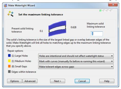
**Present solid linking tolerance** - This is the latest tolerance to which the solid has been linked.
