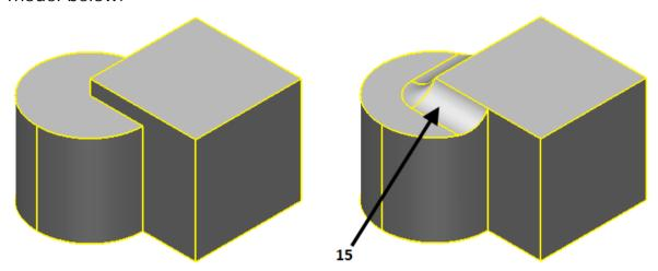
A fillet of 15 has been added at the intersection of the block and the cylinder. The important things to note about this fillet are:
