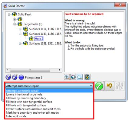
Apply 2 - Click to apply the repair option to the selected faults.
