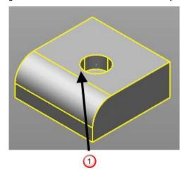
To spread the fillet beyond onto all surfaces, use the **Add All Continuous Faces** option. This option will allow you to create the fillet onto the continuous surfaces ②.
