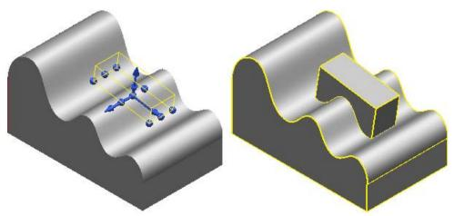
If *OFF*, the protrusion is not extended onto the main solid and the same model would look like this:
