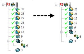
**Merge** — Use this option to merge adjacent transform features of the same type. For example, if you move a solid three times, selecting **Merge** will merge the three transform features into one.
