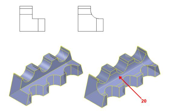
Looking at the wireframe view below, you can see that the fillet is carried right up the side walls of the block.
