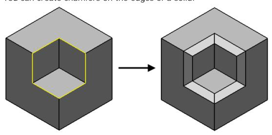
To create a solid chamfer:
