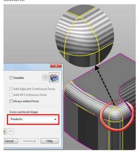
Curvature continuous - This option creates a fillet without the sharp change in curvature that is created using the Circular option. Sections of the fillet are not circular; the curvature varies continuously as the blend is created between the adjoining faces.
