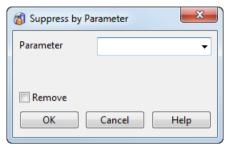
**Parameter** — Use the drop-down list to select the parameter to control suppression of the feature. The parameter can also be used to control multiple, selected features.
