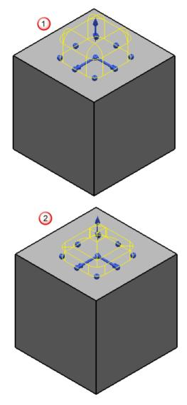
**Radius** - Enter the radius of the fillet around the base of the pocket or the top of the protrusion.
