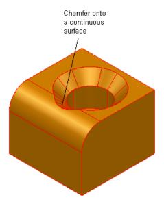
**Add all continuous faces** — This is the same as the **Add adjacent continuous faces**, except the chamfer can spread onto all surfaces that are tangent plane continuous.
