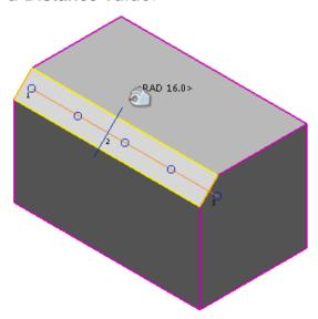
To delete the selected line, press **Delete.** End lines cannot be deleted.
