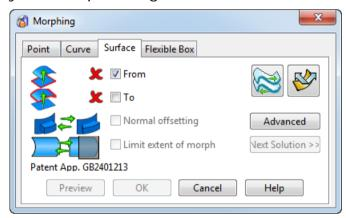
**Normal Offetting** - If *ON*, the surfaces to be morphed are bent to follow the **To** surface. Full details on how selected objects are morphed when **Normal Offsetting** are provided in the Solid Modelling manual.
