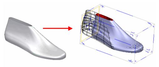
You can swap between the different drag handles at any time and make as many different edits to the box as you like before applying the morph.
