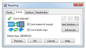
**Curve both ways** - This option affects the extent the morph is limited. If *ON*, the model is curved in two directions relative to the curve 4. If *OFF*, the distortion will be kept constant along an axis controlled by the current principal plane 5. If no workplanes exist in the model, the **World** workplane is used.
