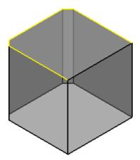
**Chamfer a face** — If this option is selected and you hover over a valid edge, before a path is selected, a path is highlighted containing all edges of a face of the solid which contains that edge.
