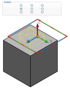
**Details** - The workplane for the feature is defined using these options. The usual workplane instrumentation is displayed whilst this page of the form is selected.
