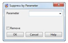
**Parameter** lets you select the parameter to control suppression of the feature. The parameter can also be used to control multiple selected features.
