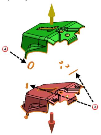
4 Click to select **Undercut shading**; this will indicate faces that have insufficient draft when viewed from above or below the tool.
