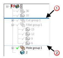
The rewind position appears as a horizontal bar on the solid tree 0.
