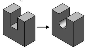
The new fillet is tangent to the walls and its base touches where the face used to lie.
