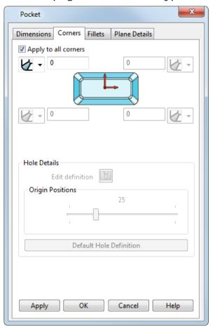
**Apply to all corners** - If *ON*, the corner details you have specified are applied to all corners. If *OFF*, each corner is defined separately.
