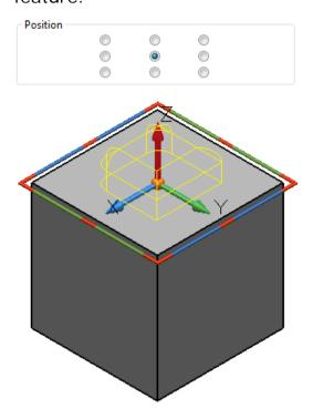
Selecting an alternative setting will define the workplane accordingly. The example below defines the workplane at the middle of the left edge of the pocket/protrusion.
