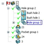
If you delete a group feature, the hole features are moved up a level in the tree and the group feature icon is removed from the tree.
