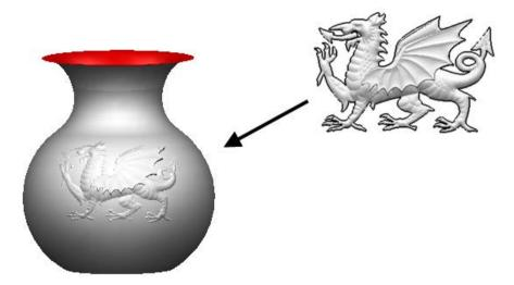
The wrapping method is the same as **Wrap Triangles** from the **Surfaces** toolbar, except the wrap is created as a solid feature displayed in the feature tree. This enables the wrap feature to be edited.
