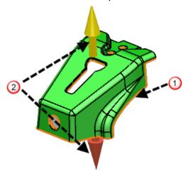
3 Use the **Solid Core/Cavity Separation** wizard (see page 303) to split a solid into core, cavity, sliders and internal features (such as holes).
