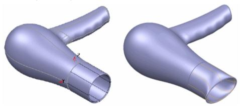
All the features on the objects such as fillets, trimming, walls, ribs and bosses remain intact, even though the shape may be totally changed.
