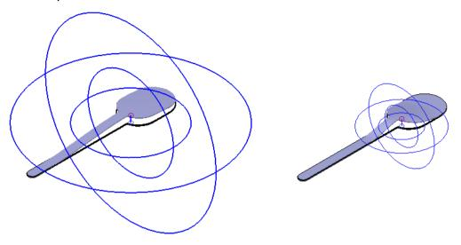
Altering the inner sphere affects the shape of the morph. Decreasing the size of the inner sphere means that the morph is sharper. Increasing the size of the inner sphere produces a more rounded bulge.
