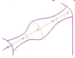
Horizontal — the radius remains constant for a short distance away from the arc and then takes on the conditions dictated by the neighbouring arc.
