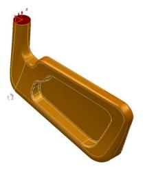
This view is a **shaded view** with the **surfaces wireframe curves displayed**.
