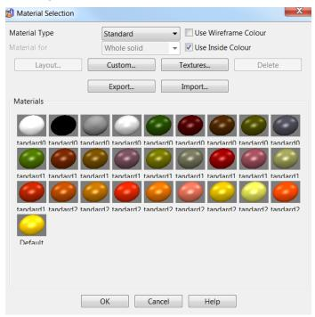
By default, all surfaces are shaded using the same material. However, individual surfaces can be modified to use a shading colour and material type from the standard range or as customised by the user. There is a comprehensive range of pre-set Material type options available, such as metallic, glass, and neon.
