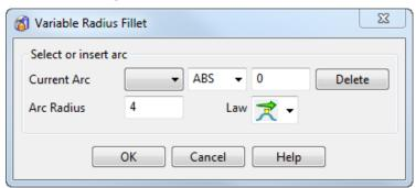
This **dialog** allows you to use the **mouse** to **select** an **arc** that represents the **radius of the fillet** at a location around the **curve** representing the shape. This works in a similar way to **variable radius filleting** of **surfaces** covered later. When you move the mouse along the track, the word **Key** appears. Click at these **points** to easily generate a **numbered arc**. The size of this **arc** can then be **stretched** or **modified** in the dialog.
