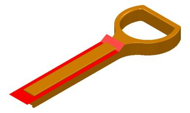
**38** Make the **inner-core solid active**, and **select** the new **extrusion surface**.
