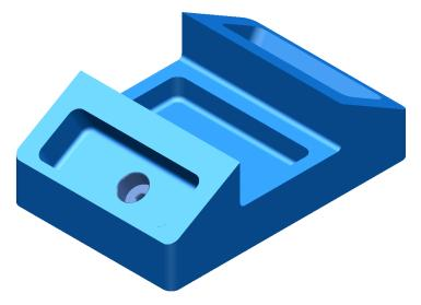
3 Create a workplane at the **centre of the pocket** aligned to the top sloped face as shown.
