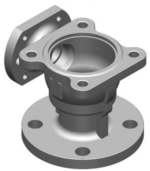
The surfaces have been shaded to show the full extent of the surface area. The wireframe from which it is constructed can also be shown if required. The model can be rotated dynamically so that the user can view the underside detail.
