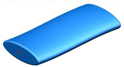
The model now is complete but before a split surface can be generated the appropriate **Draft Curve** must first be created.
