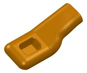
The **imported model** of a **plastic molding** is **not** in a **suitable orientation** from which to create a **mold tool**. A **suitably positioned workplane** will be **created** to provide an **appropriate tooling datum**.
