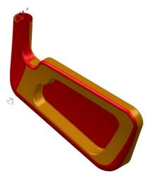
This view **enables/disables** the mode which displays **inside-out surfaces** as **red**. This allows the user to **shade** the **model without** having to **reverse inside-out surfaces**. Ensure the option is **ticked** to view **negative facing surfaces**.
