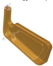
This view shows the **model partially shaded** (**transparent**), which provides a compromise with **visual access** to the inner and **wireframe detail**.
