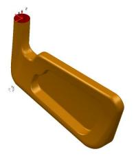
The model is displayed with the **surface skin shaded**. The **outside** of a **surface** is the **default** or **user-defined colour**; the **inside** is **shaded red**. The use of shading **restricts visual access** to **internal detail**.
