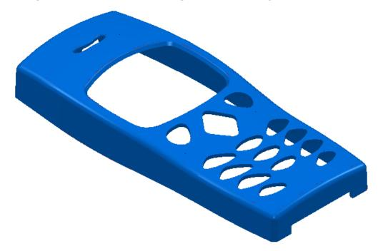
The **Phone\_Model.dgk** contains the **surface data** of a mobile phone cover. For **PowerSHAPE** to process the data through the **Die Wizard**, the model needs to be in the form of a **solid**. After conversion from a **Surface** model to a **solid** it is strongly advised to **check** for any potential **faults**.
