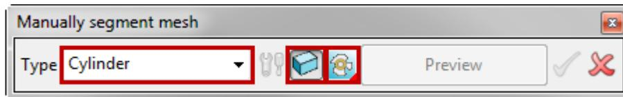
We are now going to **fit primitives** in order to create the **PCD** of **holes** on the **part**. To do this we need to **fit** a **number** of **primitive cylinders** to **calculate** the **diameter** of the **pattern** using a **3 point arc**, which will also give us the **centre point** of the **pattern**.
