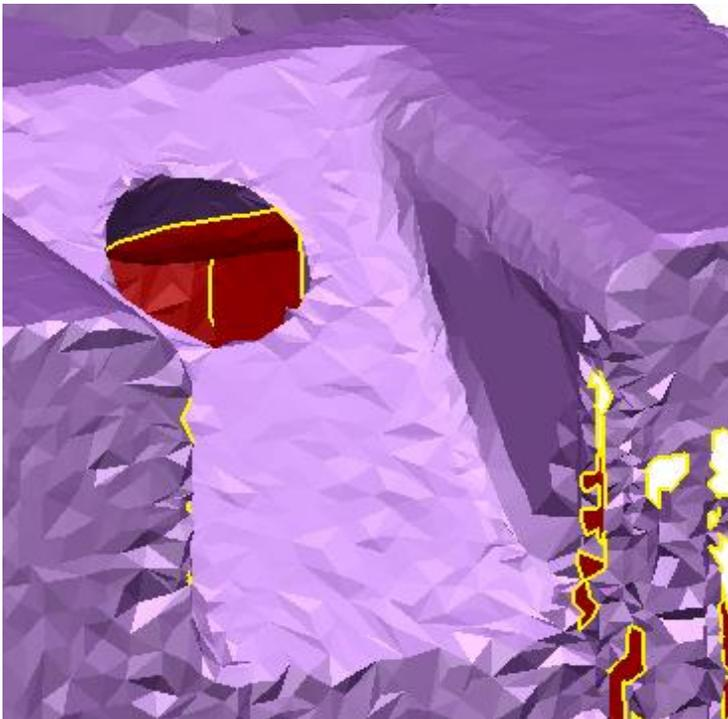
**Importantly**, taking a look at the **right hand side vertical wall** of the cut (**above**), we can see that due to some **missing data** and the **hole** being '**filled**' when the **mesh** was created, the wall is not quite vertical. We can solve this issue by **Moving** a **copy** of the **surface** we generate from the **opposite wall**.
