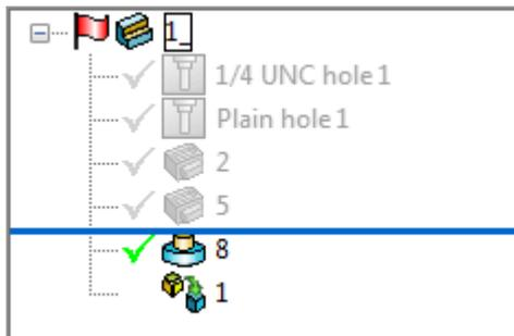
To remove the **Rewind Position** simply right-click in the solid tree on any feature and select the option to **Remove Rewind Position**.
