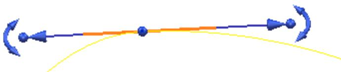
These handles allow the user to graphically edit the **Tangency** and **Magnitude** of the curve point.
