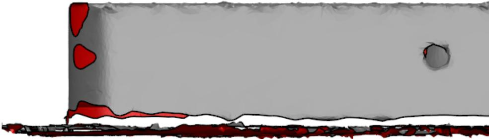
Removing any **unwanted data** in the **mesh** will **reduce** the **overall mesh size** and **complexity** and **speed** up the **software graphics**. We will do this using **limit selection** from a **new workplane**, and as we already have **isolated a small section** to provide the **overall part depth** and placed it on a **separate level**, we can **remove** the rest of the **extra data**.
