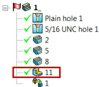
The **Solid cut** feature is added to the bottom of the solid feature tree below the three solid pockets created earlier.
