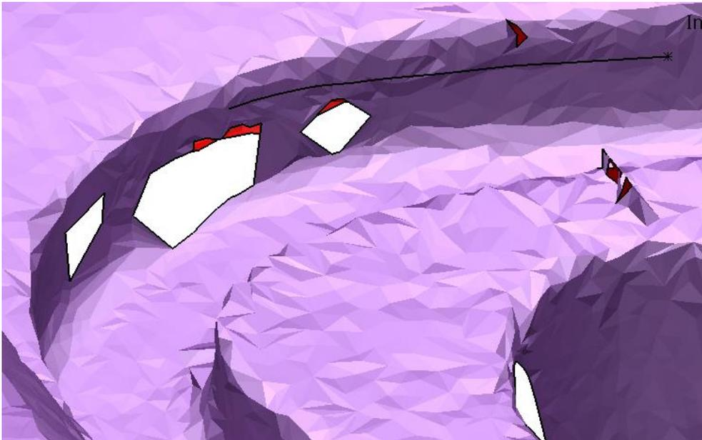
**300** When almost complete, the **curve** can be **closed** and **created** to **double clicking** on the **first point**.
