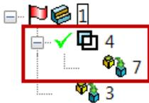
Looking to the **left** at the **Solid History Tree** we can see that this feature has been created by effectively creating a **solid** from the **wrapped curve** and the using a **Boolean Remove** function to create the cut.
