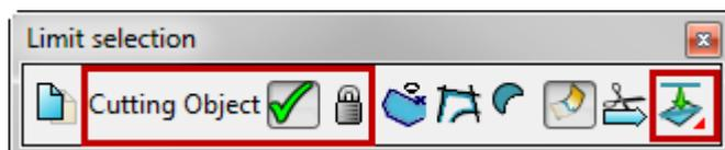
**233** In the **graphics area**, **select** and **limit** the **ALL section curves** to this **line**. The **workplane projection mode** will **limit** using a **plane** created by the **line** and the **principal axis**.
