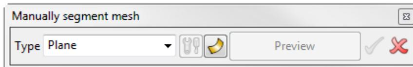
This will also open the **Set Triangle Area to Local Horizon** menu to allow to select **individual (multiple) triangles** in the **mesh**. This dialog allows you to manually seek primitive object on the mesh using the drop down menu provided.
